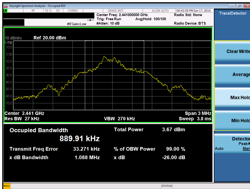
Plot 7-1. Occupied Bandwidth Plot (ANT+ – Ch. 39)
