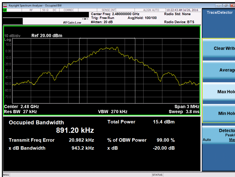
Plot 7-3. 20dB Bandwidth Plot (Bluetooth, 1Mbps – Ch. 78)
