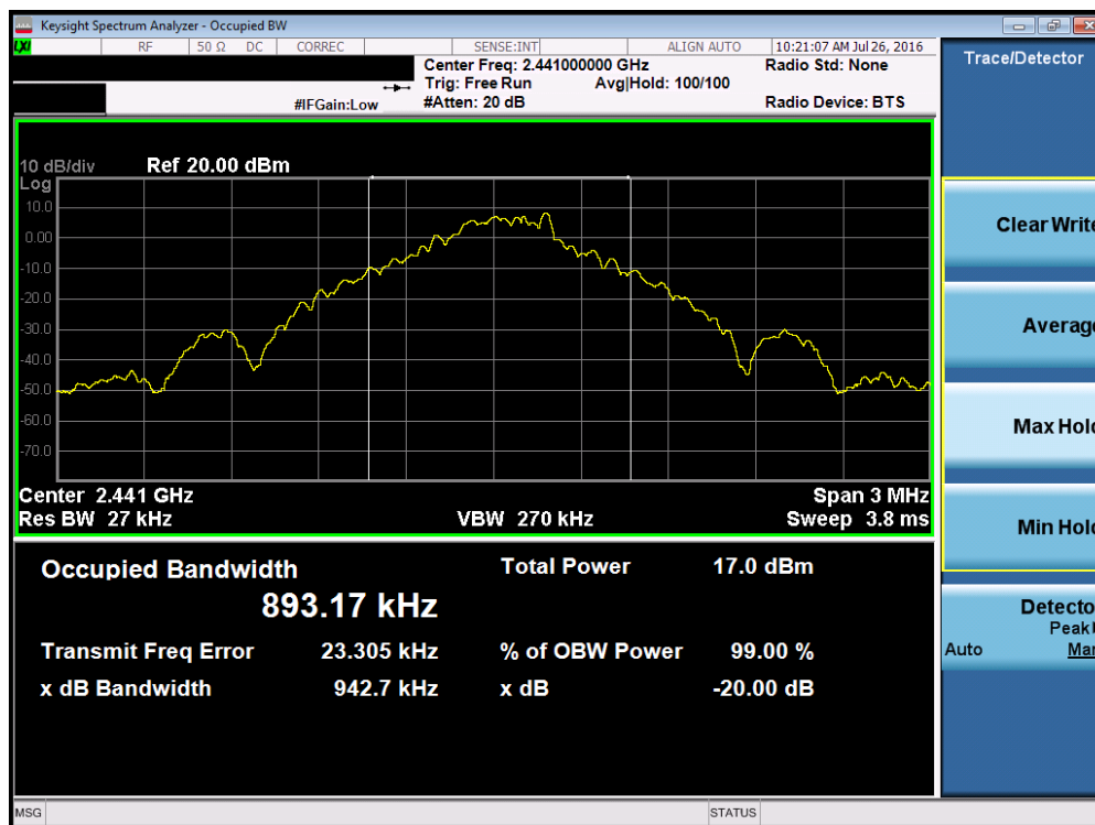
Plot 7-2. 20dB Bandwidth Plot (Bluetooth, 1Mbps – Ch. 39)
