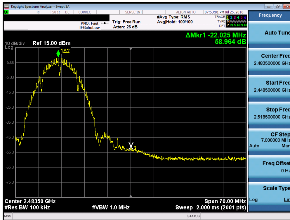
Plot 7-20. Band Edge Plot (802.11b – Ch. 11)
