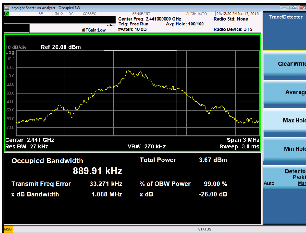
Plot 7-1. Occupied Bandwidth Plot (ANT+ – Ch. 39)
