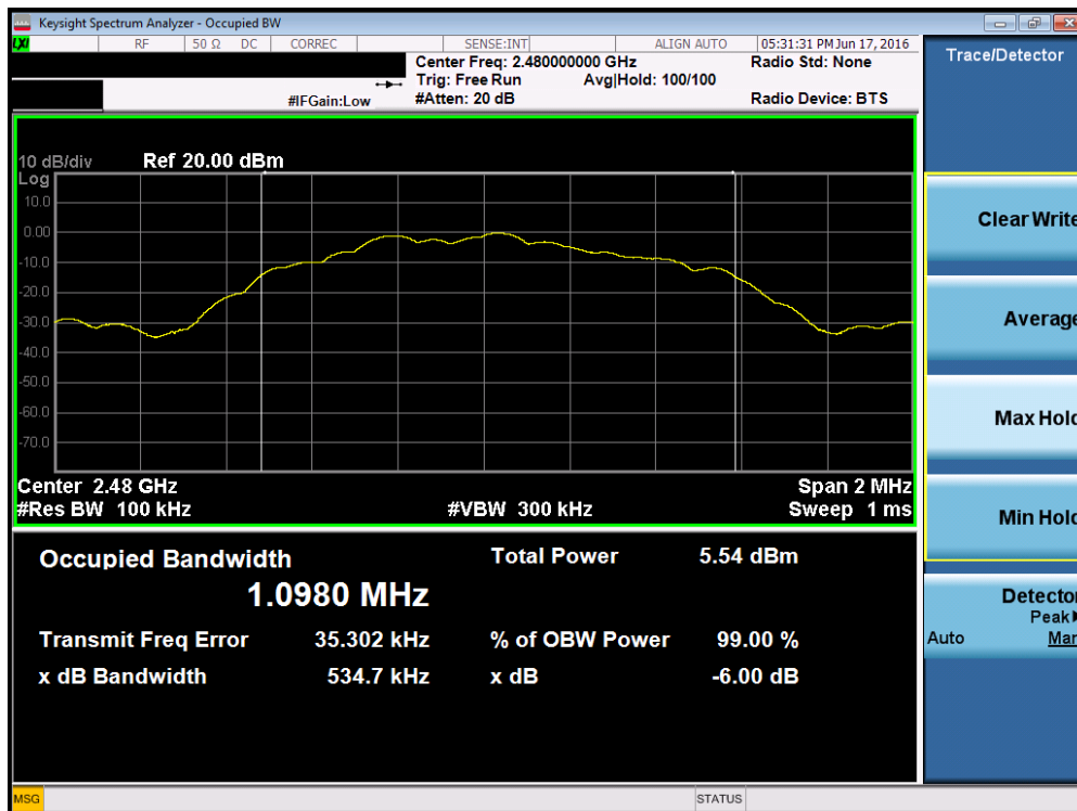
Plot 7-3. 6dB Bandwidth Plot (Bluetooth (LE) – Ch. 39)
