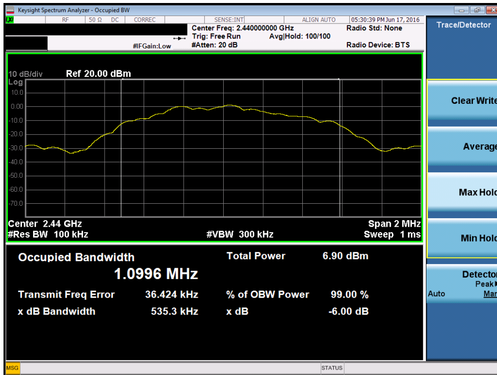
Plot 7-2. 6dB Bandwidth Plot (Bluetooth (LE) – Ch. 19)
