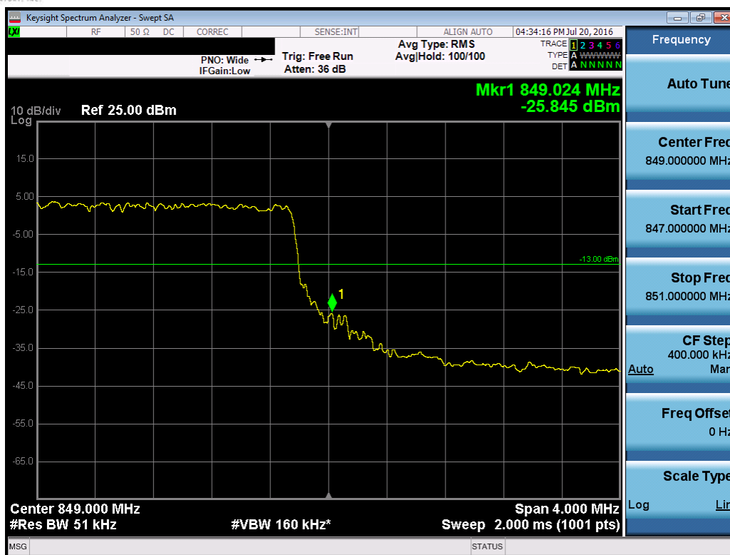
Plot 7-28. Upper Band Edge Plot (Band 5 – 5.0MHz QPSK – RB Size 25)
