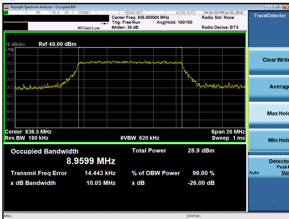
Plot 7-7. Occupied Bandwidth Plot (Band 5 – 10.0MHz QPSK – RB Size 50)
