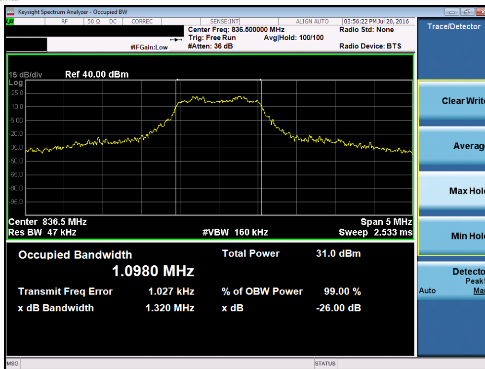
Plot 7-1. Occupied Bandwidth Plot (Band 5 – 1.4MHz QPSK – RB Size 6)
