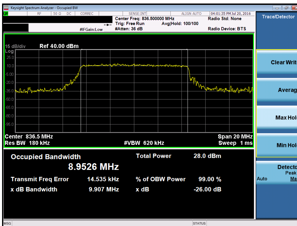
Plot 7-8. Occupied Bandwidth Plot (Band 5 – 10.0MHz 16-QAM – RB Size 50)
