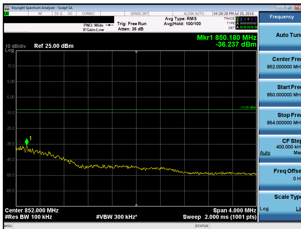
Plot 7-21. Upper Extended Band Edge Plot (Band 5 – 1.4MHz QPSK – RB Size 6)
