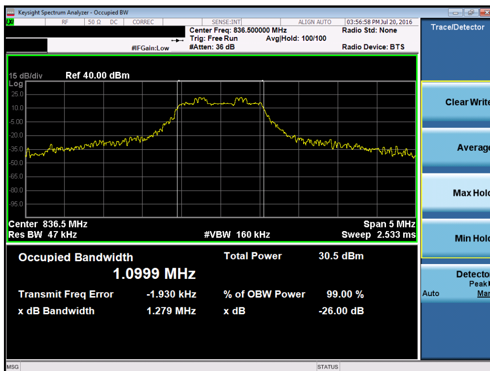
Plot 7-2. Occupied Bandwidth Plot (Band 5 – 1.4MHz 16-QAM – RB Size 6)
