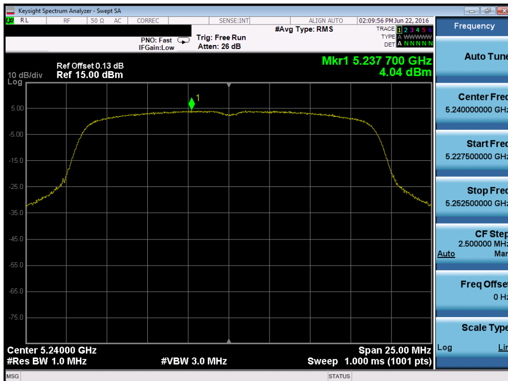
Plot 7-45. Power Spectral Density Plot (20MHz BW 802.11n (UNII Band 1) – Ch. 48)
