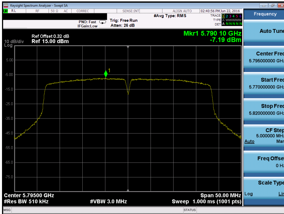
Plot 7-77. Power Spectral Density Plot (40MHz BW 802.11n (UNII Band 3) – Ch. 159)
