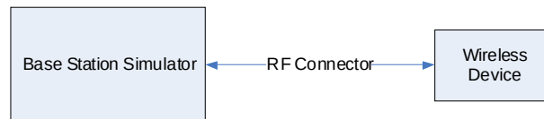
Figure 8-1 Power Measurement Setup
