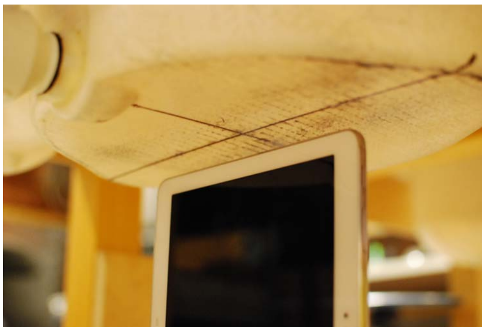
SAR Test Setup Photo 6 – Left Edge at 1.5 cm
