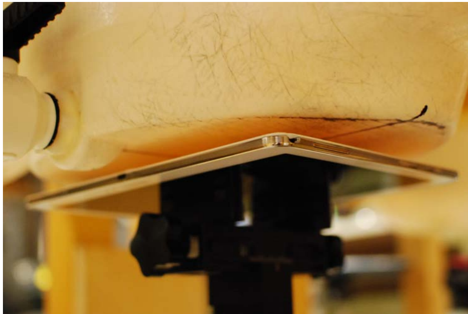
SAR Test Setup Photo 2 – Back Side at 1.2 cm
