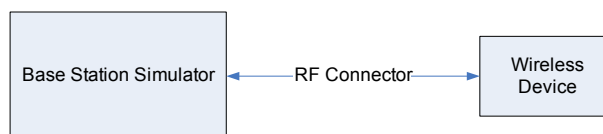
Figure 8-2 Power Measurement Setup
