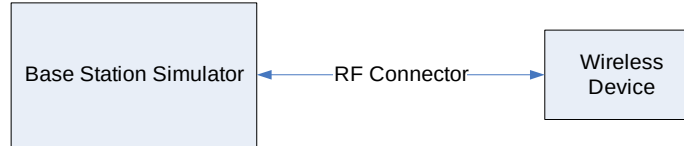
Figure 8-2 Power Measurement Setup
