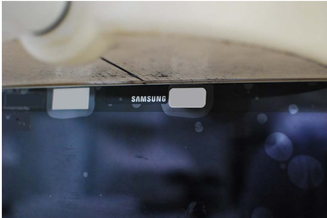
SAR Test Setup Photo 3: Top at 0.0 mm
