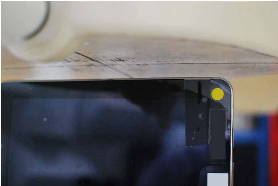
SAR Test Setup Photo 5: Left at 12 mm
