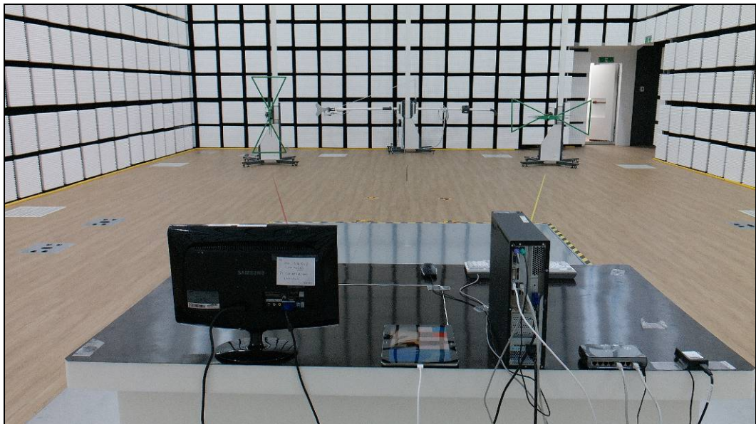
[ Radiated Disturbance for Below 1 GHz – Rear ]
