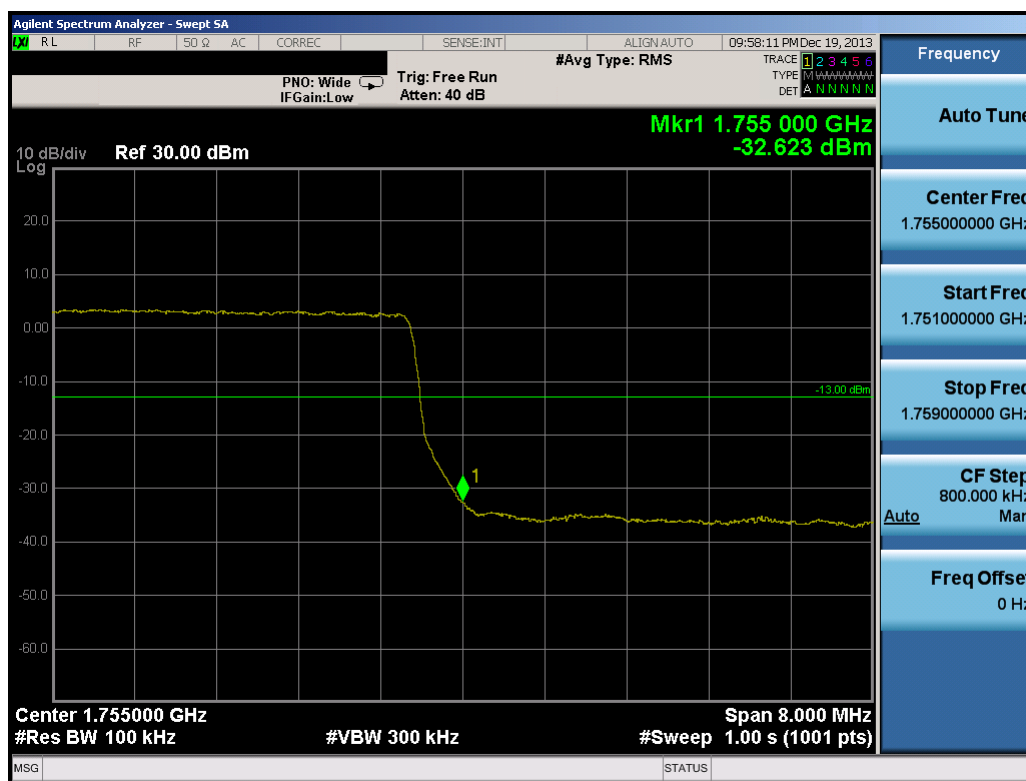
Plot 9-53. Upper Band Edge Plot (10.0MHz QPSK – RB Size 50)
