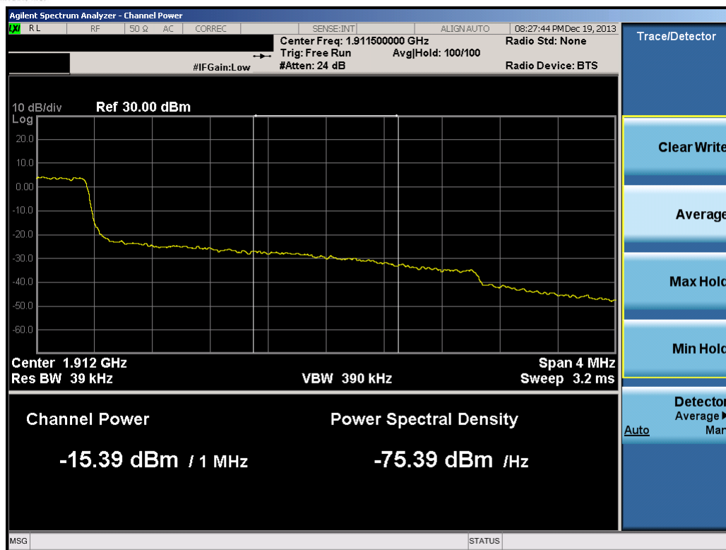
Plot 10-26. Upper Extended Band Edge Plot (3.0MHz QPSK – RB Size 15)
