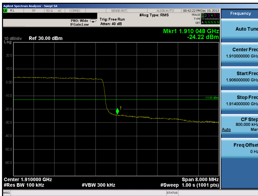
Plot 10-53. Upper Band Edge Plot (10.0MHz QPSK – RB Size 50)
