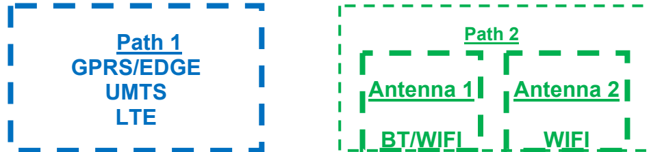
Figure 1-2 Simultaneous Transmission Paths
