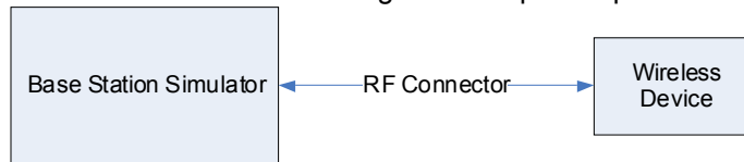
Figure 8-1 Power Measurement Setup
