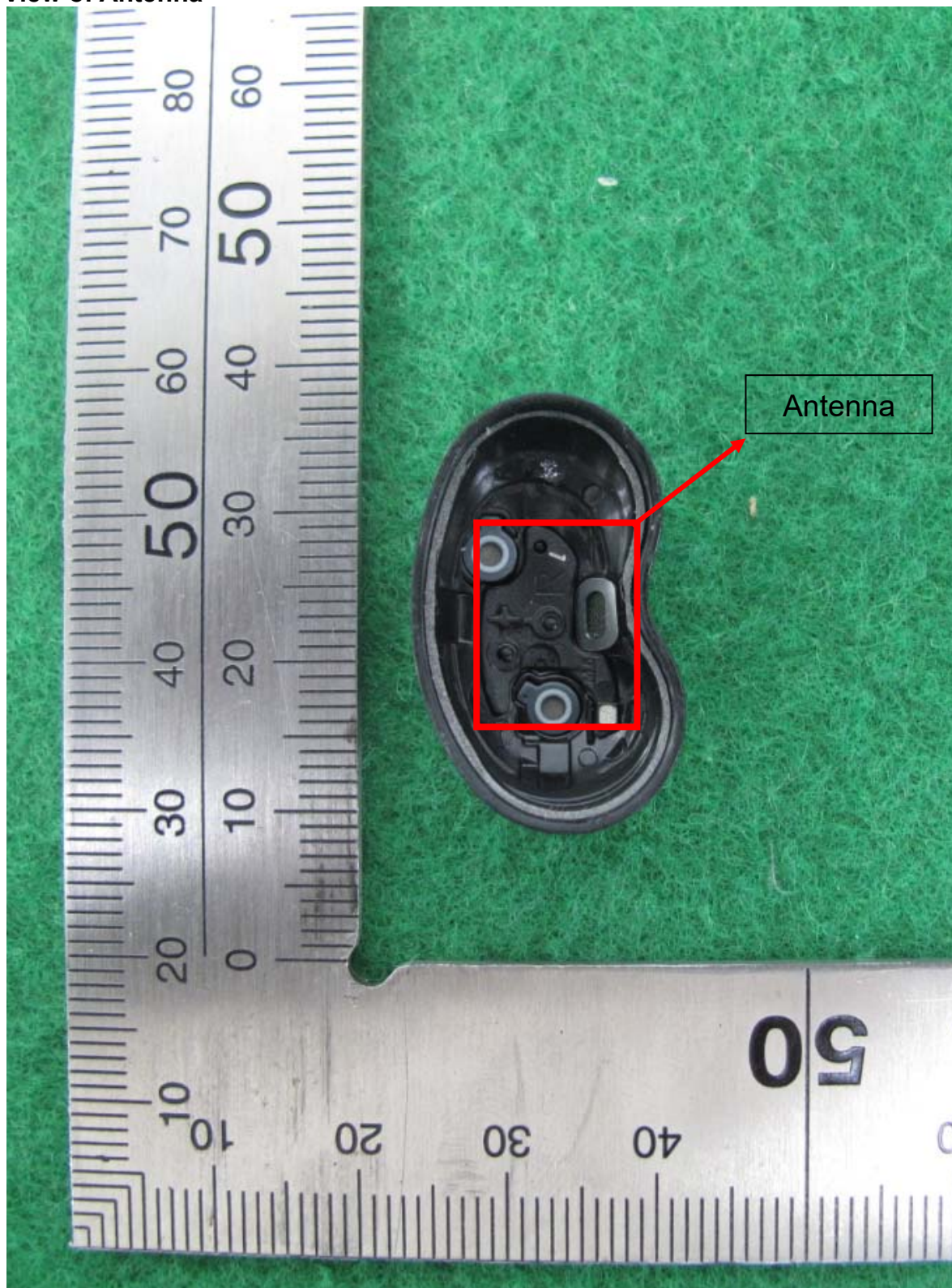
View of Antenna
