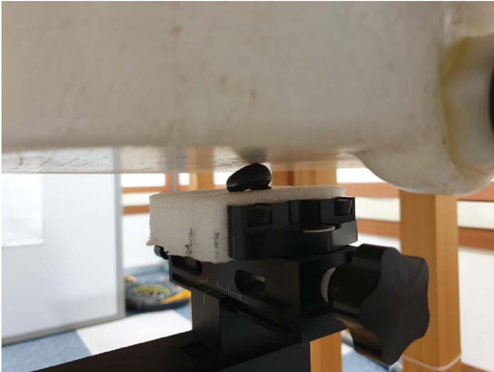
SAR Test Picture(Back), Test separation distance : 0 mm
