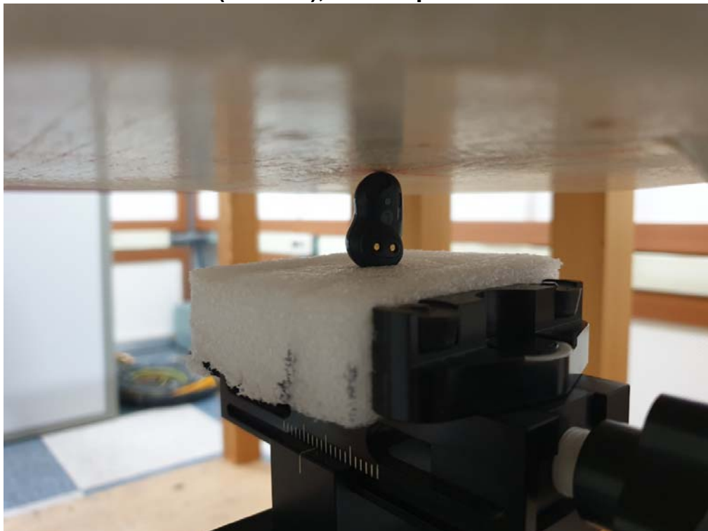
SAR Test Picture(Bottom), Test separation distance : 0 mm
