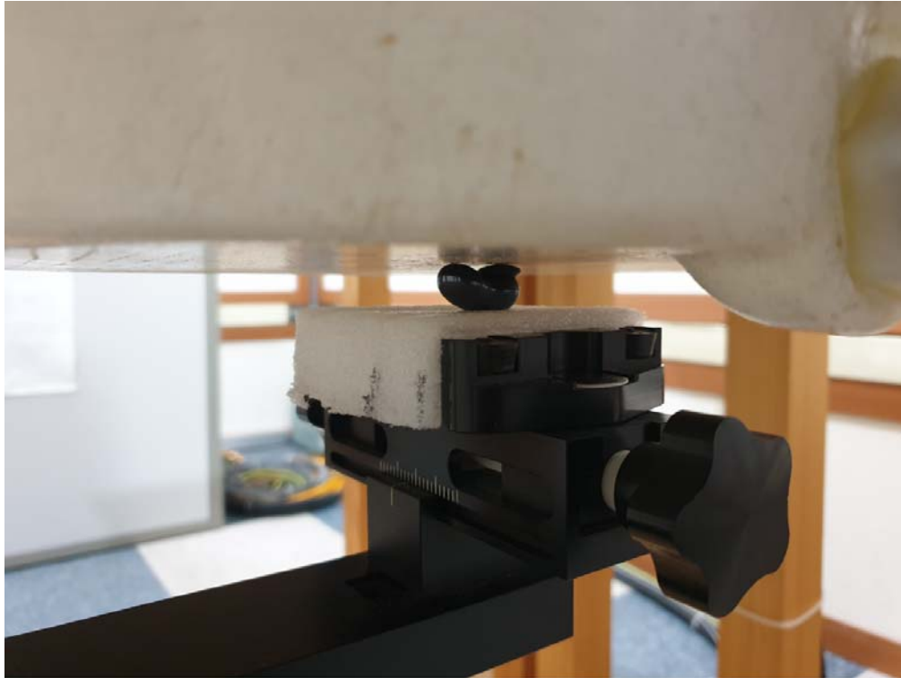
SAR Test Picture(Front), Test separation distance : 0 mm
