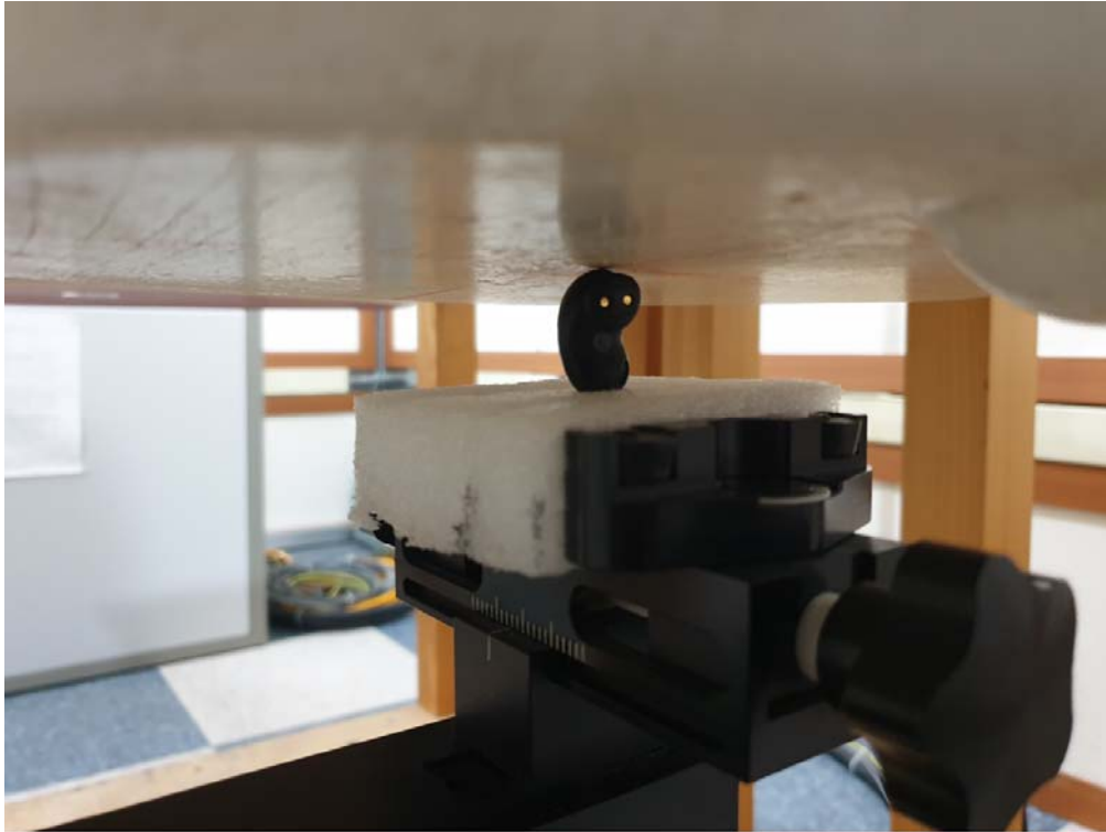
SAR Test Picture(Top), Test separation distance : 0 mm
