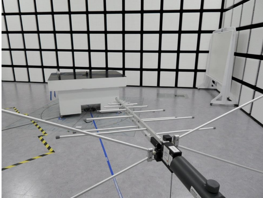
RADIATED FRONT PHOTO (BELOW 1 GHz)
