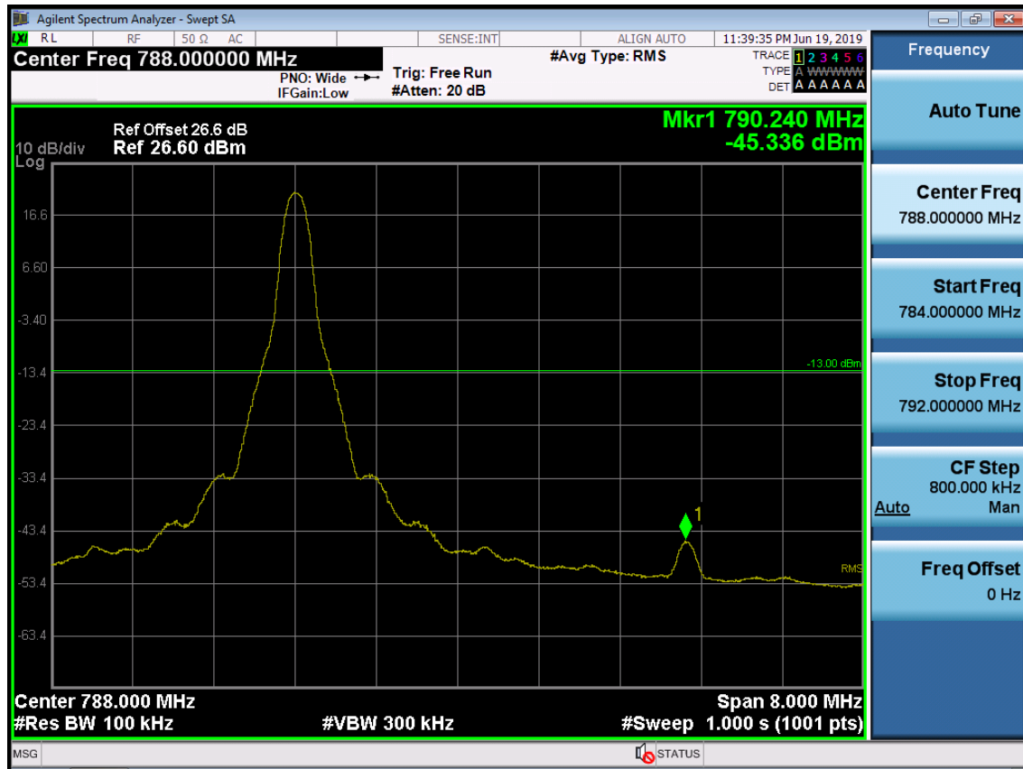
Band 13 Upper Band Edge Plot (10M BW Ch.23230 QPSK_RB1_Offset_49)
