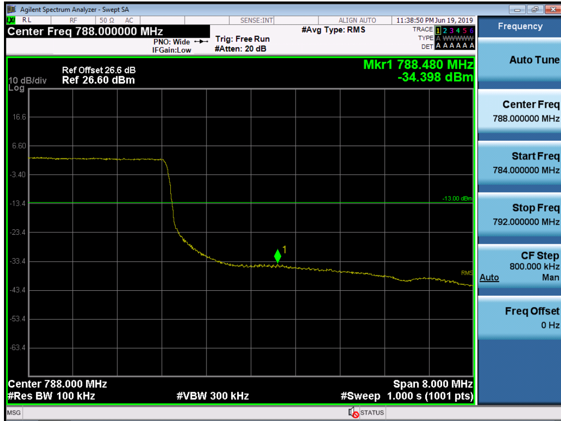
Band 13 Upper Band Edge Plot (10M BW Ch.23230 QPSK_ QPSK_RB_50)
