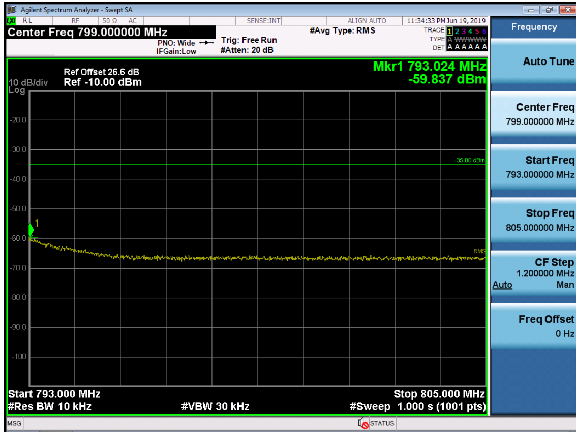
Band 13 Upper Emission Mask (793 MHz ~805 MHz) Plot (5M BW Ch.23255 QPSK_RB25_0)
