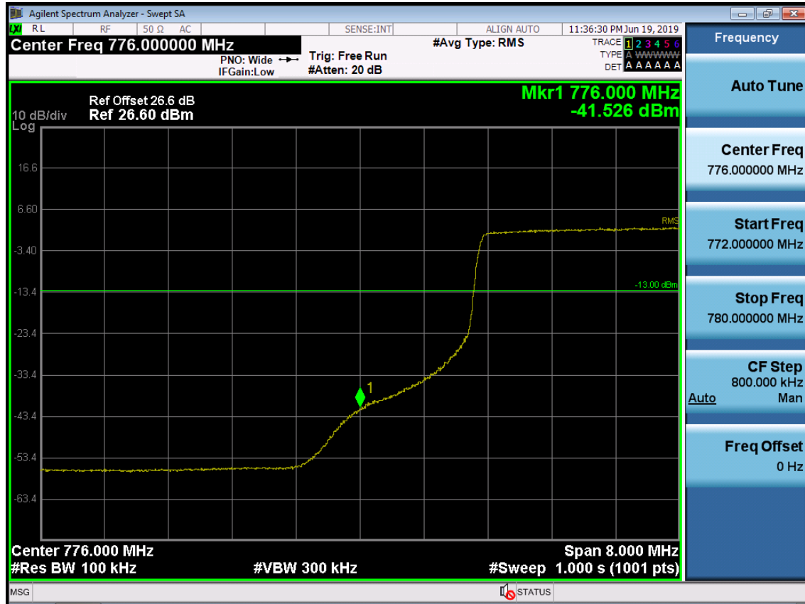
BAND 13. Lower &amp; Upper Band Edge Plot (10M BW Ch.23230 QPSK RB_50)
