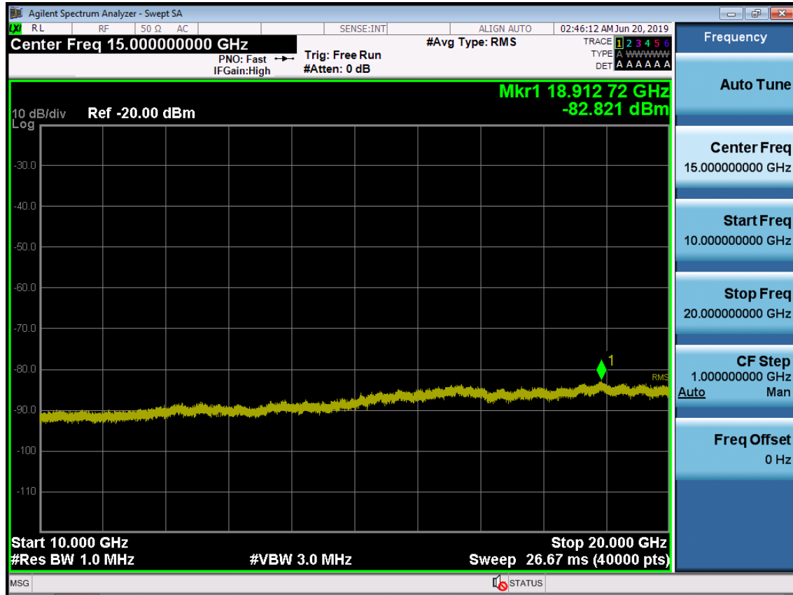
BAND 66. Conducted Spurious Plot_2 (132322ch_15MHz_QPSK_ RB 1_0)
