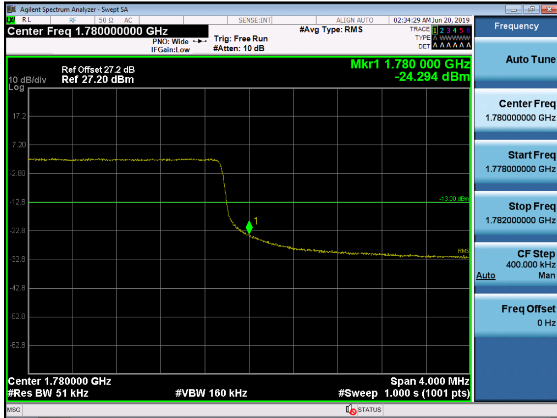
BAND 66. Upper Band Edge Plot (5M BW Ch.132647 QPSK_RB25) -2
