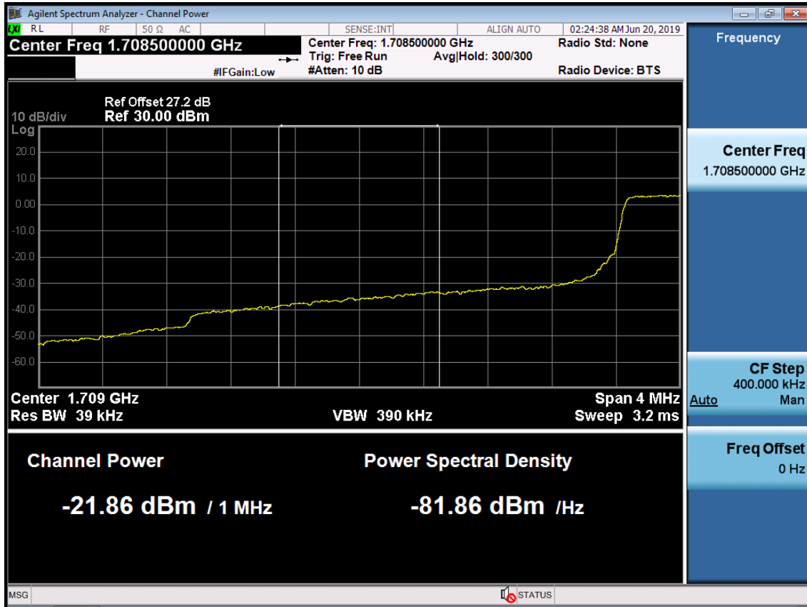
BAND 66. Lower Extended Band Edge Plot (3M BW Ch.131987 QPSK_RB15_0) -3
