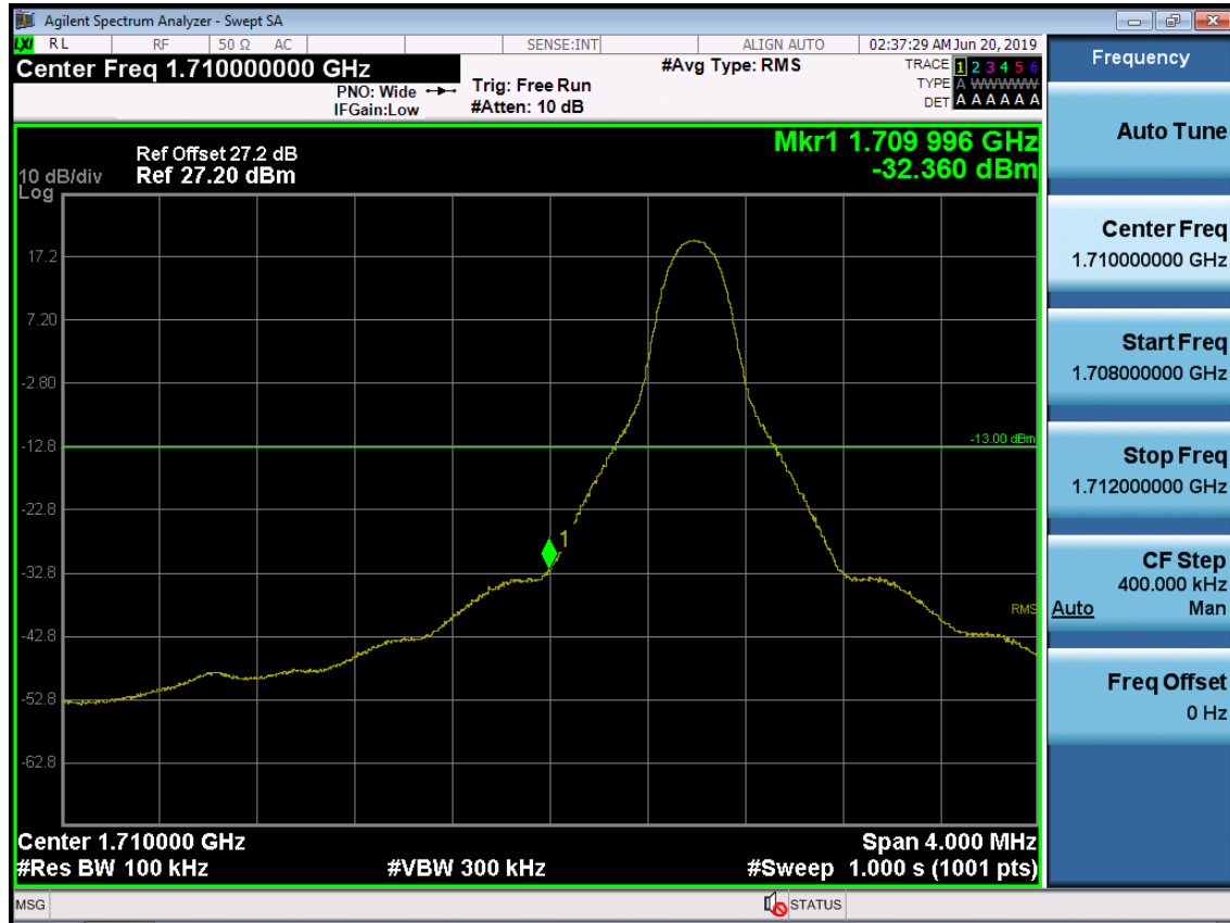
BAND 66. Lower Band Edge Plot (10M BW Ch.132022 QPSK RB 1, Offset 0) -1
