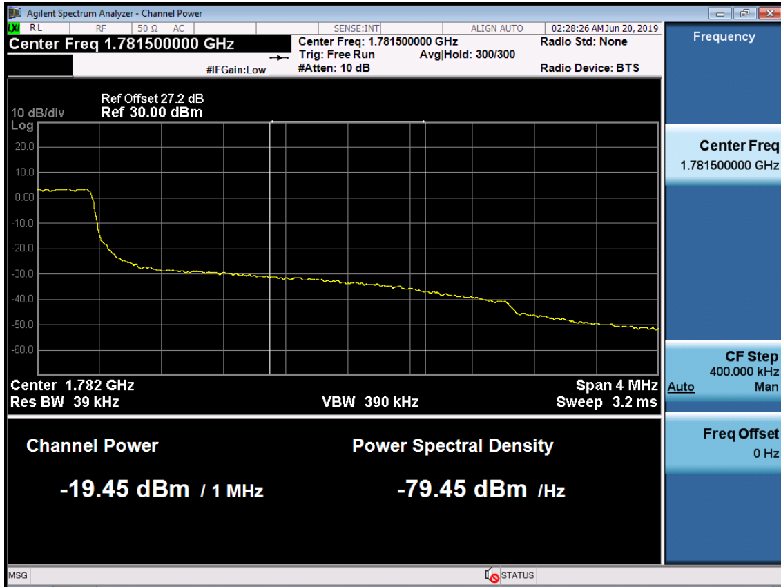
BAND 66. Upper Extended Band Edge Plot (3M BW Ch.132657 QPSK_RB15_0) -3
