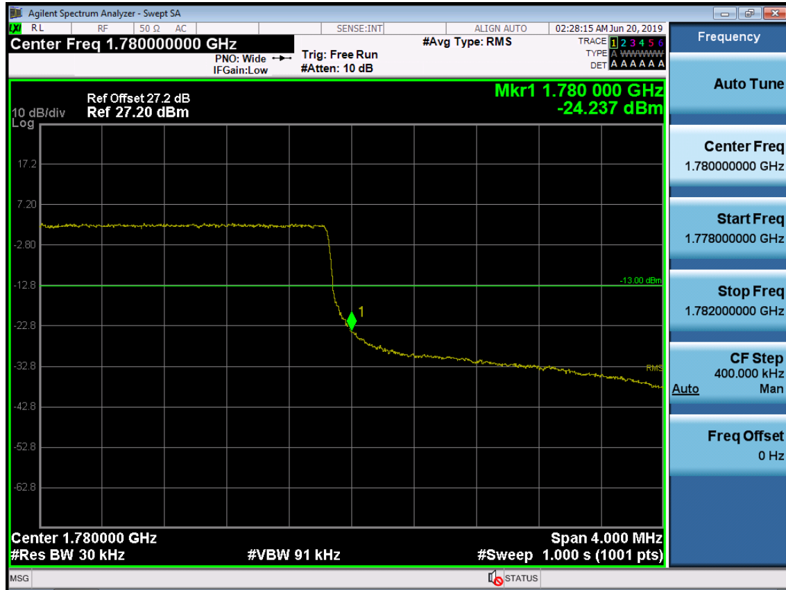
BAND 66. Upper Band Edge Plot (3M BW Ch.132657 QPSK_RB15) -2
