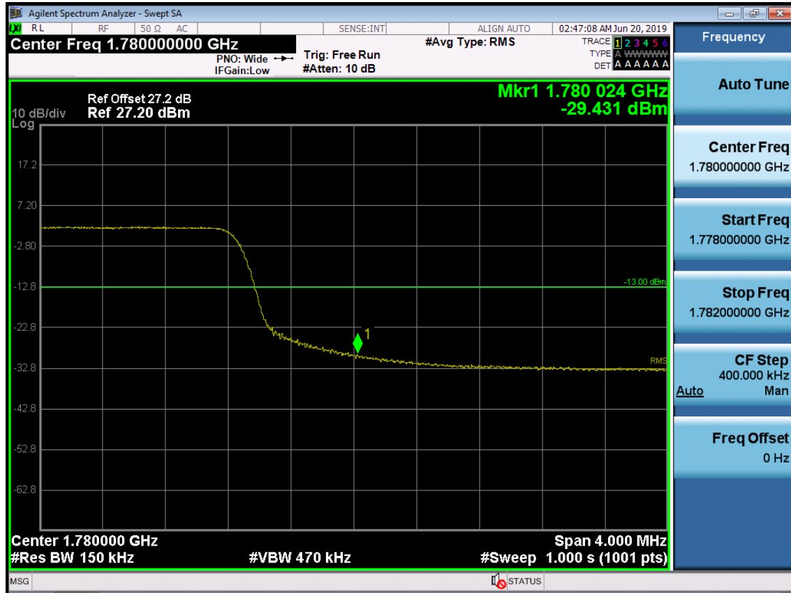
BAND 66. Upper Band Edge Plot (15M BW Ch.132597 QPSK_RB75) -2
