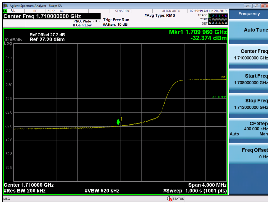
BAND 66. Lower Band Edge Plot (20M BW Ch.132072 QPSK RB 100) -2
