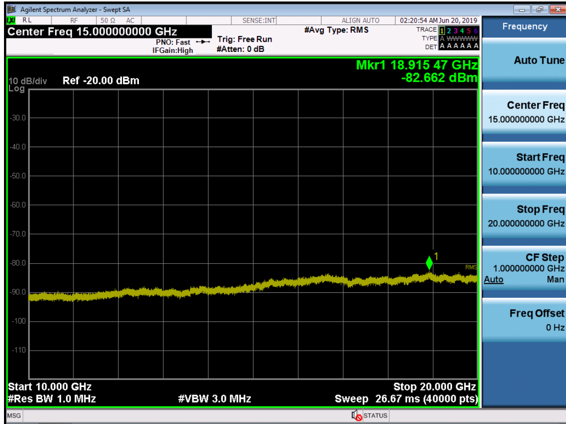
BAND 66. Conducted Spurious Plot_2 (132322ch_1.4MHz_QPSK_ RB 1_0)
