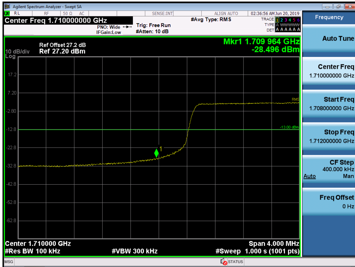
BAND 66. Lower Band Edge Plot (10M BW Ch.132022 QPSK RB 50) -2
