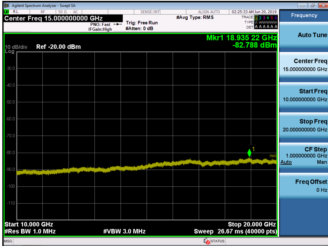
BAND 66. Conducted Spurious Plot_2 (131987ch_3MHz_QPSK_RB 1_0)
