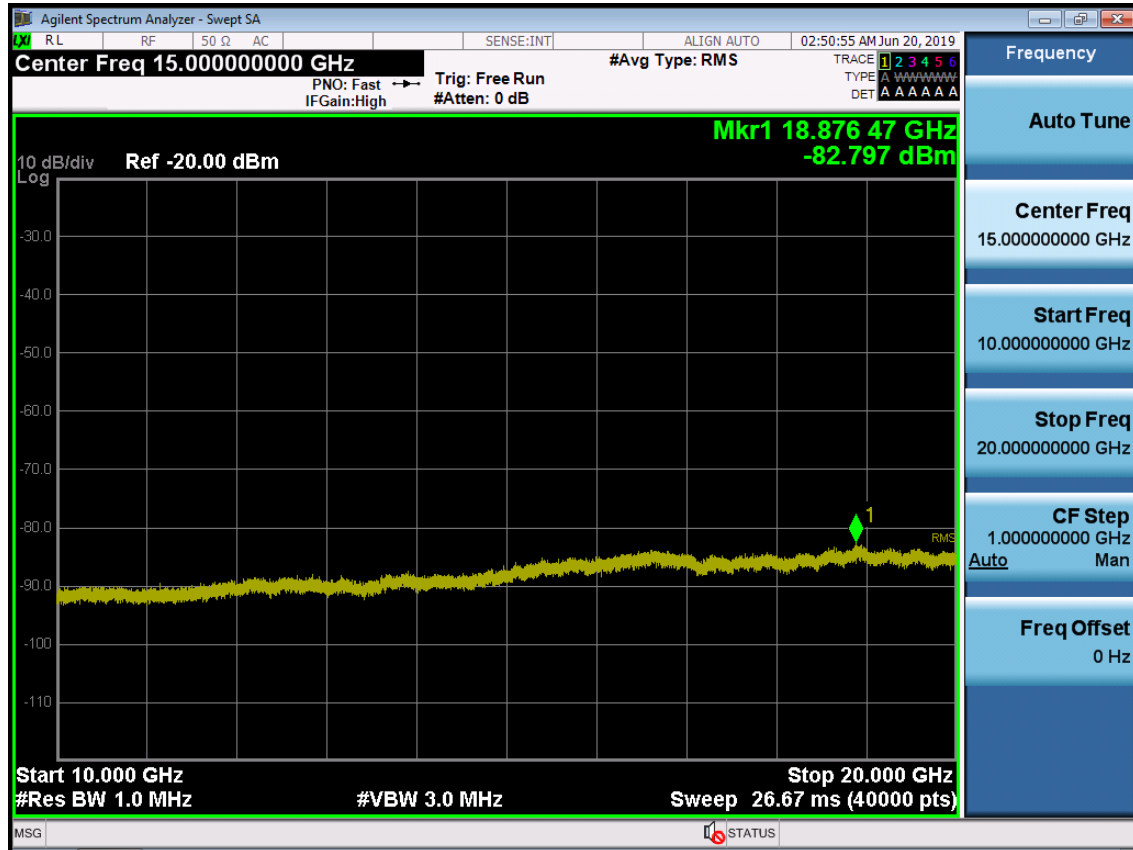
BAND 66. Conducted Spurious Plot_2 (132072ch_20MHz_QPSK_ RB 1_0)
