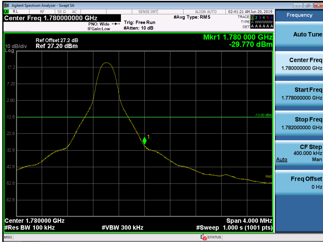
BAND 66. Upper Band Edge Plot (10M BW Ch.132622 QPSK_RB1_Offset 49) -1
