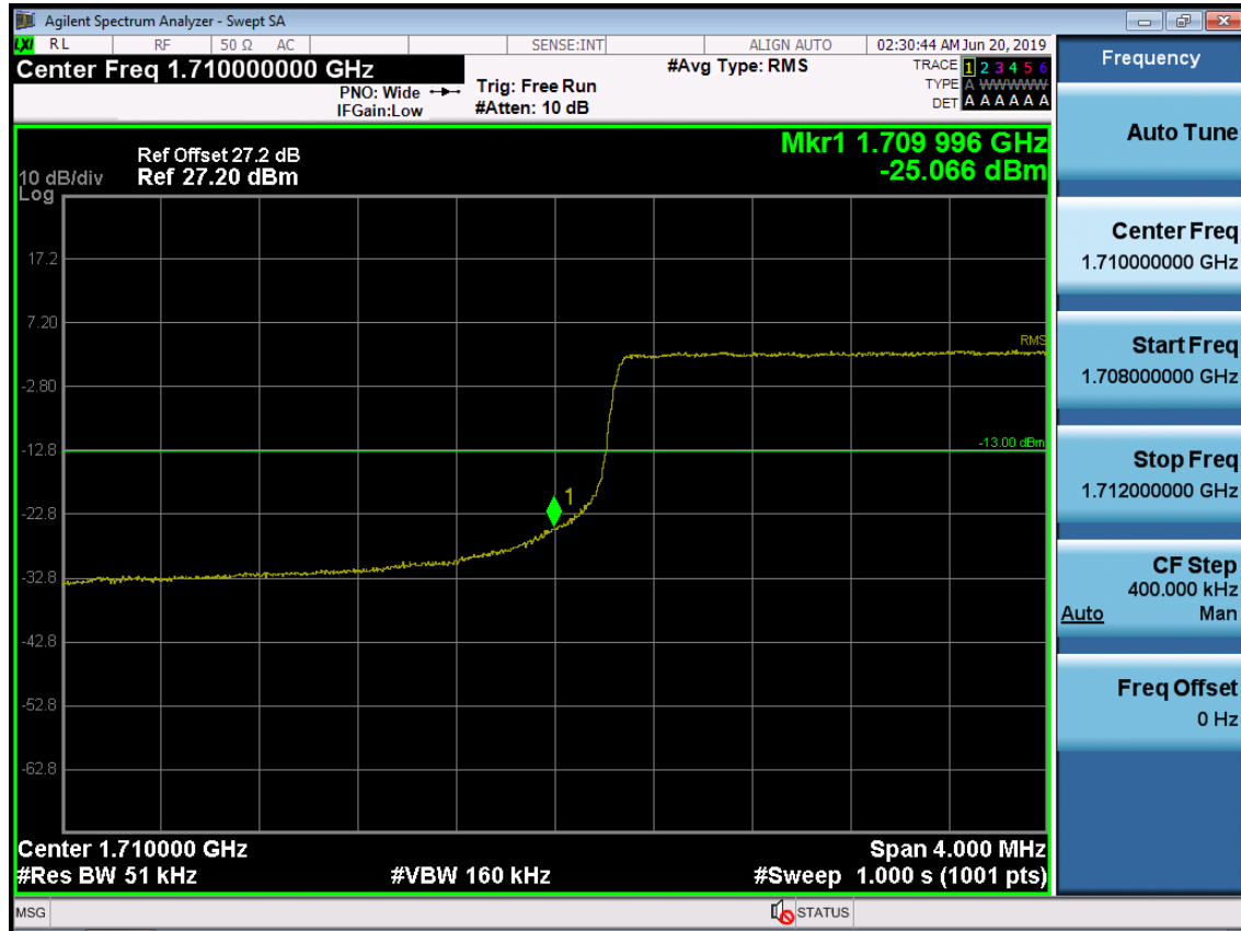
BAND 66. Lower Band Edge Plot (5M BW Ch.131997 QPSK RB 25) -2
