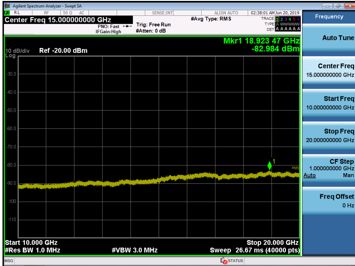
BAND 66. Conducted Spurious Plot_2 (132022ch_10MHz_QPSK_ RB 1_0)
