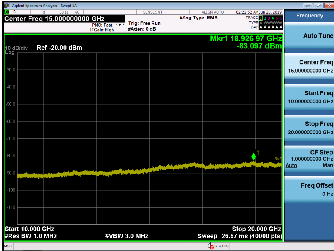
BAND 66. Conducted Spurious Plot_2 (132665ch_1.4MHz_QPSK_ RB 1_0)
