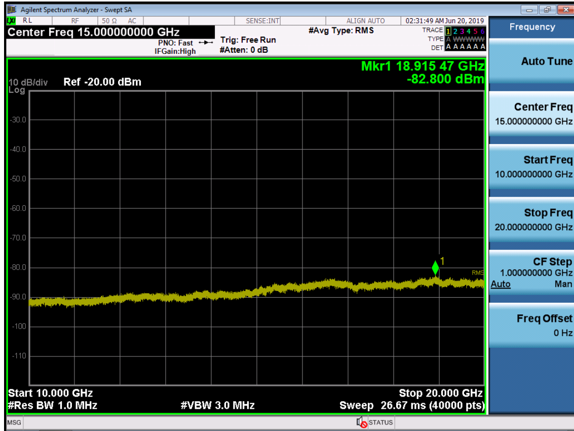
BAND 66. Conducted Spurious Plot_2 (131997ch_5MHz_QPSK_RB 1_0)
