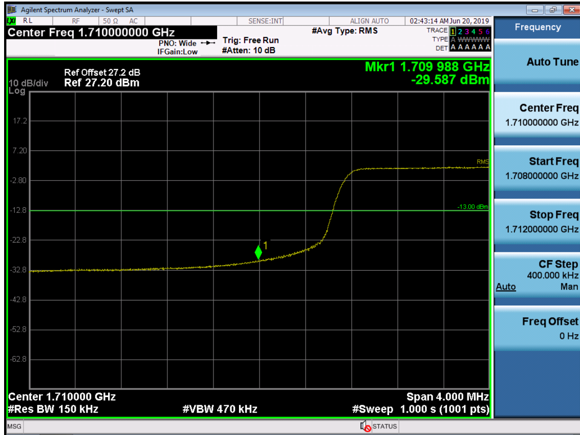
BAND 66. Lower Band Edge Plot (15M BW Ch.132047 QPSK RB 75) -2
