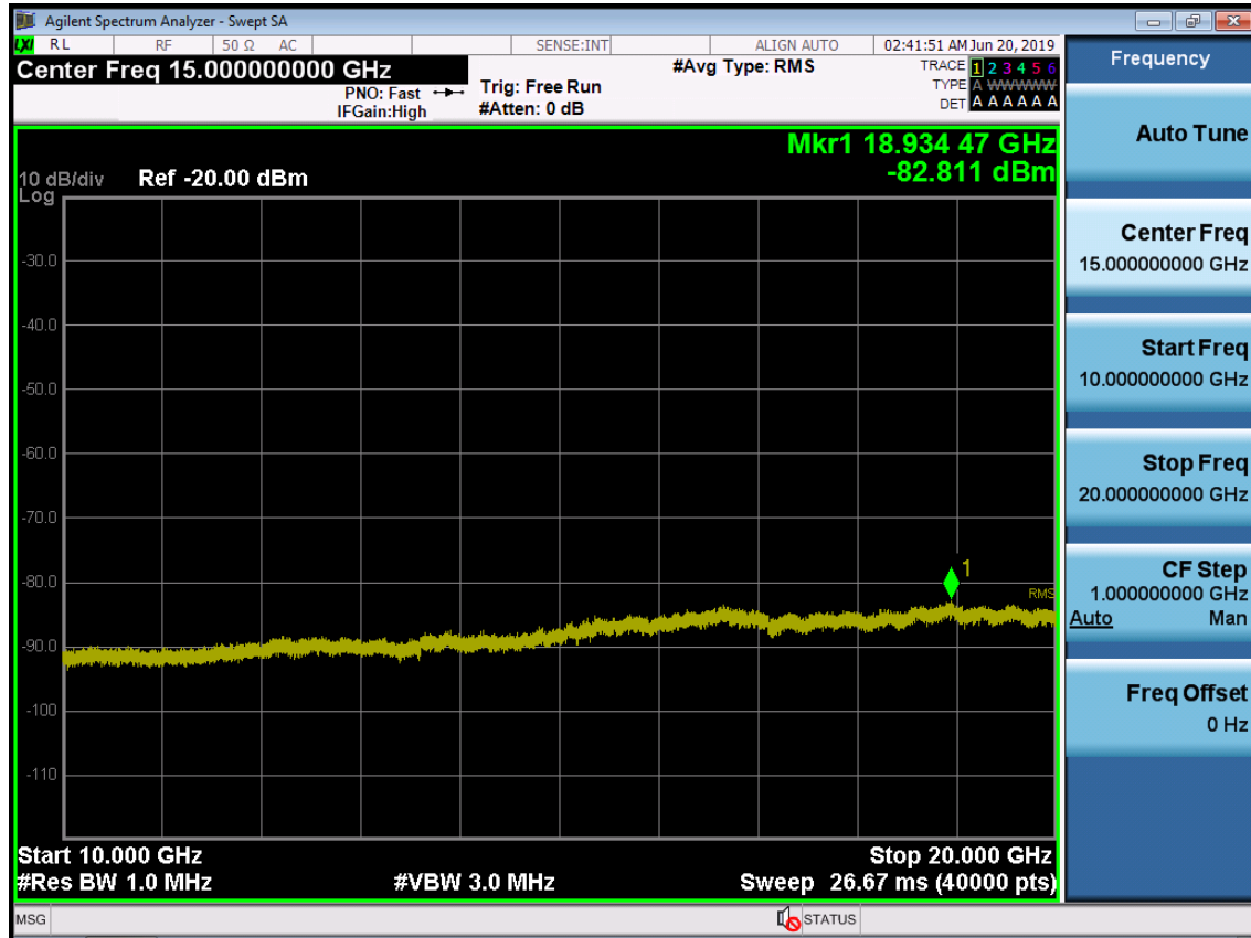
BAND 66. Conducted Spurious Plot_2 (132622ch_10MHz_QPSK_ RB 1_0)
