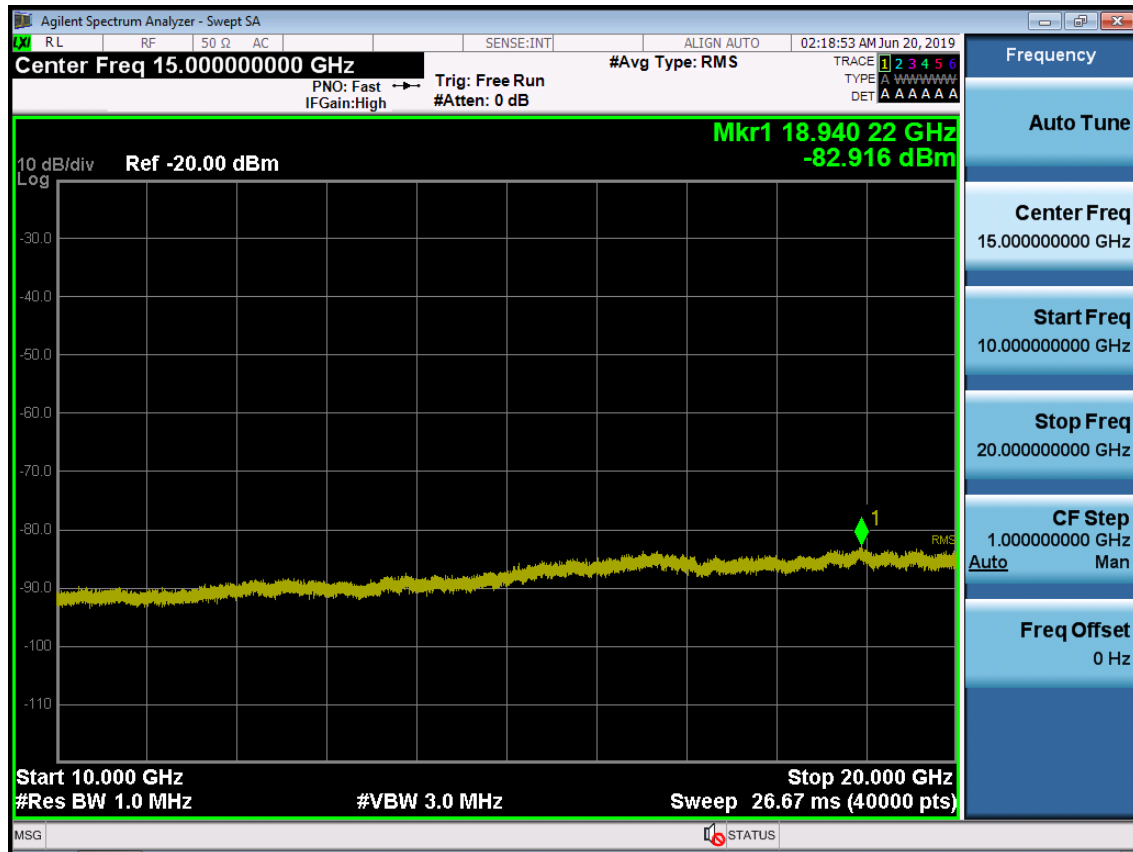
BAND 66. Conducted Spurious Plot_2 (131979ch_1.4MHz_QPSK_ RB 1_0)
