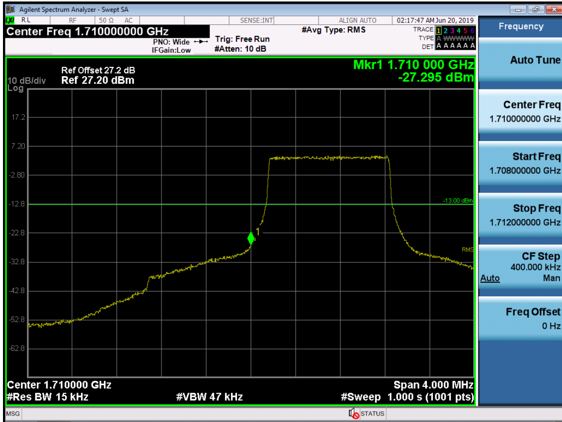
BAND 66. Lower Band Edge Plot (1.4M BW Ch.131979 QPSK RB 6) -2
