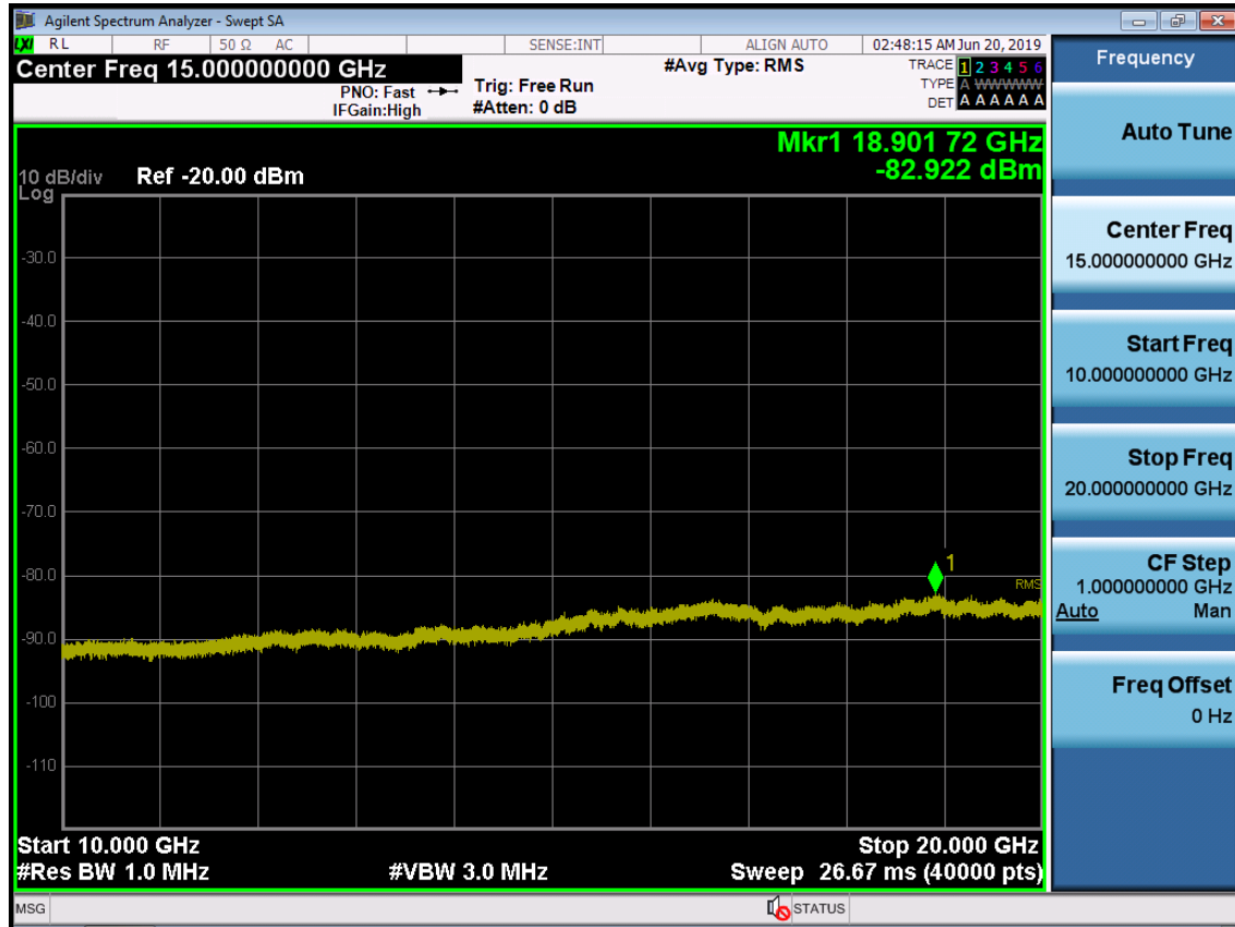
BAND 66. Conducted Spurious Plot_2 (132597ch_15MHz_QPSK_ RB 1_0)
