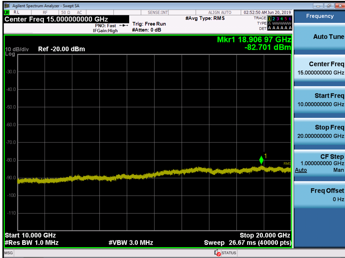
BAND 66. Conducted Spurious Plot_2 (132322ch_20MHz_QPSK_ RB 1_0)
