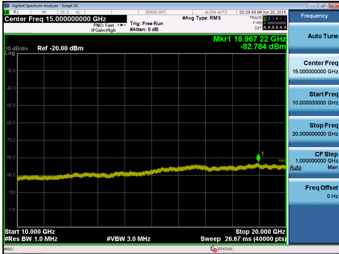
BAND 66. Conducted Spurious Plot_2 (132322ch_10MHz_QPSK_ RB 1_0)
