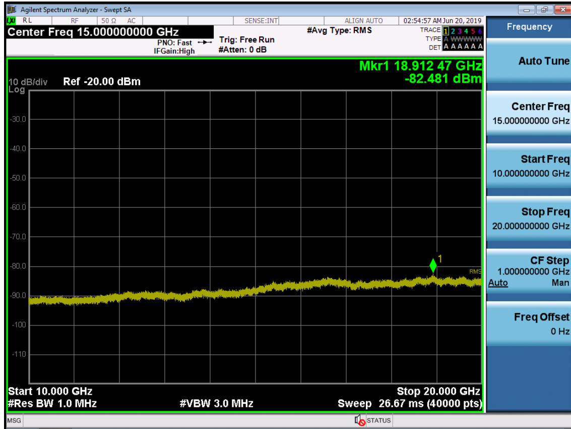
BAND 66. Conducted Spurious Plot_2 (132572ch_20MHz_QPSK_ RB 1_0)
