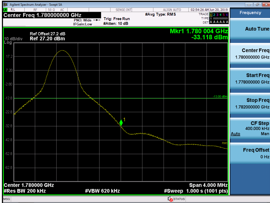
BAND 66. Upper Band Edge Plot (20M BW Ch.132572 QPSK_RB1_Offset 99) -1
