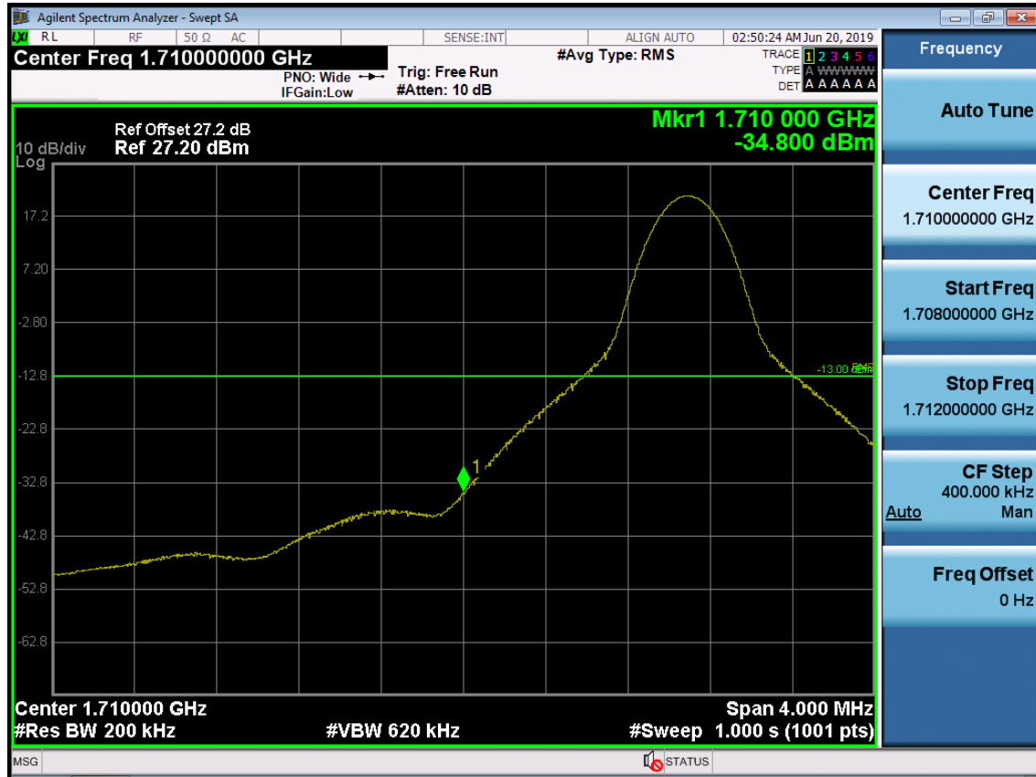
BAND 66. Lower Band Edge Plot (20M BW Ch.132072 QPSK RB 1, Offset 0) -1
