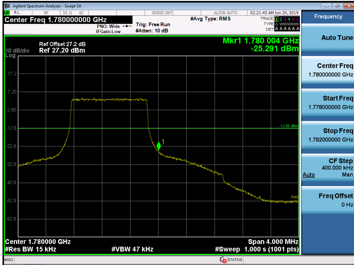
BAND 66. Upper Band Edge Plot (1.4M BW Ch.132665 QPSK_RB6) -2
