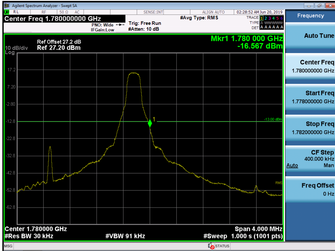
BAND 66. Upper Band Edge Plot (3M BW Ch.132657 QPSK_RB1_Offset 14) -1
