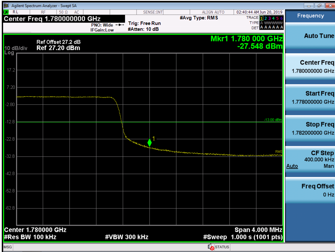
BAND 66. Upper Band Edge Plot (10M BW Ch.132622 QPSK_RB50) -2
