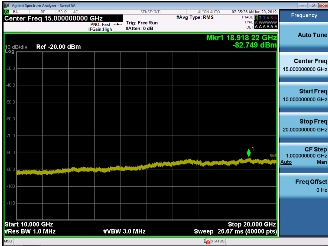
BAND 66. Conducted Spurious Plot_2 (132647ch_5MHz_QPSK_RB 1_0)
