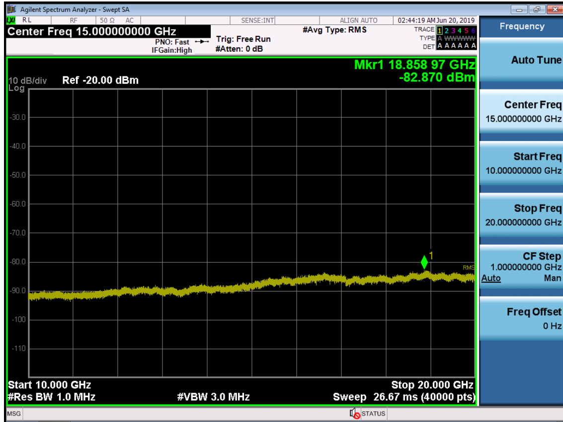
BAND 66. Conducted Spurious Plot_2 (132047ch_15MHz_QPSK_ RB 1_0)
