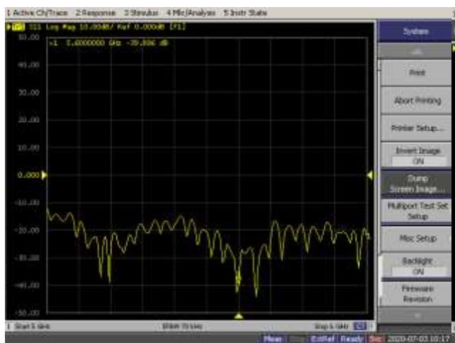
< Figure 1. Measurement result of Head Return Loss>
