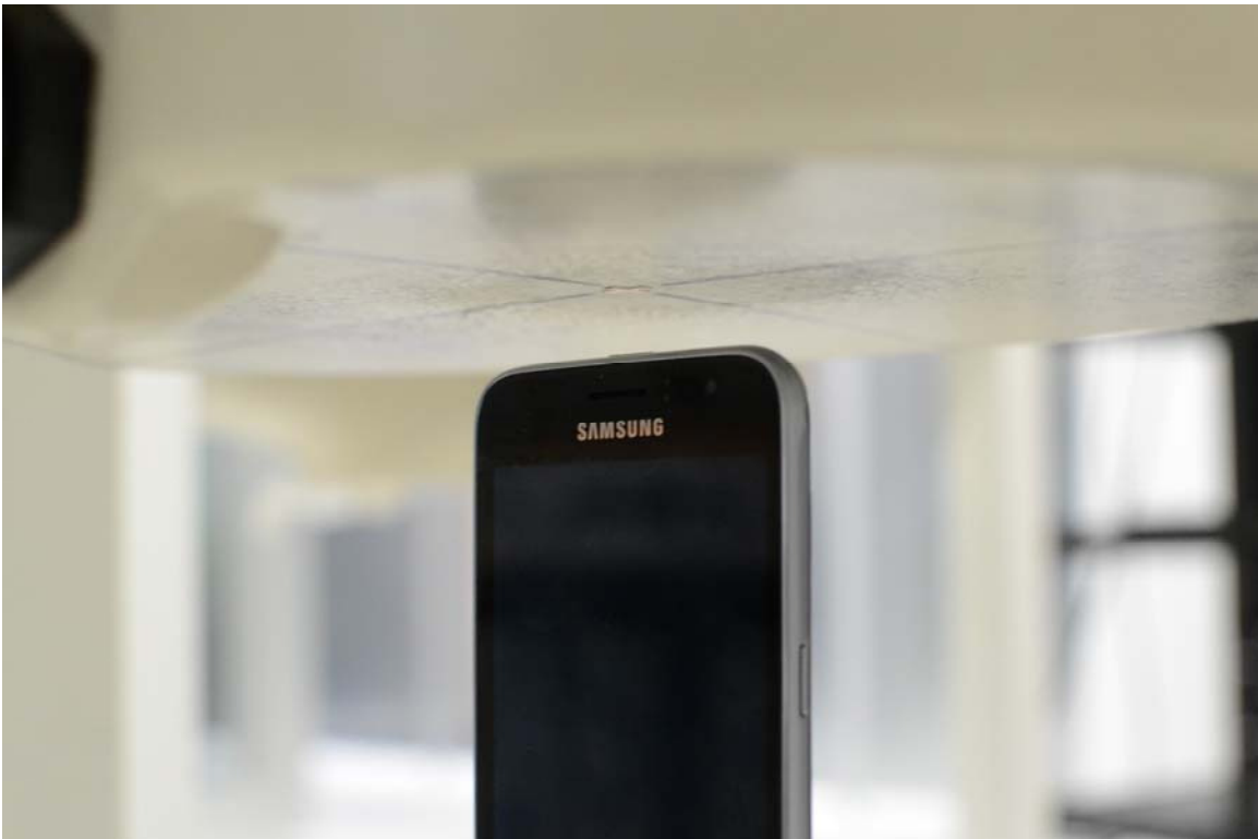
SAR Test Setup Photo 8 – Top Edge (10 mm)
