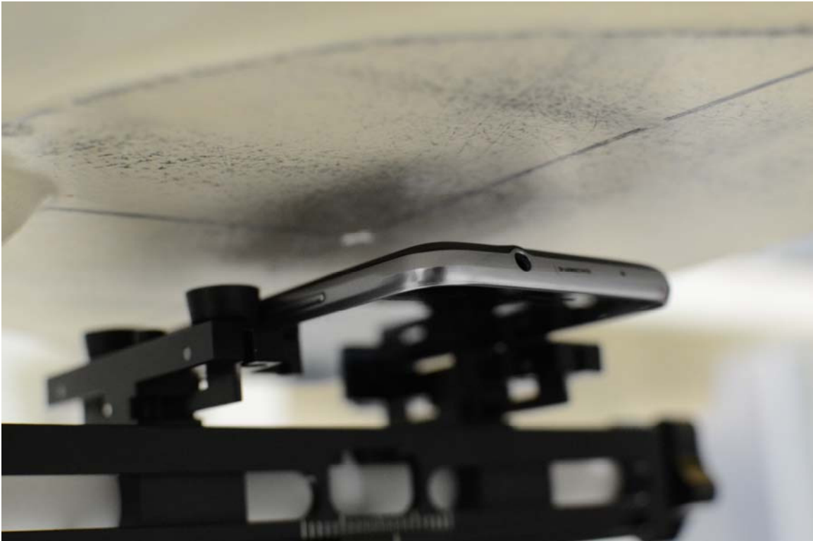
SAR Test Setup Photo 6 – Back Side (15 mm)
