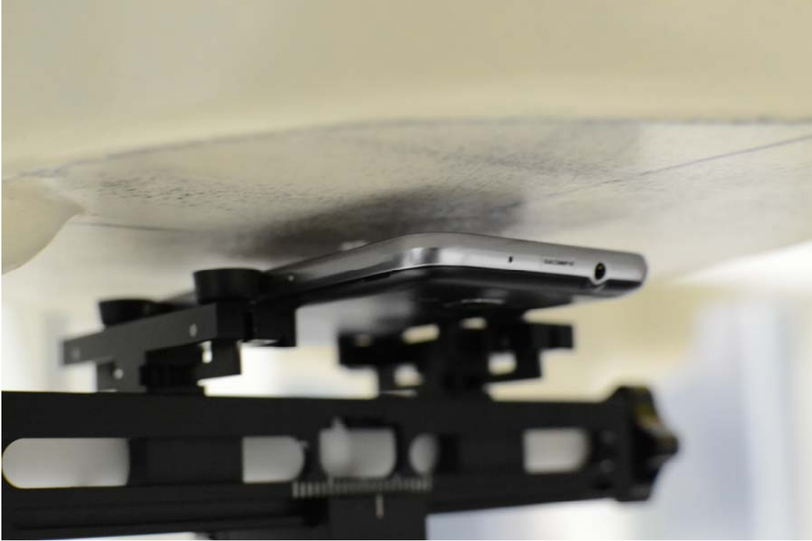
SAR Test Setup Photo 7 – Front Side (10 mm)
