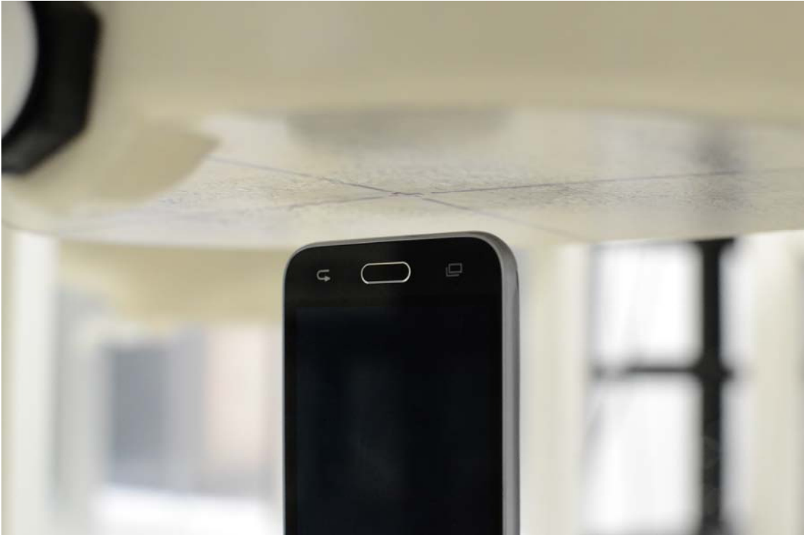
SAR Test Setup Photo 9 – Bottom Edge (10 mm)
