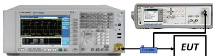
Figure 7-3. Test Instrument & Measurement Setup
