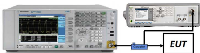
Figure 7-6. Test Instrument & Measurement Setup
