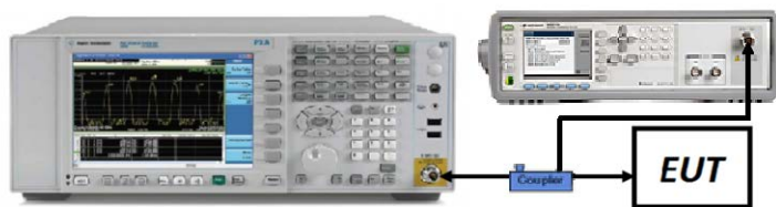
Figure 7-7. Test Instrument & Measurement Setup
