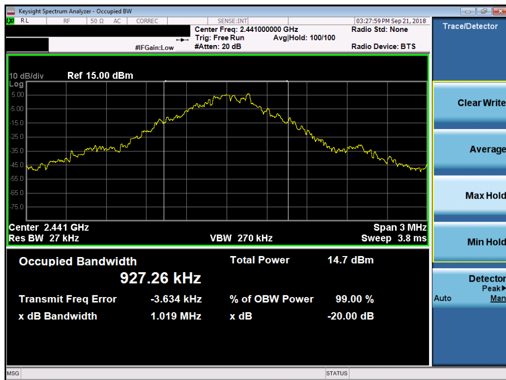
Plot 7-2. 20dB Bandwidth Plot (Bluetooth, 1Mbps – Ch. 39)
