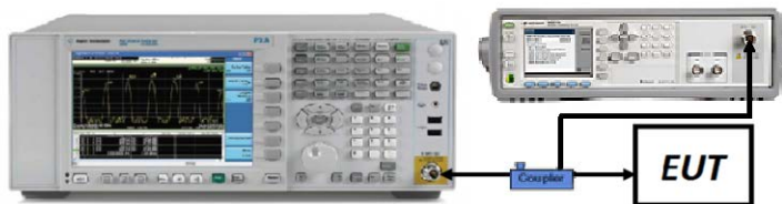
Figure 7-4. Test Instrument & Measurement Setup
