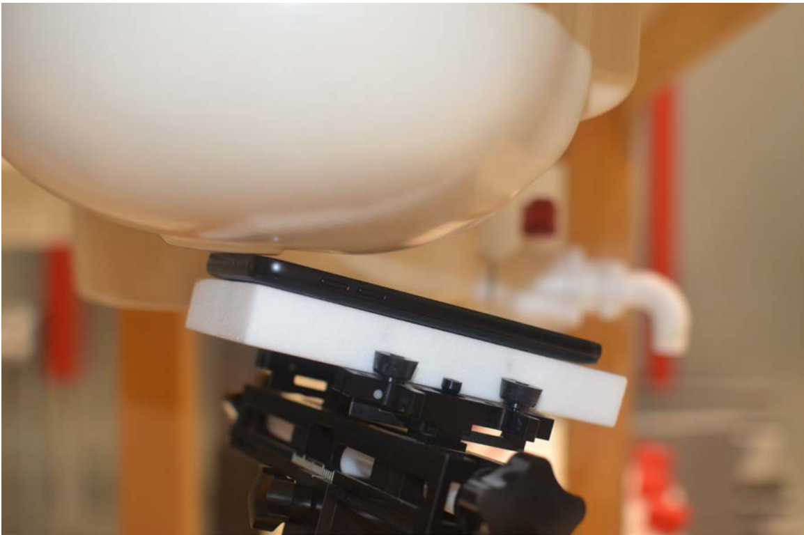
SAR Test Setup Photo 2 – Right Tilt
