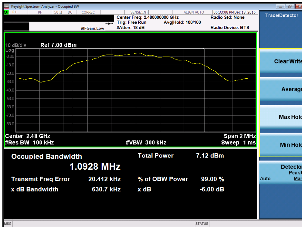
Plot 7-3. 6dB Bandwidth Plot (Bluetooth (LE) – Ch. 39)
