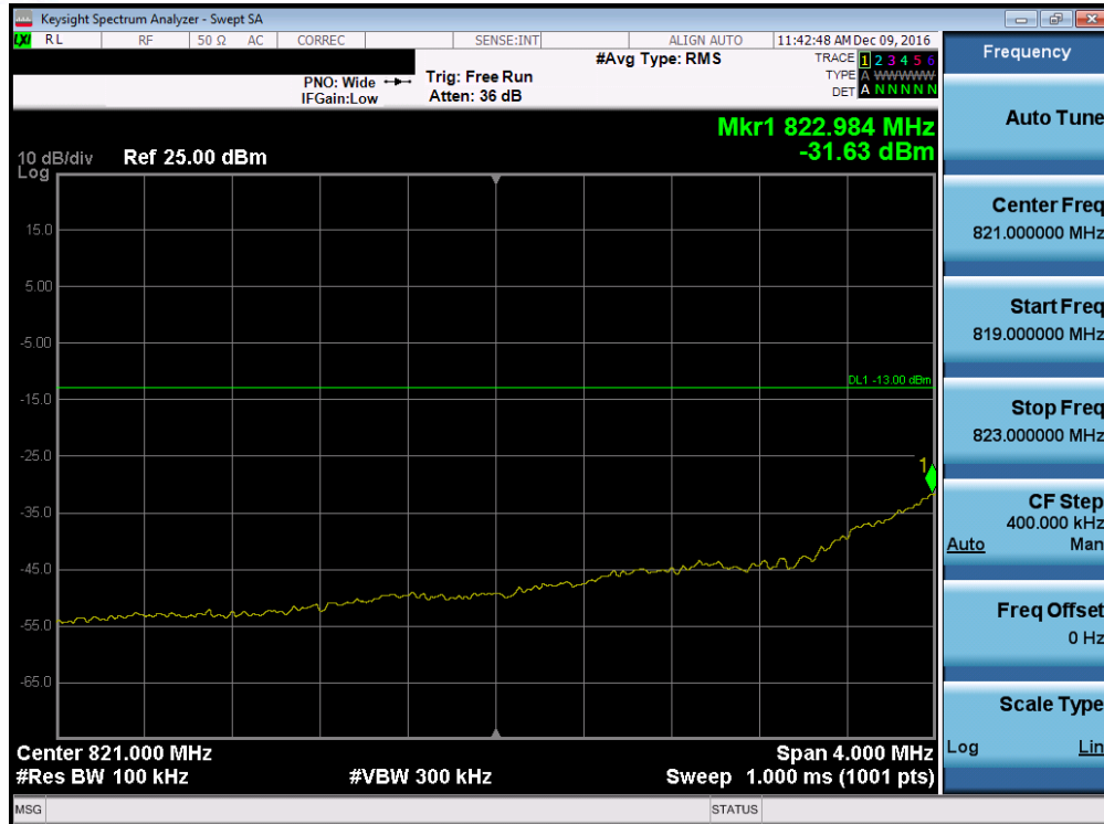
Plot 7-76. Lower Extended Band Edge Plot (Band 5 – 1.4MHz QPSK – RB Size 6)
