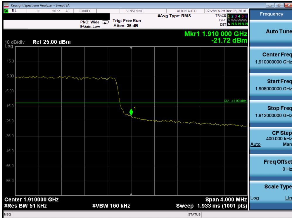
Plot 7-123. Upper Band Edge Plot (Band 2 – 5.0MHz QPSK – RB Size 25)
