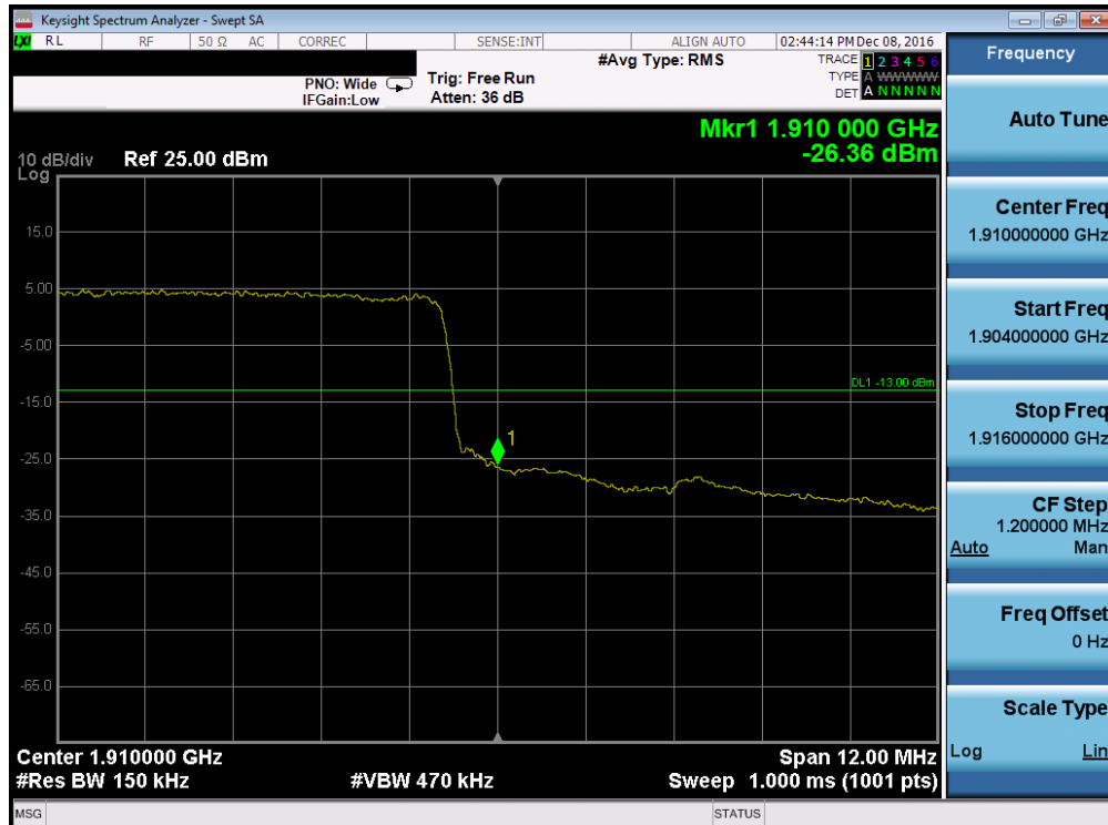
Plot 7-131. Upper Band Edge Plot (Band 2 – 15.0MHz QPSK – RB Size 75)
