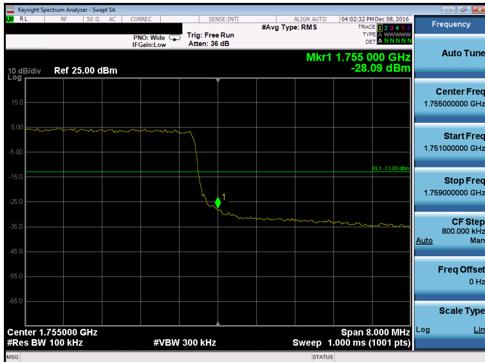
Plot 7-103. Upper Band Edge Plot (Band 4 – 10.0MHz QPSK – RB Size 50)
