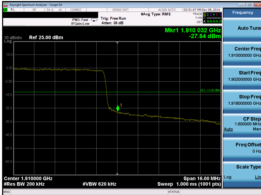
Plot 7-135. Upper Band Edge Plot (Band 2 – 20.0MHz QPSK – RB Size 100)
