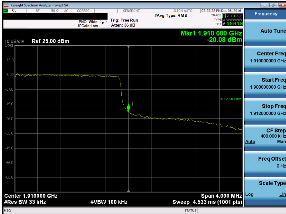
Plot 7-119. Upper Band Edge Plot (Band 2 – 3.0MHz QPSK – RB Size 15)
