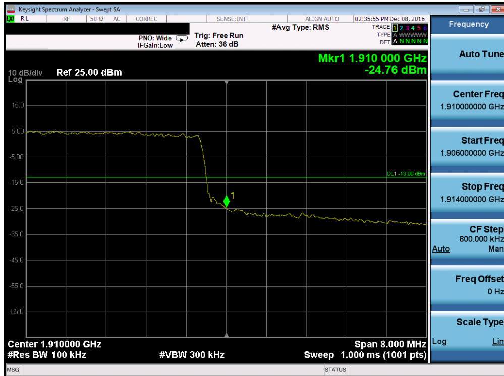
Plot 7-127. Upper Band Edge Plot (Band 2 – 10.0MHz QPSK – RB Size 50)
