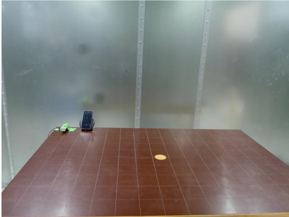
Figure 13. Test Setup – ACLC– <30MHz
