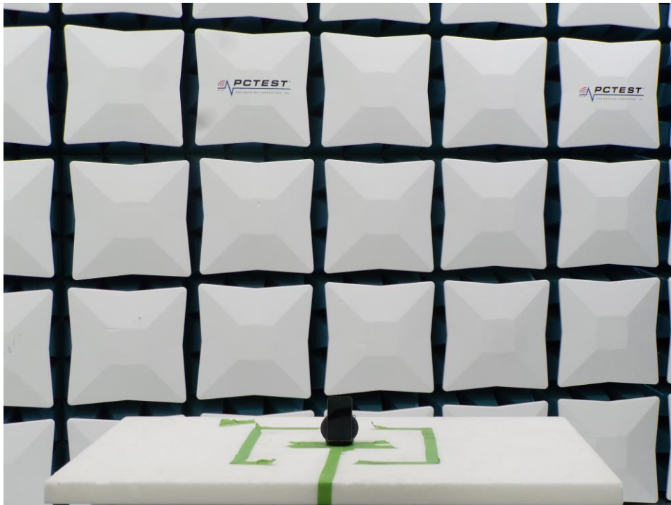
Figure 10. Test Setup – WCP Position – 30MHz-1GHz
