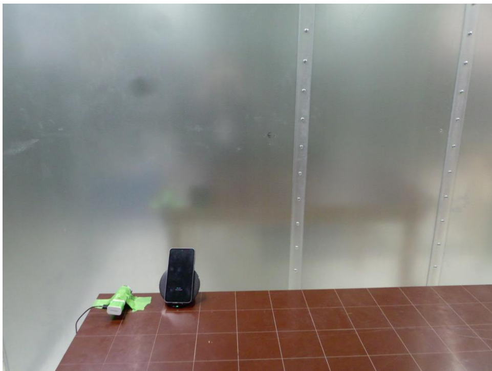
Figure 14. Test Setup – ACLC– <30MHz
