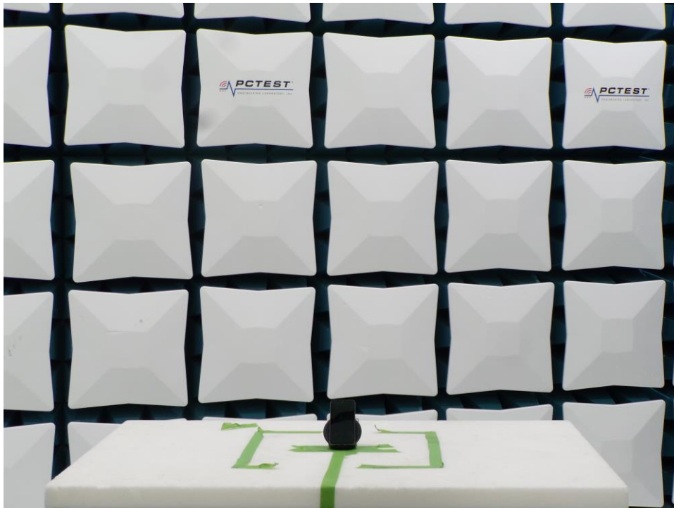
Figure 10. Test Setup – WCP Position – 30MHz-1GHz
