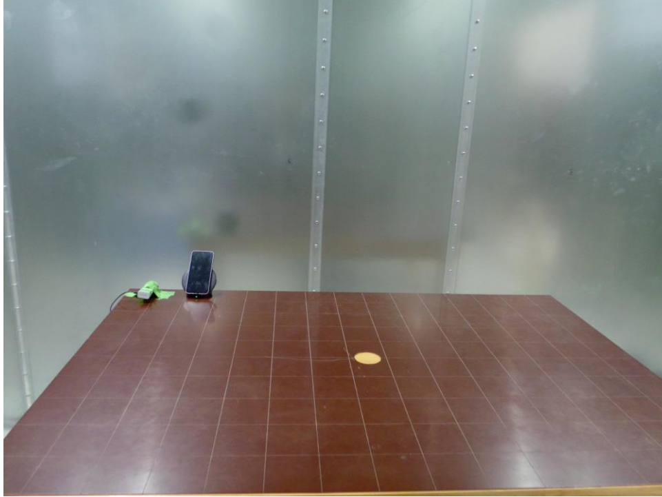
Figure 13. Test Setup – ACLC– <30MHz
