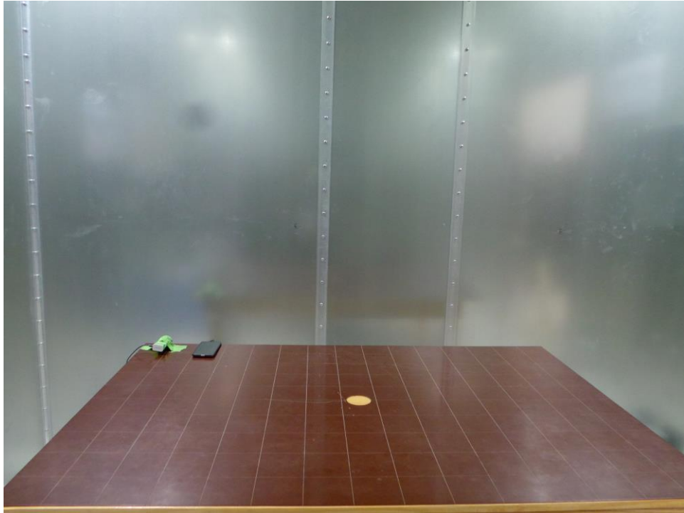
Figure 11. Test Setup – ACLC– <30MHz
