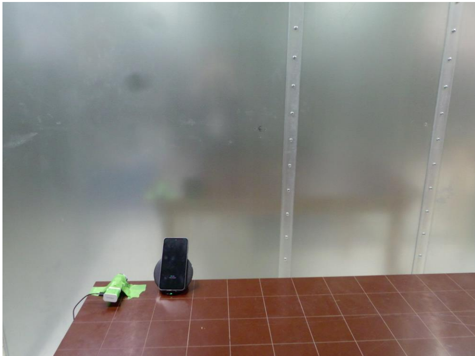
Figure 14. Test Setup – ACLC– <30MHz
