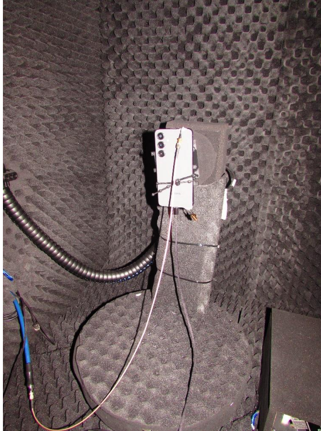
Test setup photo-5 mmW NR radiated power measurement
