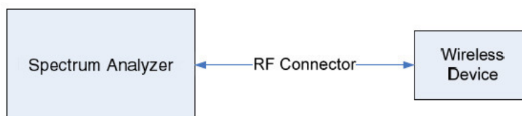
Figure 7-1. Test Instrument & Measurement Setup
