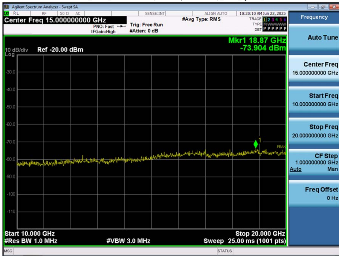
LTE B2_20 M_Conducted Spurious(Above10 G)_Low_QPSK_1RB
