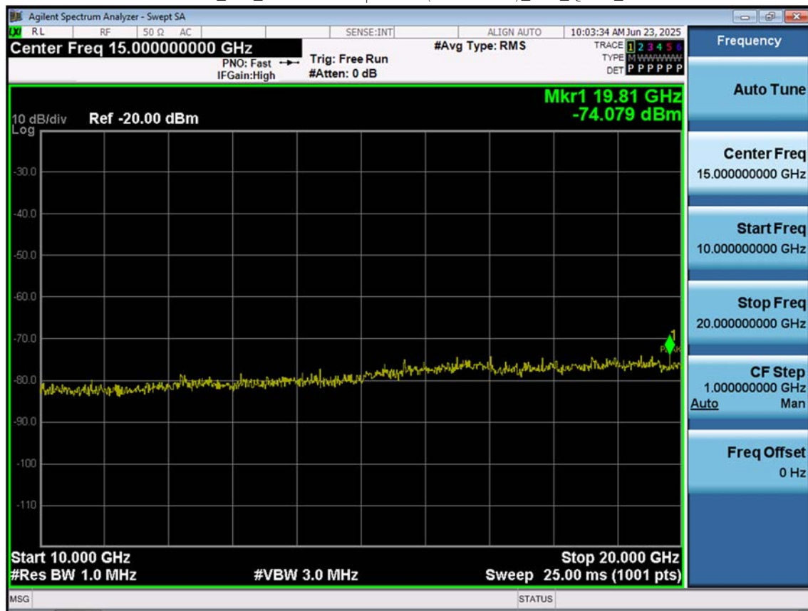
LTE B2_5 M_Conducted Spurious(Above10 G)_Mid_QPSK_1RB
