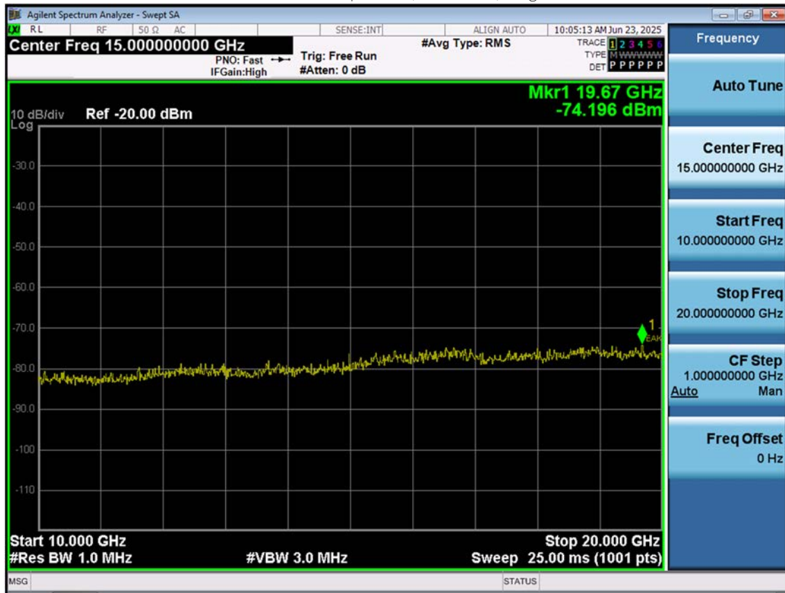
LTE B2_5 M_Conducted Spurious(Above10 G)_High_QPSK_1RB
