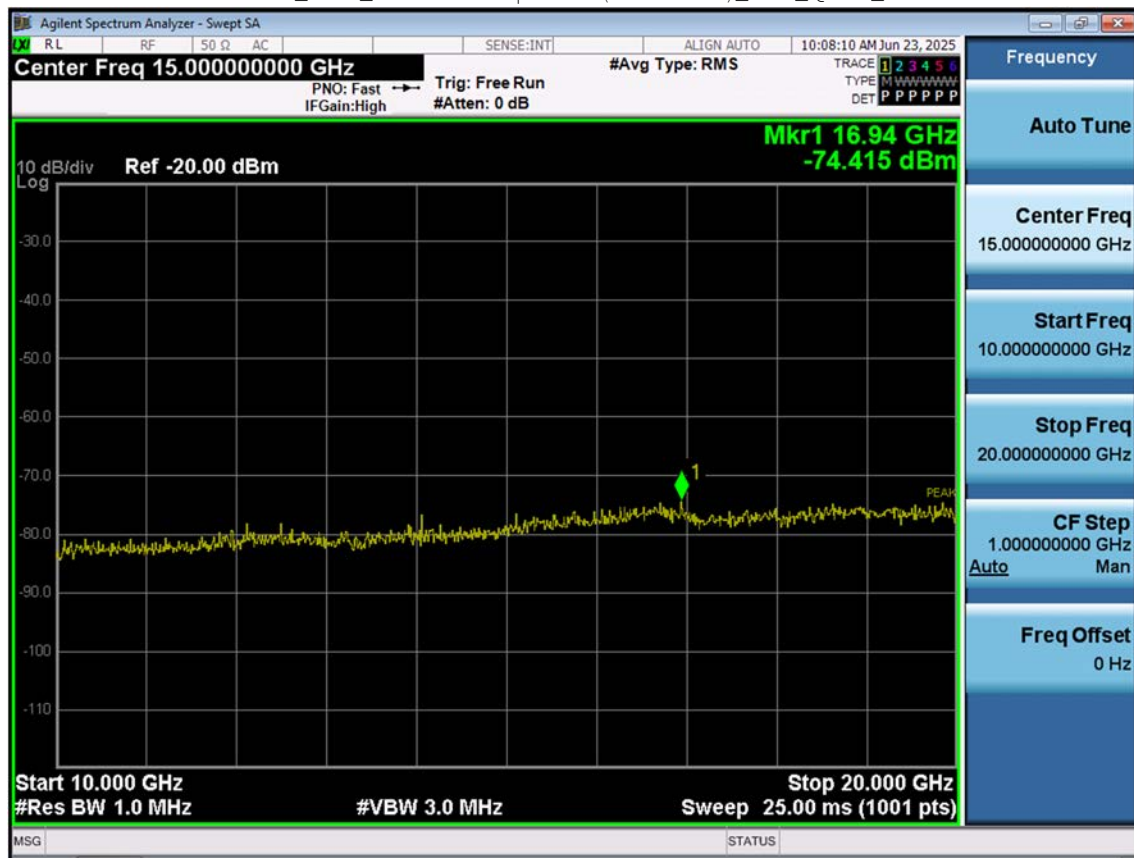
LTE B2_10 M_Conducted Spurious(Above10 G)_Low_QPSK_1RB
