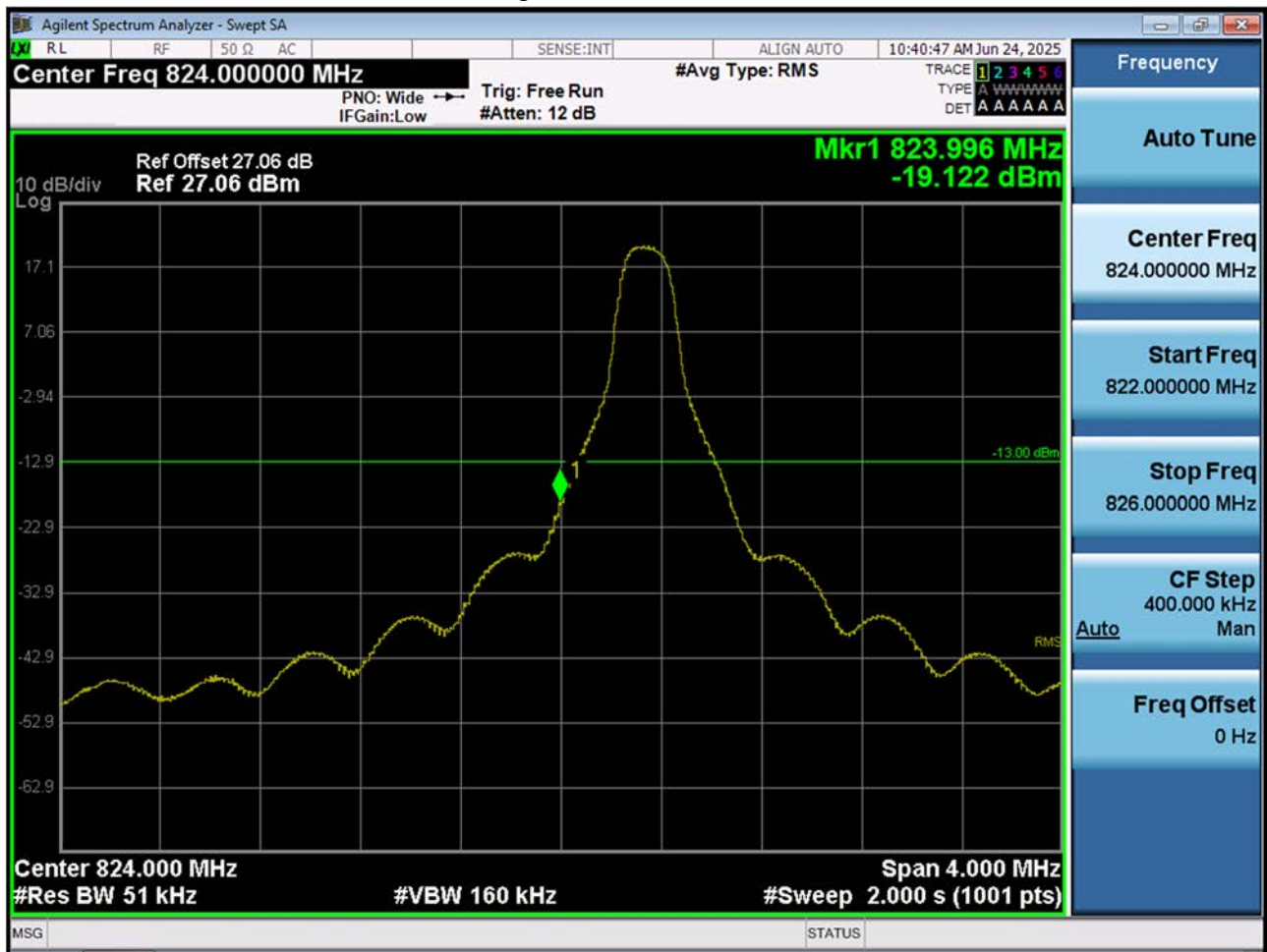
LTE B26_Lower Band Edge Plot (5 M BW Ch.26815 QPSK_RB1_Offset 0)
