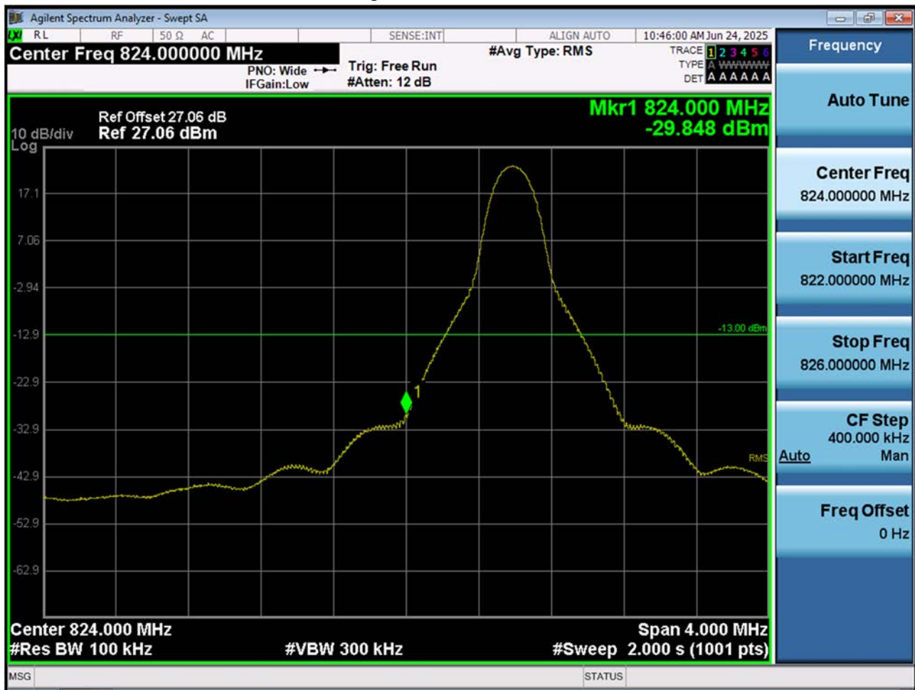
LTE B26_Lower Band Edge Plot (10 M BW Ch.26840 QPSK_RB1_Offset 0)
