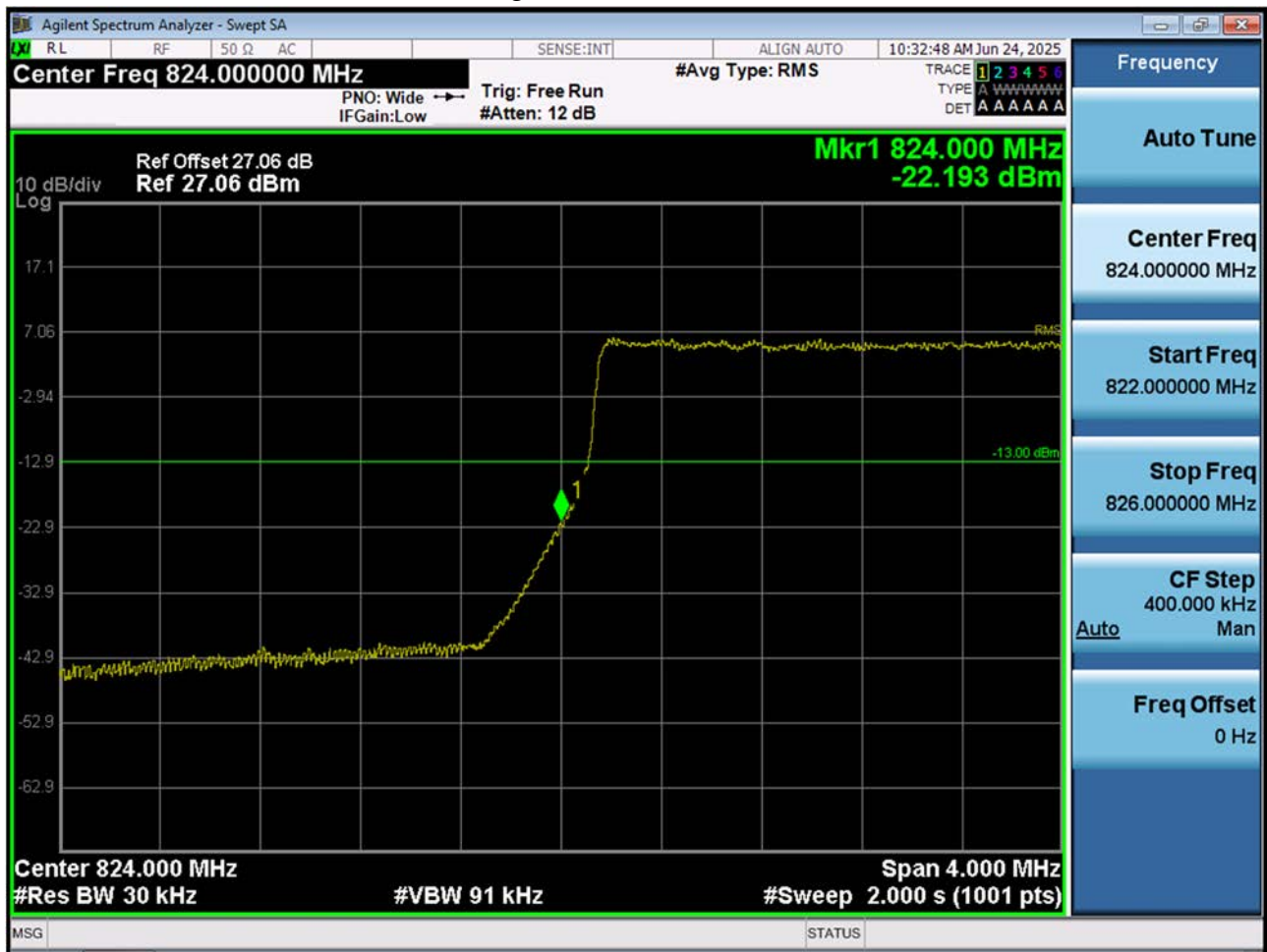
LTE B26_Lower Band Edge Plot (3 M BW Ch.26805 QPSK_RB15_Offset 0)
