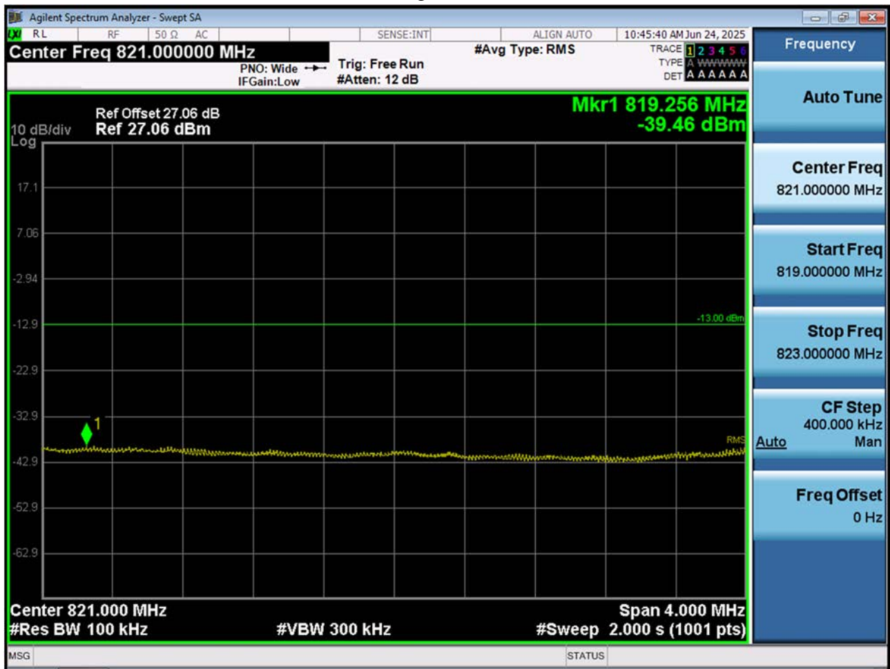
LTE B26_Lower Extended Band Edge Plot (10 M BW Ch.26840 QPSK_RB50_0)
