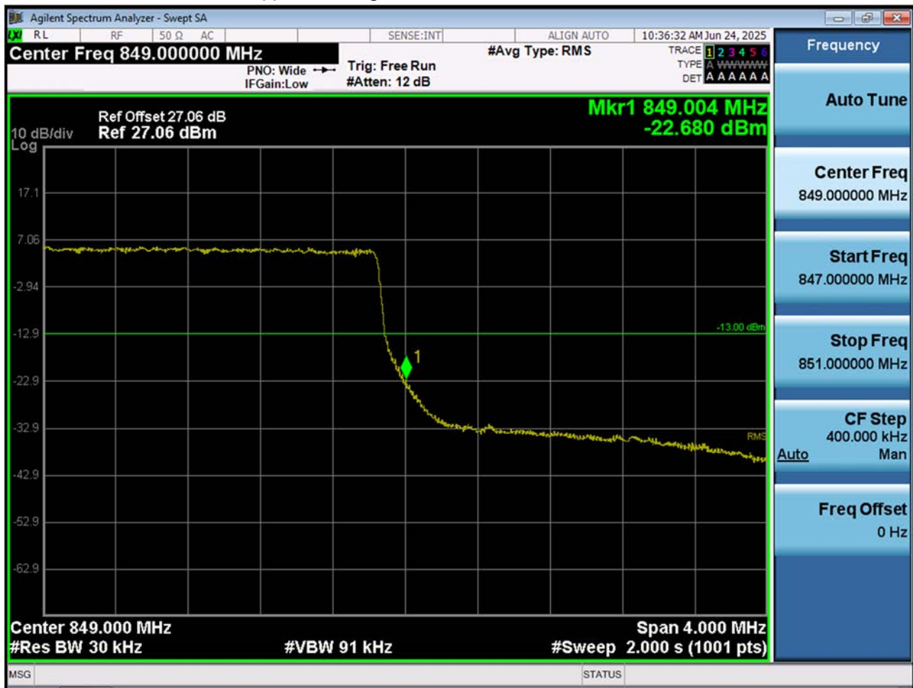
LTE B26_Upper Band Edge Plot (3 M BW Ch.27025 QPSK_RB15_Offset 0)
