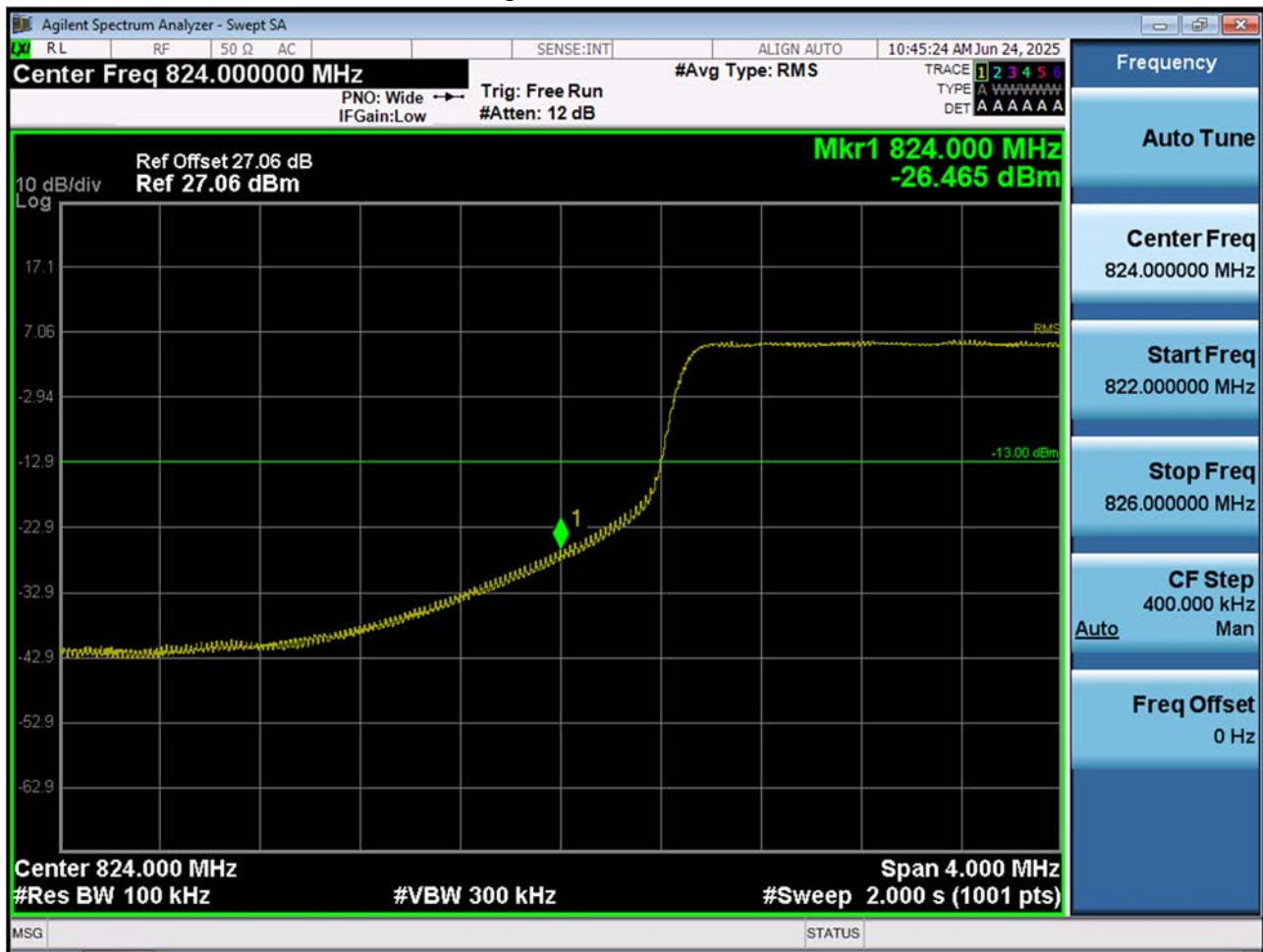
LTE B26_Lower Band Edge Plot (10 M BW Ch.26840 QPSK_RB50_Offset 0)
