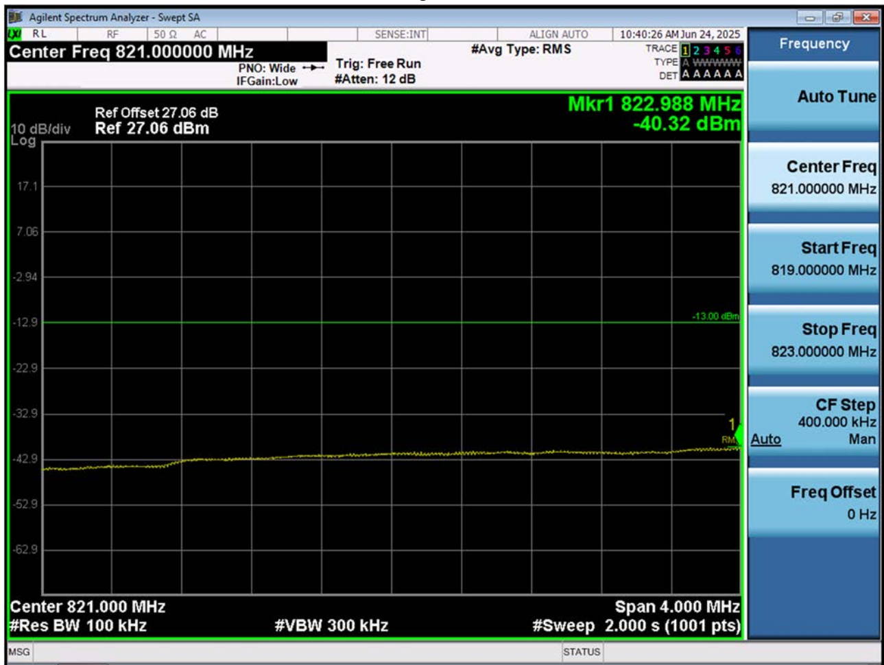
LTE B26_Lower Extended Band Edge Plot (5 M BW Ch.26815 QPSK_RB25_0)
