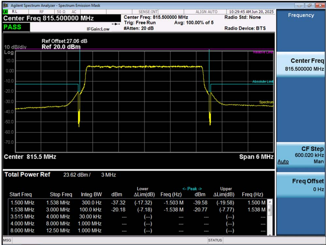
LTE B26_ Lower Channel Edge Plot (3 M BW Ch.26705 QPSK_RB15_Offset 0)
