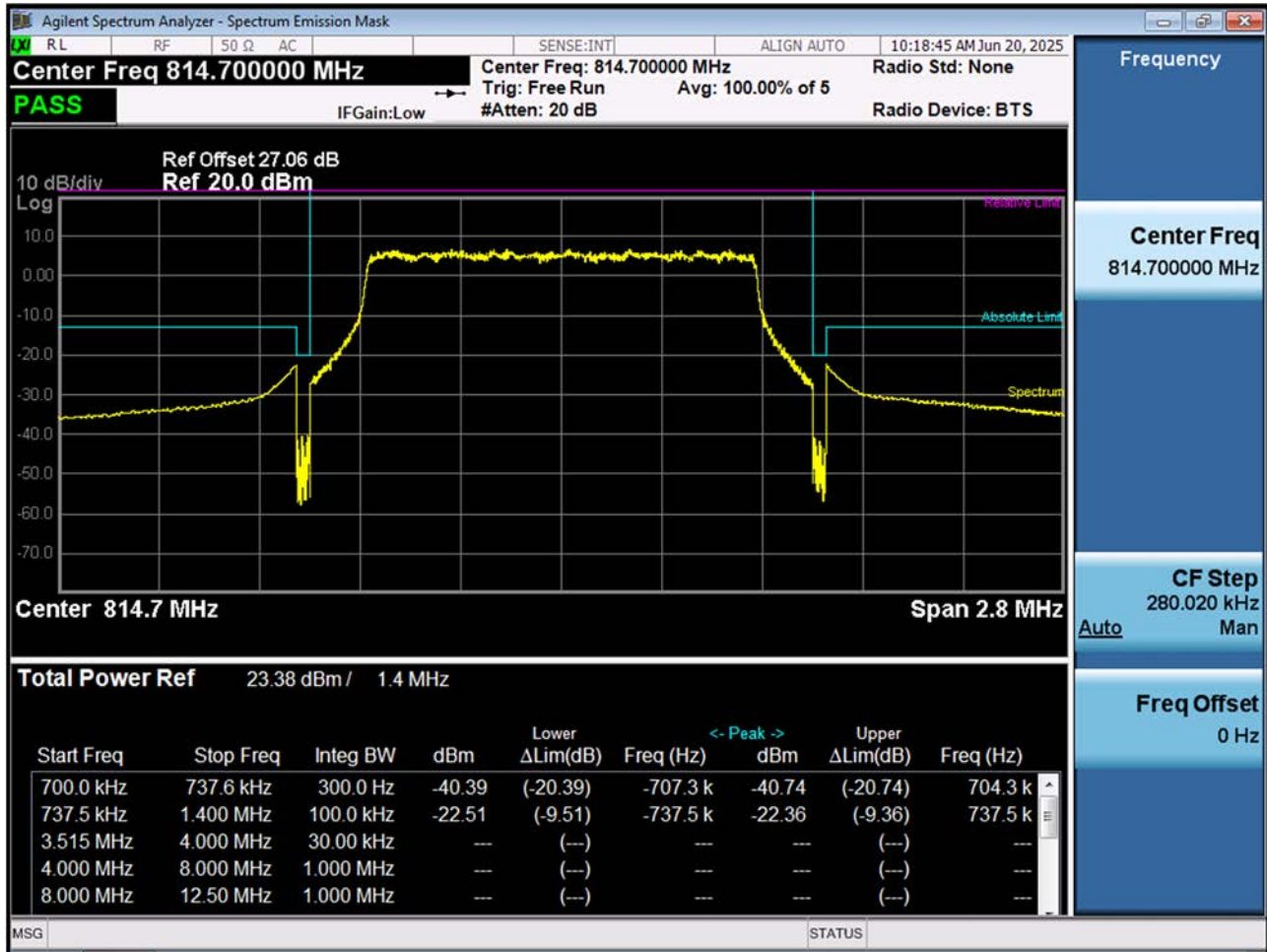
LTE B26_ Lower Channel Edge Plot (1.4 M BW Ch.26697 QPSK_RB6_Offset 0)
