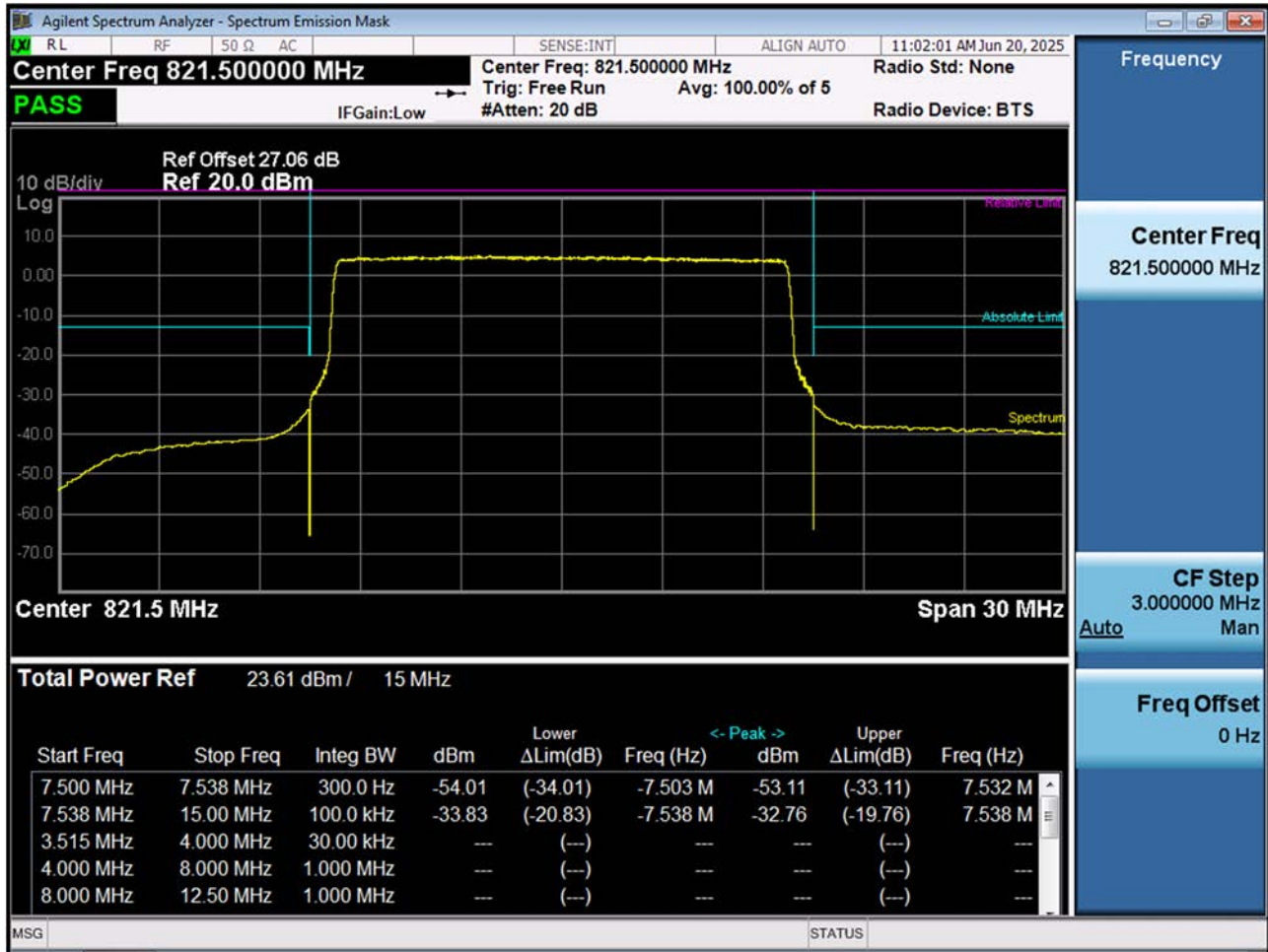
LTE B26_ Low Channel Edge Plot (15 M BW Ch.26765 QPSK RB 75, Offset0)
