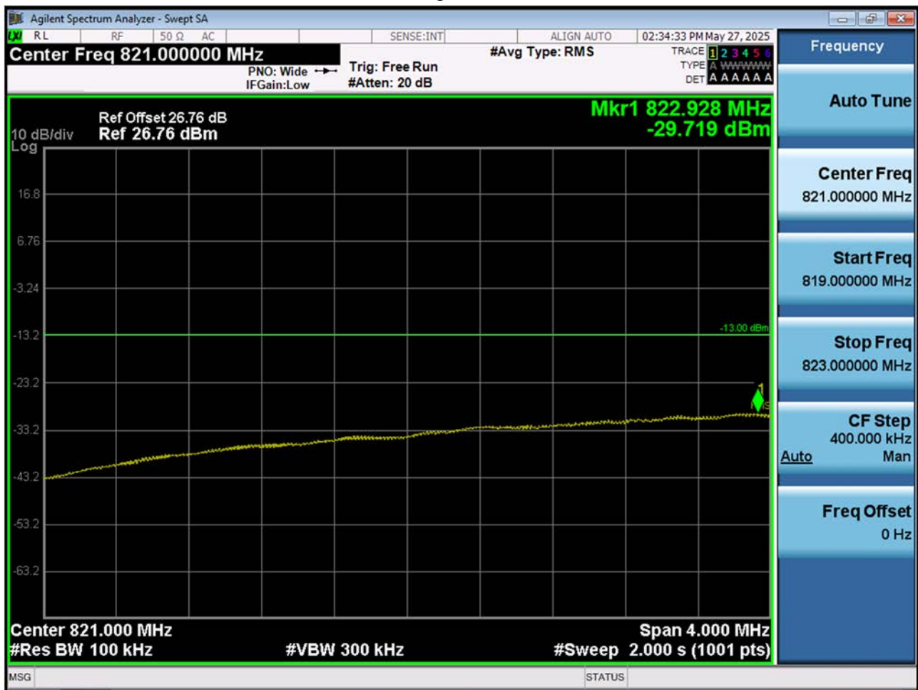
LTE B26_Lower Extended Band Edge Plot (3 M BW Ch.26805 QPSK_RB15_0)
