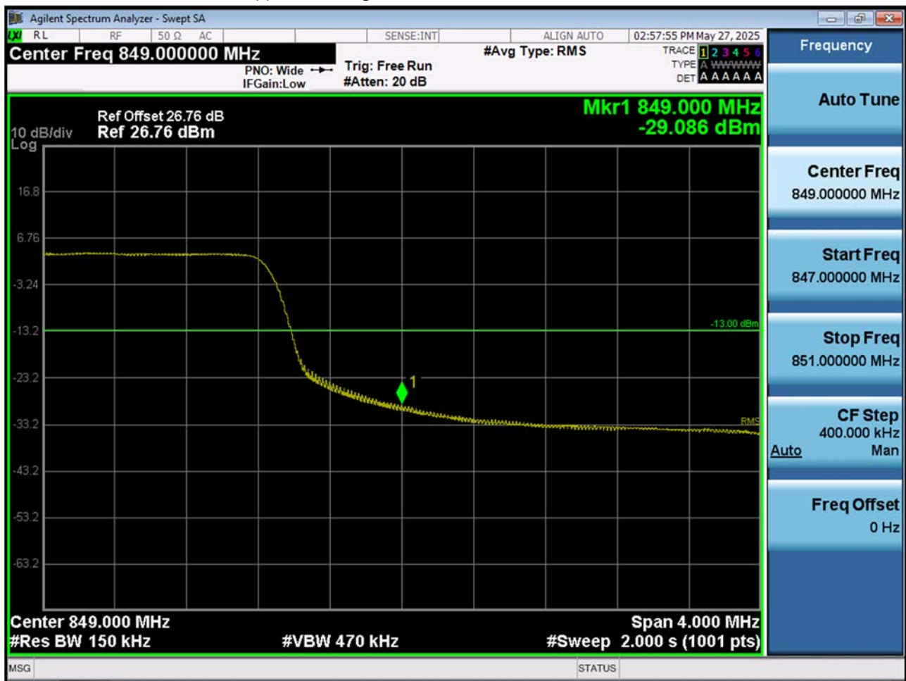
LTE B26_Upper Band Edge Plot (15 M BW Ch.26965 QPSK_RB75_Offset 0)
