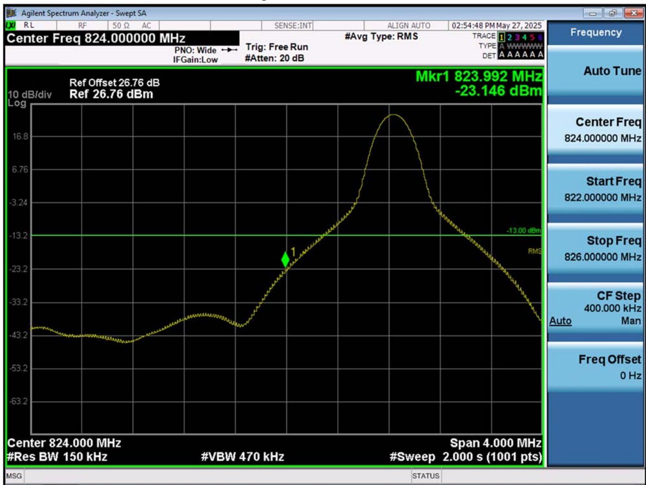
LTE B26_Lower Band Edge Plot (15 M BW Ch.26865 QPSK_RB1_Offset 0)
