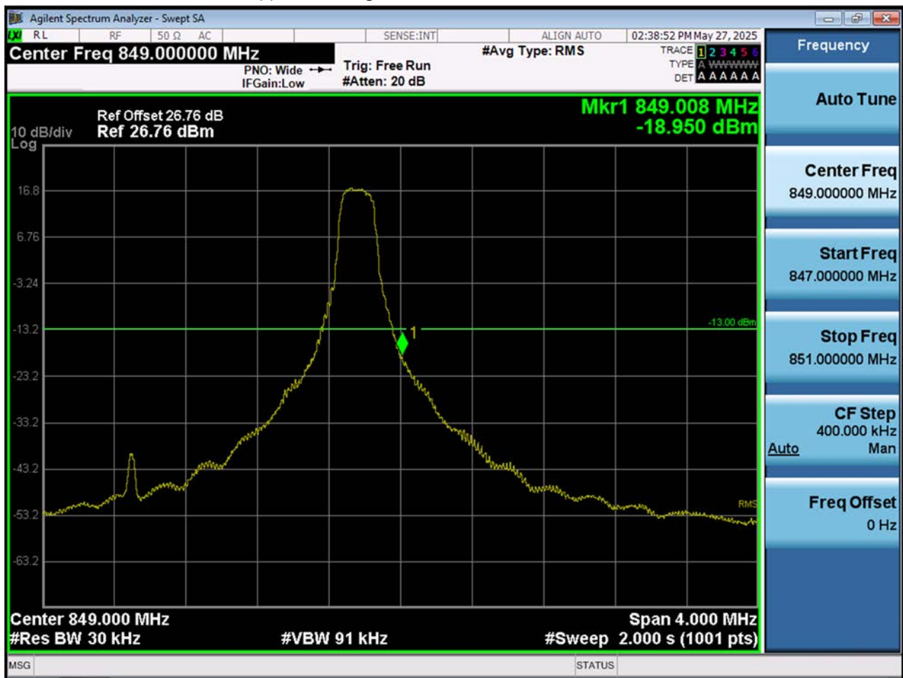
LTE B26_Upper Band Edge Plot (3 M BW Ch.27025 QPSK_RB1_Offset 14)
