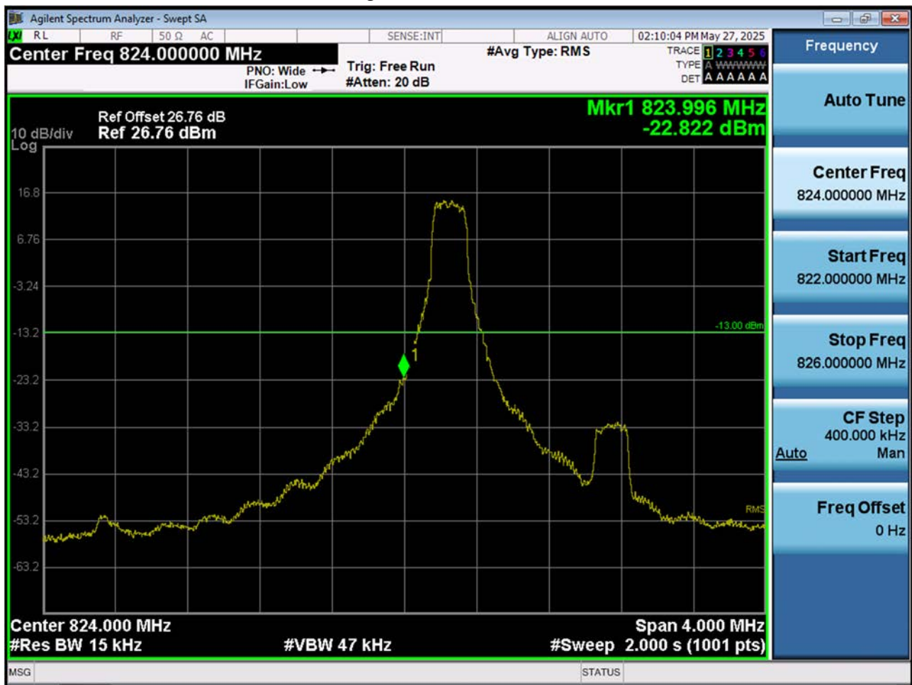
LTE B26_Lower Band Edge Plot (1.4 M BW Ch.26797 QPSK_RB1_Offset 0)
