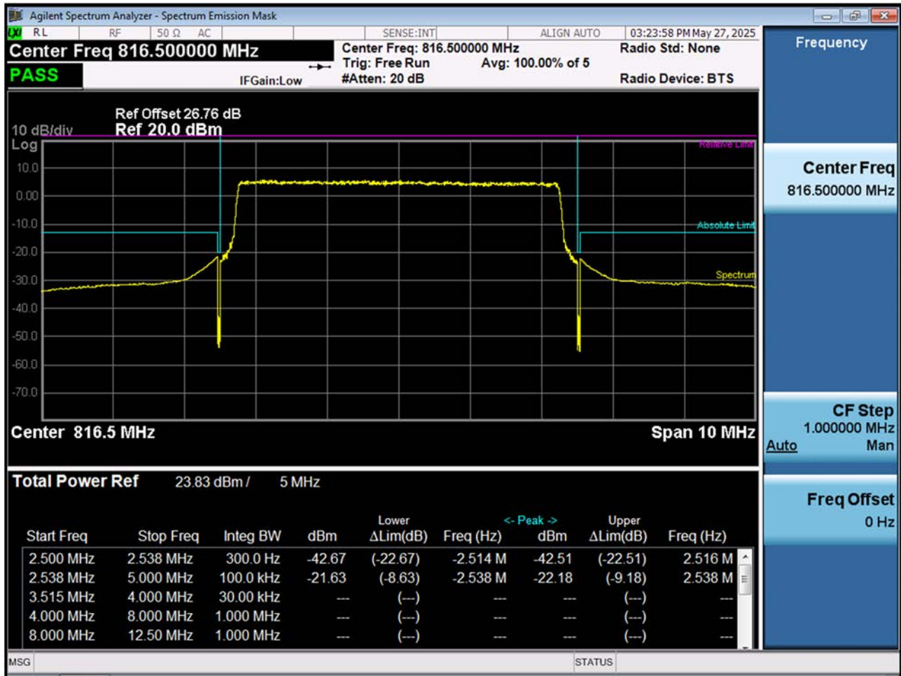
LTE B26_ Lower Channel Edge Plot (5 M BW Ch.26715 QPSK_RB25_Offset 0)
