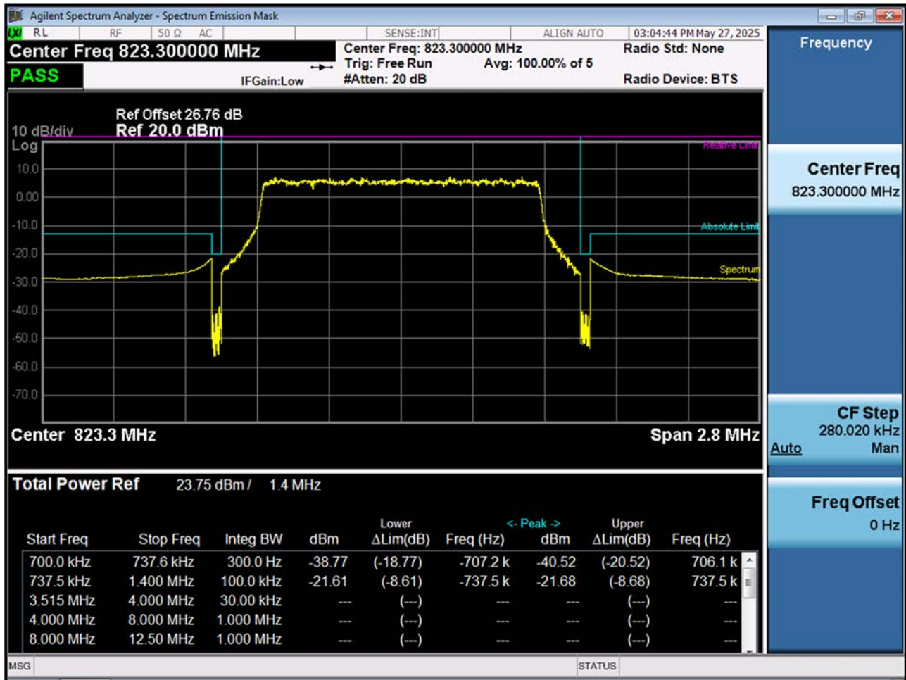
LTE B26_ Upper Channel Edge Plot (1.4 M BW Ch.26783 QPSK_RB6_Offset 0)
