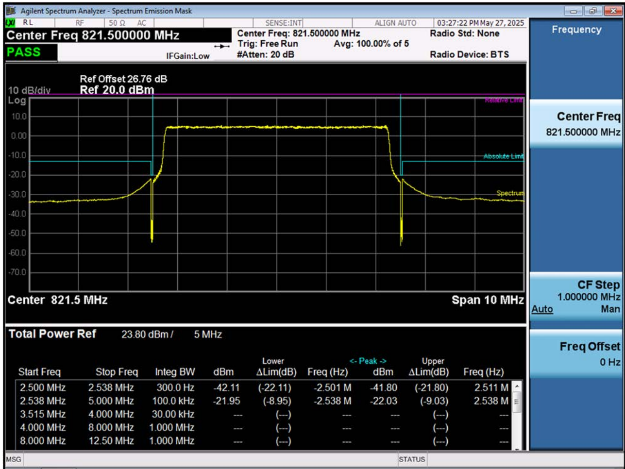
LTE B26_ Upper Channel Edge Plot (5 M BW Ch.26765 QPSK_RB25_Offset 0)
