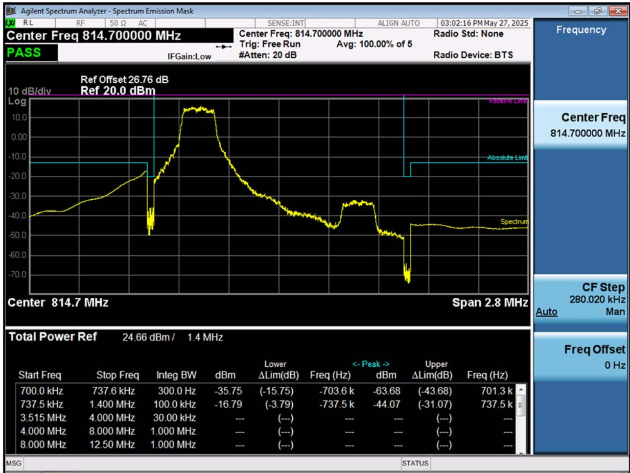
LTE B26_ Lower Channel Edge Plot (1.4 M BW Ch.26697 QPSK RB 1, Offset 0)
