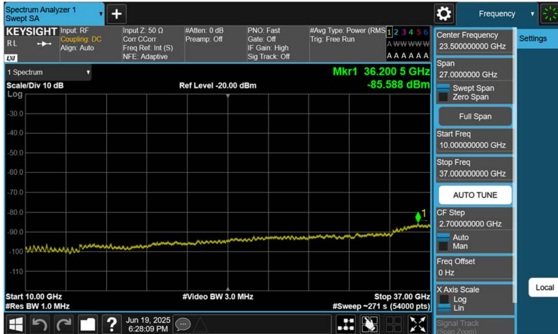
NR48_40 M_Conducted Spurious(Above10 G)_Low_BPSK_1RB
