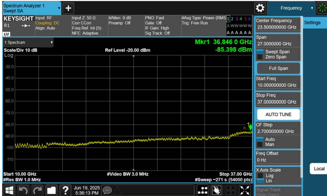
NR48_20 M_Conducted Spurious(Above10 G)_Low_BPSK_1RB
