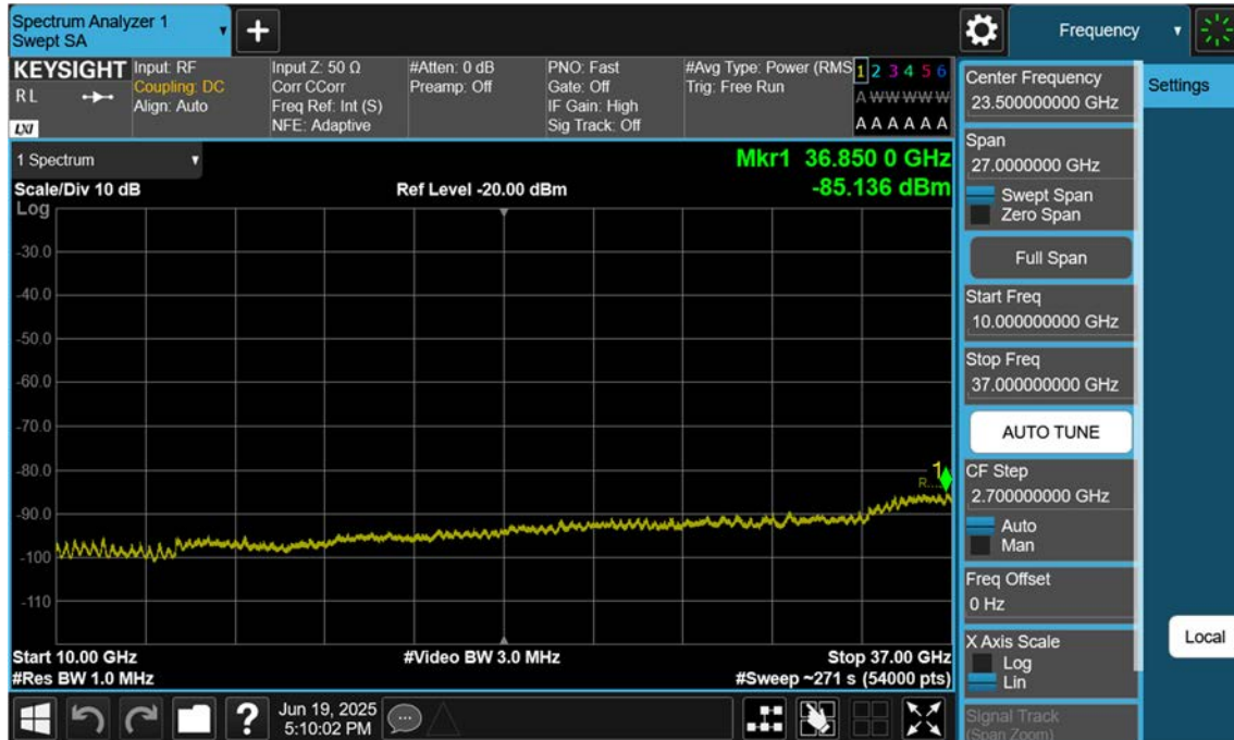
NR48_15 M_Conducted Spurious(Above10 G)_Low_BPSK_1RB
