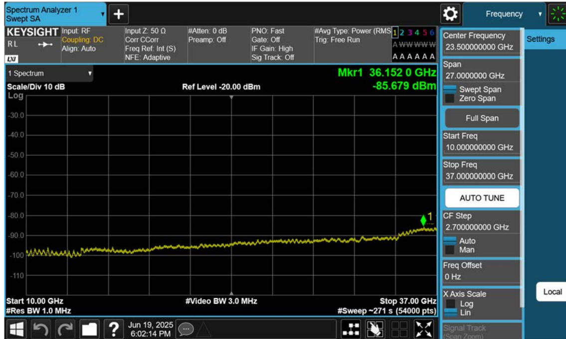
NR48_30 M_Conducted Spurious(Above10 G)_Low_BPSK_1RB
