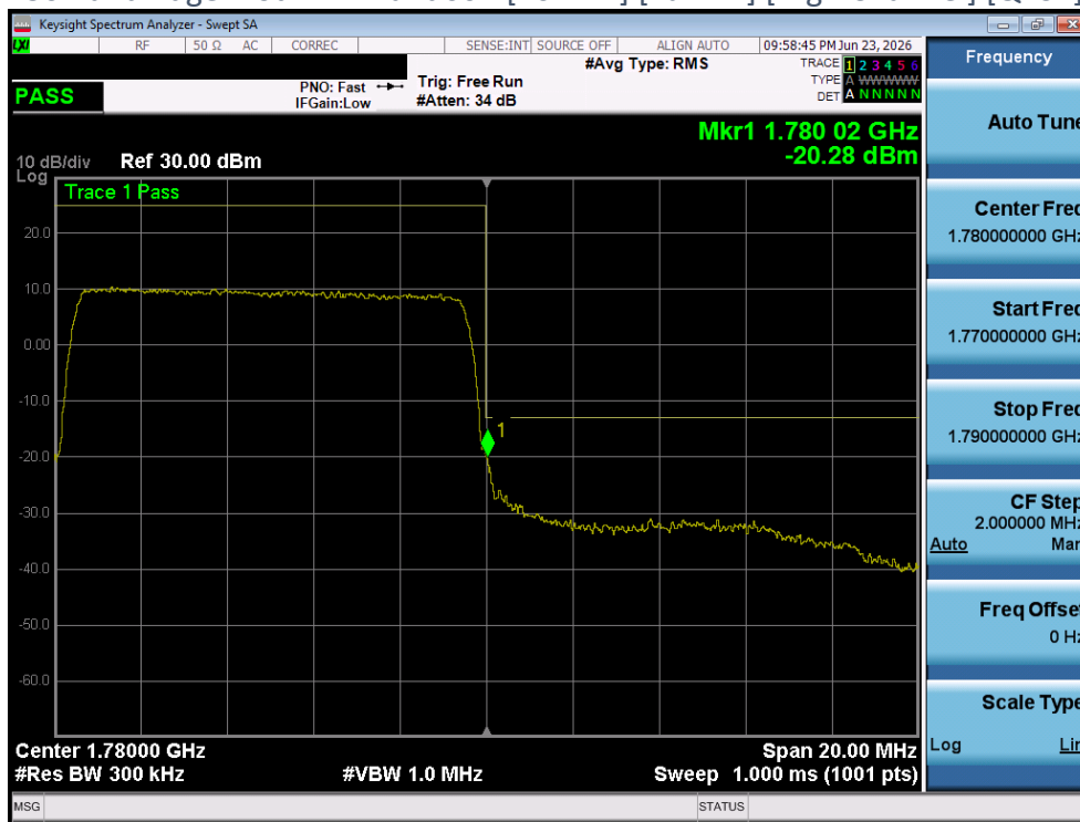
Plot 4-130 Band Edge Plot - LTE Band66 - [10MHz] [Full RB] [High Channel] [QPSK] [Ant 1]
