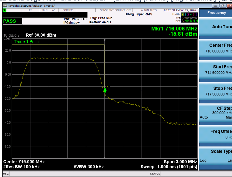
Plot 4-112 Band Edge Plot - LTE Band12/17 - [1.4MHz] [Full RB] [High Channel] [QPSK] [Ant 1]
