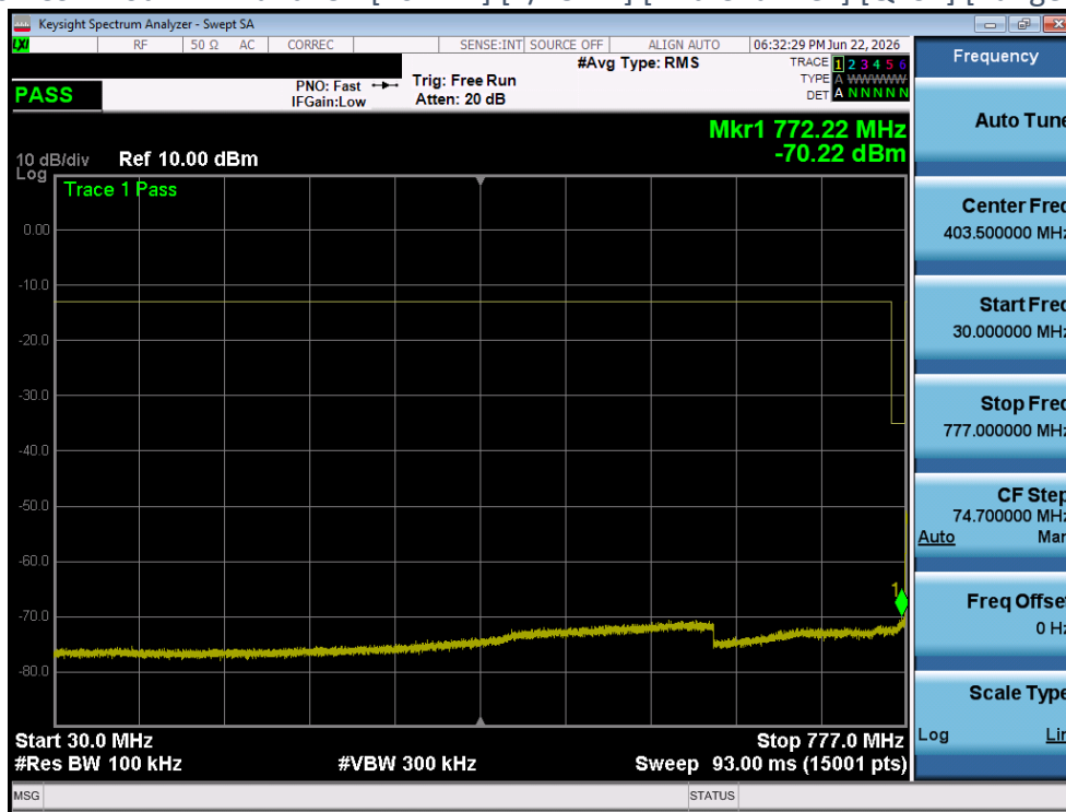
Plot 4-162 CSE Plot - LTE Band13 - [10MHz] [50/0 RB] [Mid Channel] [QPSK] [Range B] [Ant 1]
