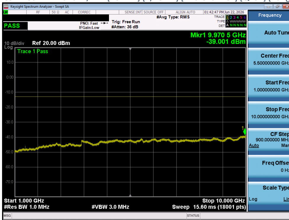
Plot 4-186 CSE Plot - LTE Band12/17 - [10MHz] [50/0 RB] [High Channel] [QPSK] [Range A] [Ant 2]
