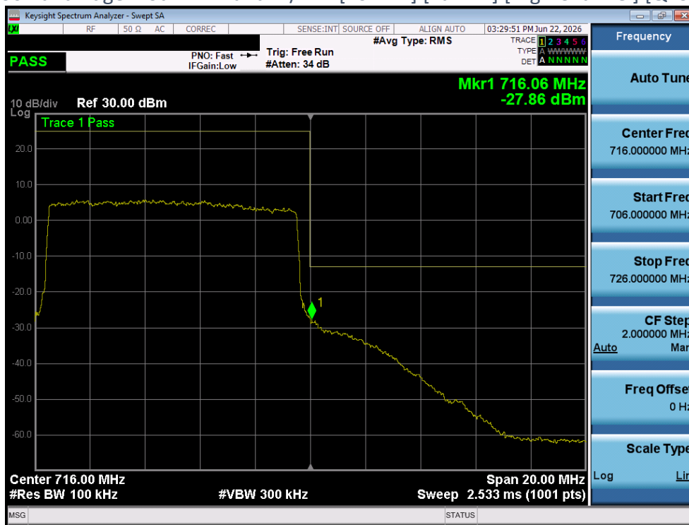
Plot 4-106 Band Edge Plot - LTE Band12/17 - [10MHz] [Full RB] [High Channel] [QPSK] [Ant 1]
