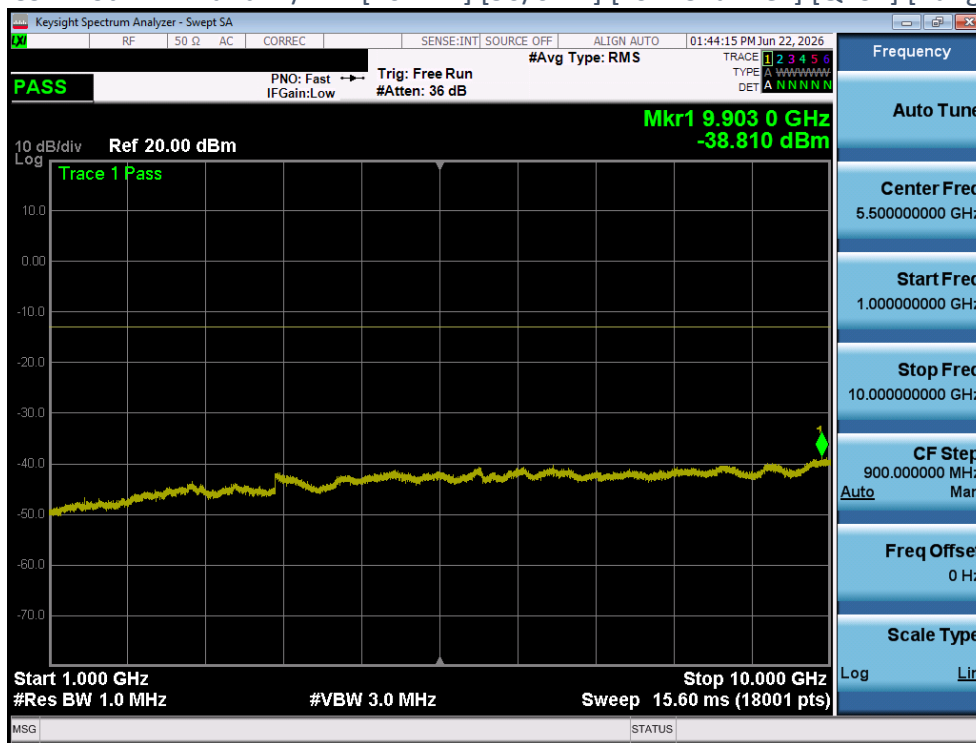
Plot 4-182 CSE Plot - LTE Band12/17 - [10MHz] [50/0 RB] [Low Channel] [QPSK] [Range C] [Ant 2]
