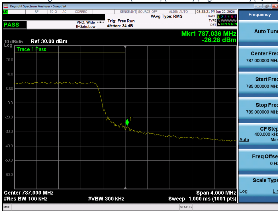
Plot 4-102 Band Edge Plot - LTE Band13 - [10MHz] [Full RB] [High Channel] [QPSK] [Ant 2]
