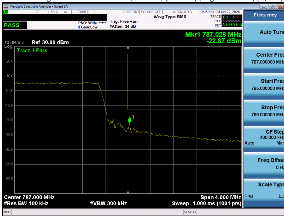
Plot 4-98 Band Edge Plot - LTE Band13 - [10MHz] [Full RB] [High Channel] [QPSK] [Ant 1]
