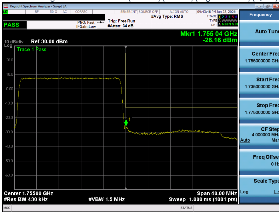
Plot 4-138 Band Edge Plot - LTE Band4 - [15MHz] [Full RB] [High Channel] [QPSK] [Ant 1]
