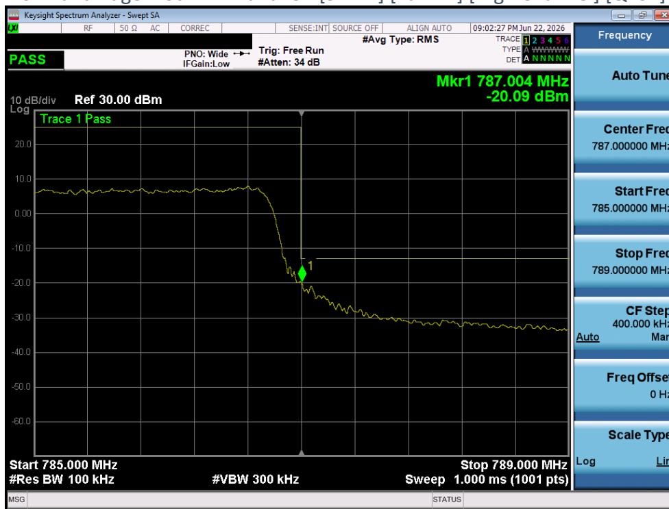
Plot 4-104 Band Edge Plot - LTE Band13 - [5MHz] [Full RB] [High Channel] [QPSK] [Ant 2]
