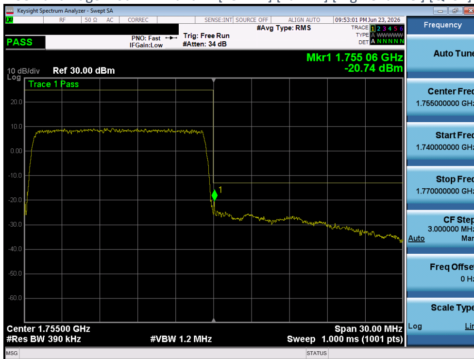
Plot 4-138 Band Edge Plot - LTE Band4 - [15MHz] [Full RB] [High Channel] [QPSK] [Ant 1]
