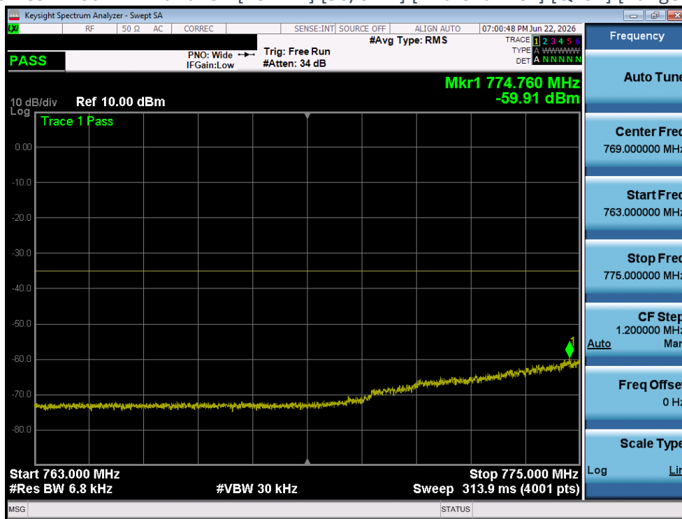
Plot 4-162 CSE Plot - LTE Band13 - [10MHz] [50/0 RB] [Mid Channel] [QPSK] [Range B] [Ant 1]
