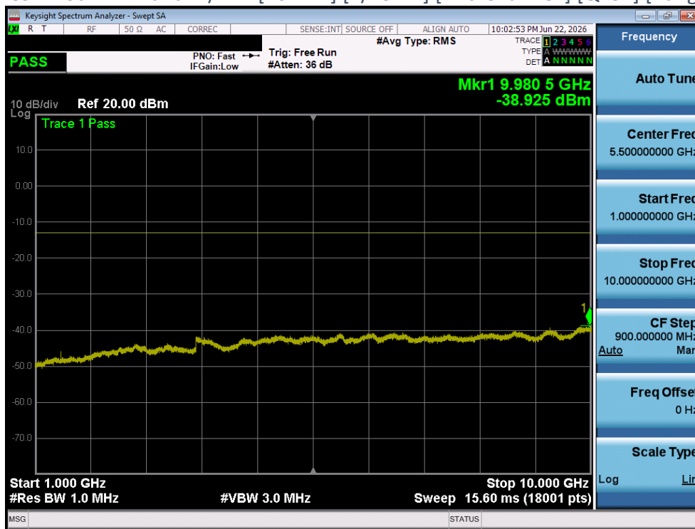
Plot 4-176 CSE Plot - LTE Band12/17 - [10MHz] [1/25 RB] [Mid Channel] [QPSK] [Range C] [Ant 1]
