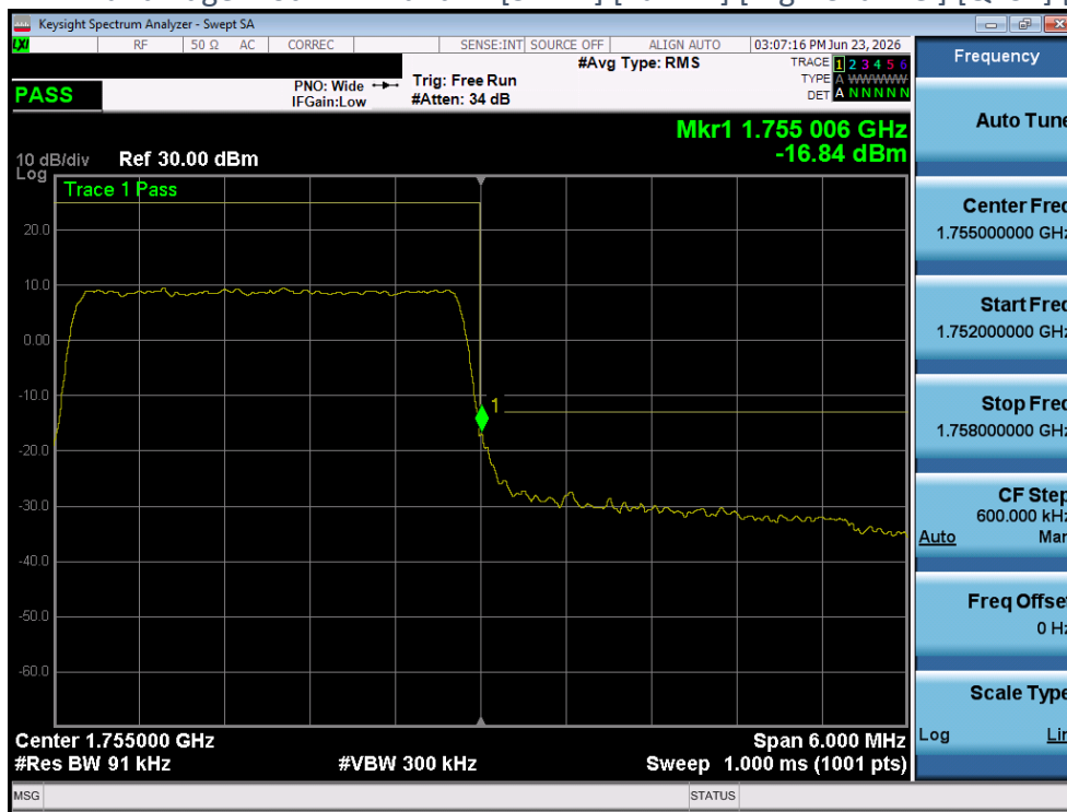
Plot 4-142 Band Edge Plot - LTE Band4 - [1.4MHz] [Full RB] [High Channel] [QPSK] [Ant 1]
