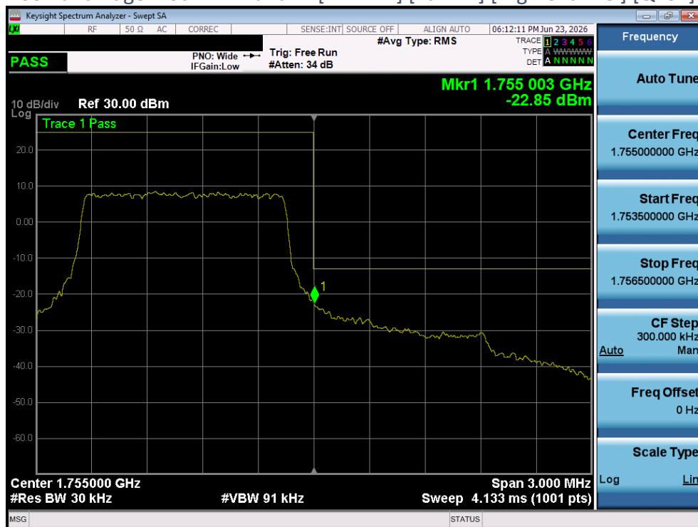
Plot 4-160 Band Edge Plot - LTE Band4 - [1.4MHz] [Full RB] [High Channel] [QPSK] [Ant 2]
