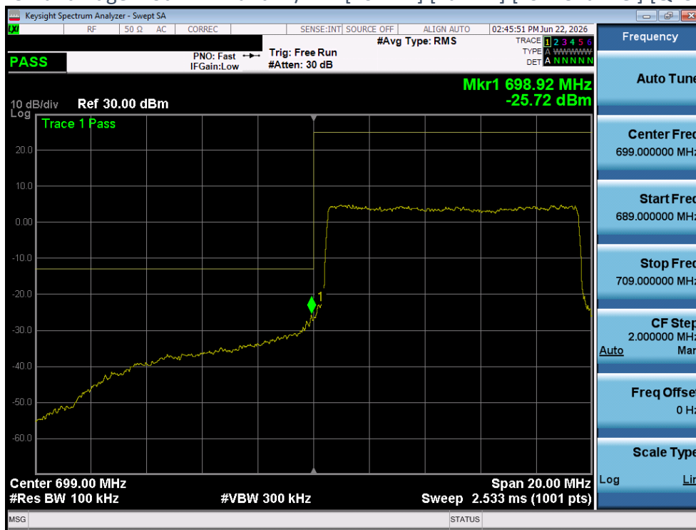
Plot 4-116 Band Edge Plot - LTE Band12/17 - [10MHz] [Full RB] [High Channel] [QPSK] [Ant 2]
