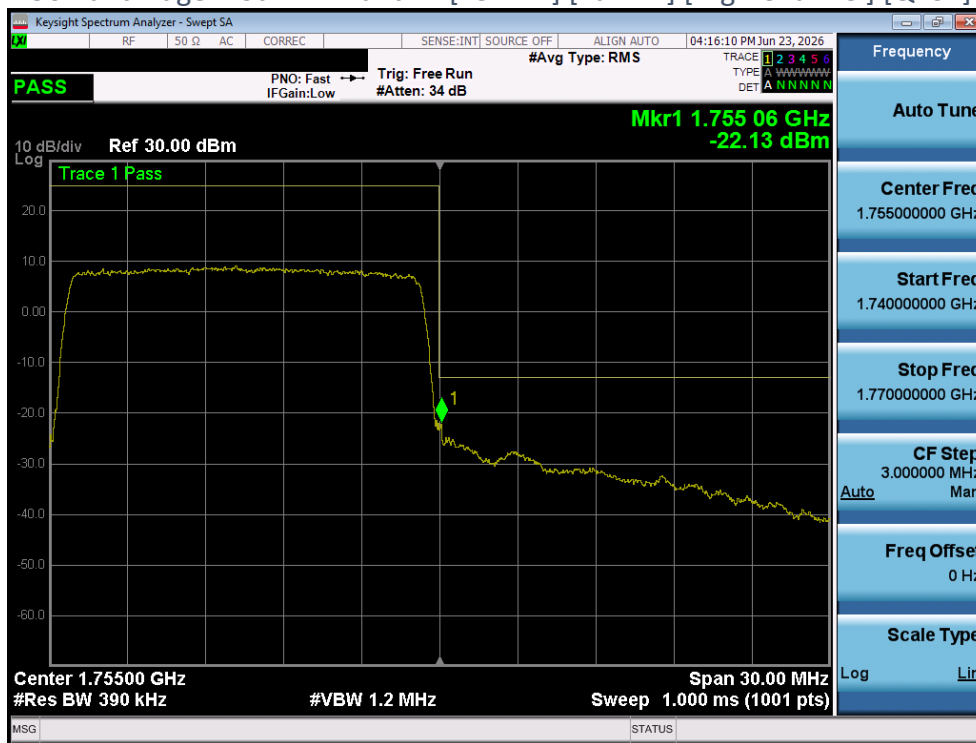
Plot 4-156 Band Edge Plot - LTE Band4 - [15MHz] [Full RB] [High Channel] [QPSK] [Ant 2]
