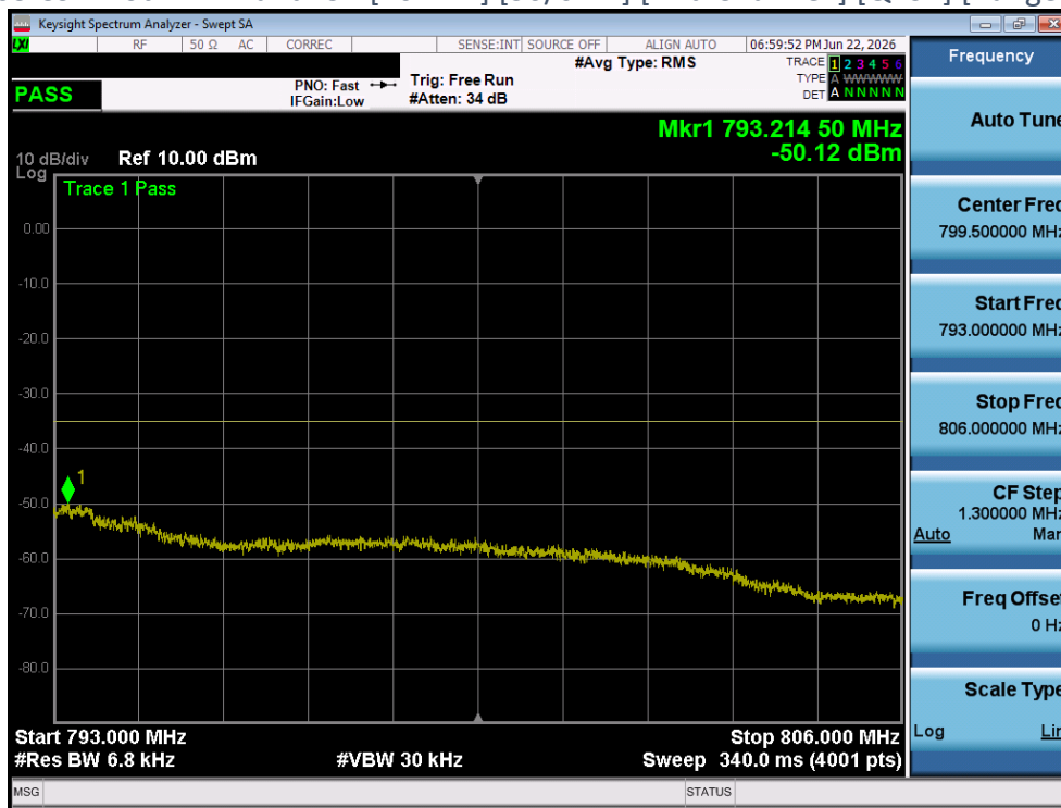
Plot 4-164 CSE Plot - LTE Band13 - [10MHz] [1/25 RB] [Mid Channel] [QPSK] [Range D] [Ant 1]
