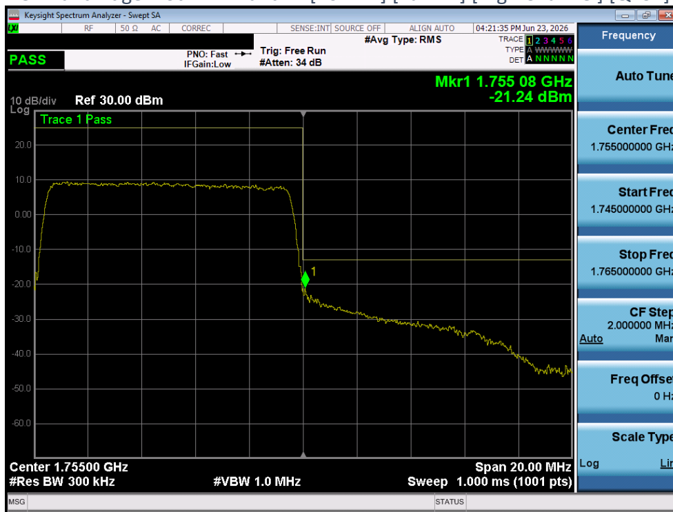
Plot 4-158 Band Edge Plot - LTE Band4 - [5MHz] [Full RB] [High Channel] [QPSK] [Ant 2]
