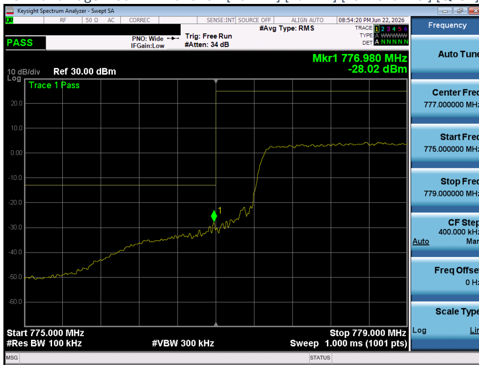
Plot 4-102 Band Edge Plot - LTE Band13 - [10MHz] [Full RB] [High Channel] [QPSK] [Ant 2]
