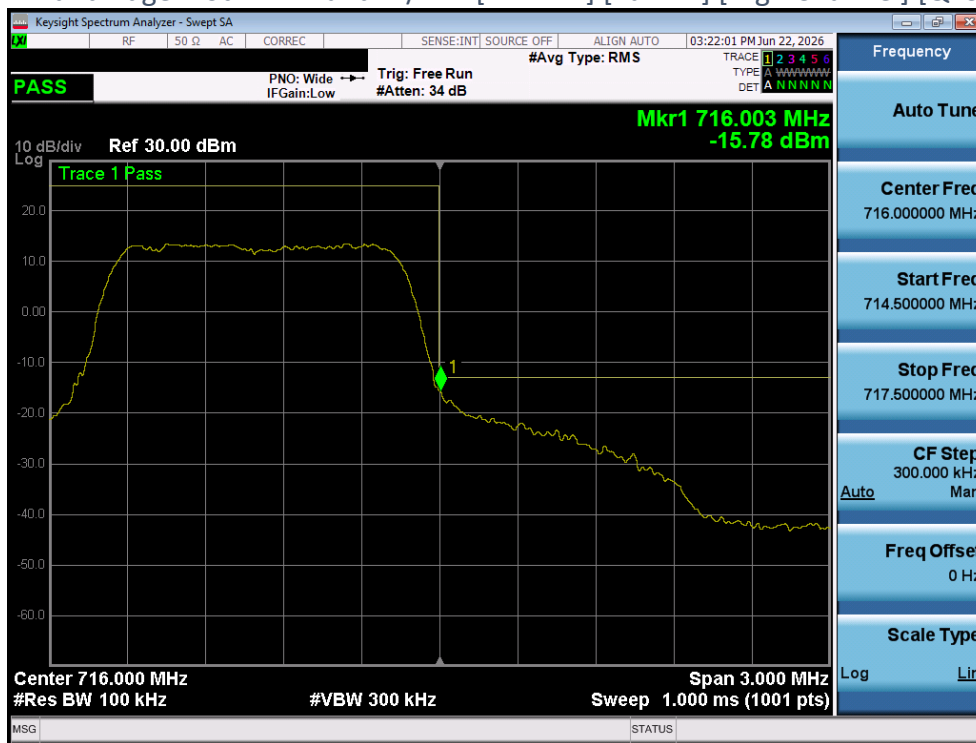
Plot 4-122 Band Edge Plot - LTE Band12/17 - [1.4MHz] [Full RB] [High Channel] [QPSK] [Ant 2]
