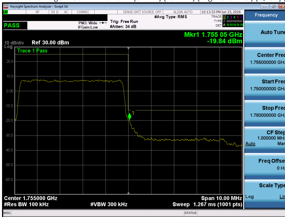
Plot 4-140 Band Edge Plot - LTE Band4 - [5MHz] [Full RB] [High Channel] [QPSK] [Ant 1]
