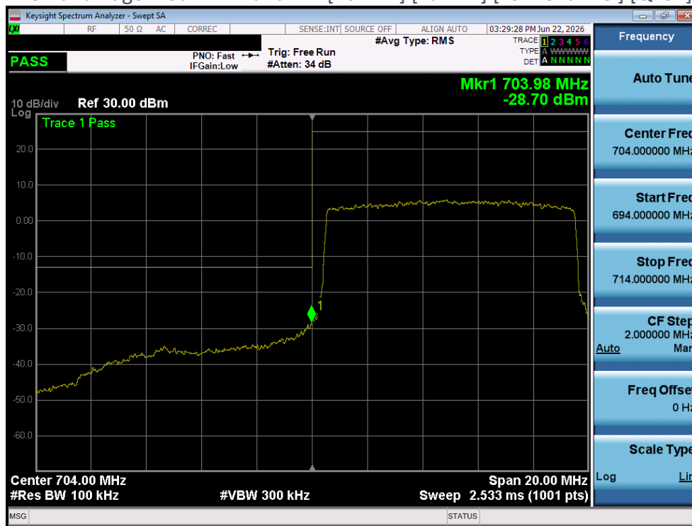
Plot 4-113 Band Edge Plot - LTE Band17 - [10MHz] [Full RB] [Low Channel] [QPSK] [Ant 1]
