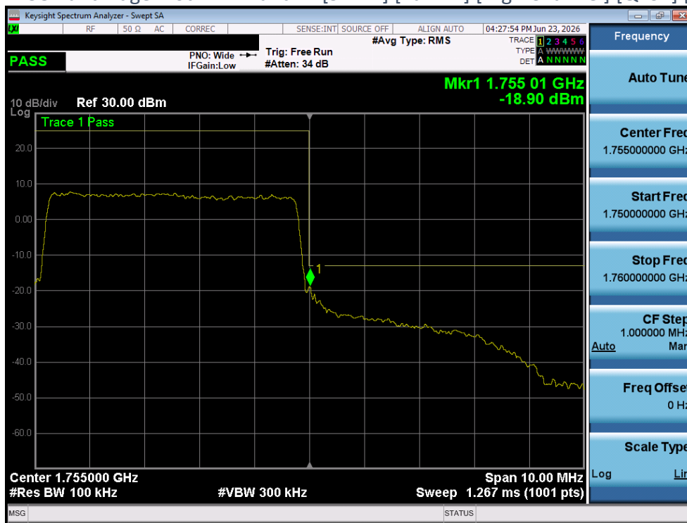
Plot 4-158 Band Edge Plot - LTE Band4 - [5MHz] [Full RB] [High Channel] [QPSK] [Ant 2]
