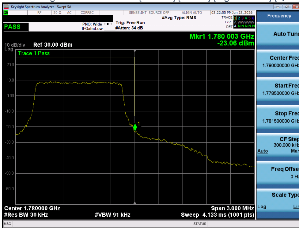
Plot 4-136 Band Edge Plot - LTE Band66 - [1.4MHz] [Full RB] [High Channel] [QPSK] [Ant 1]
