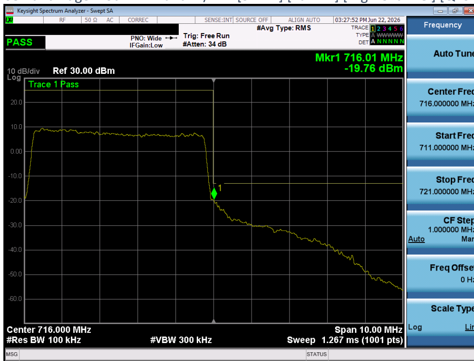
Plot 4-108 Band Edge Plot - LTE Band12/17 - [5MHz] [Full RB] [High Channel] [QPSK] [Ant 1]
