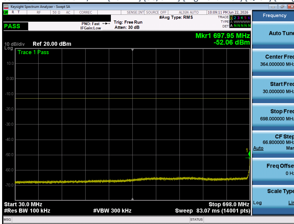
Plot 4-178 CSE Plot - LTE Band12/17 - [10MHz] [50/0 RB] [High Channel] [QPSK] [Range B] [Ant 1]
