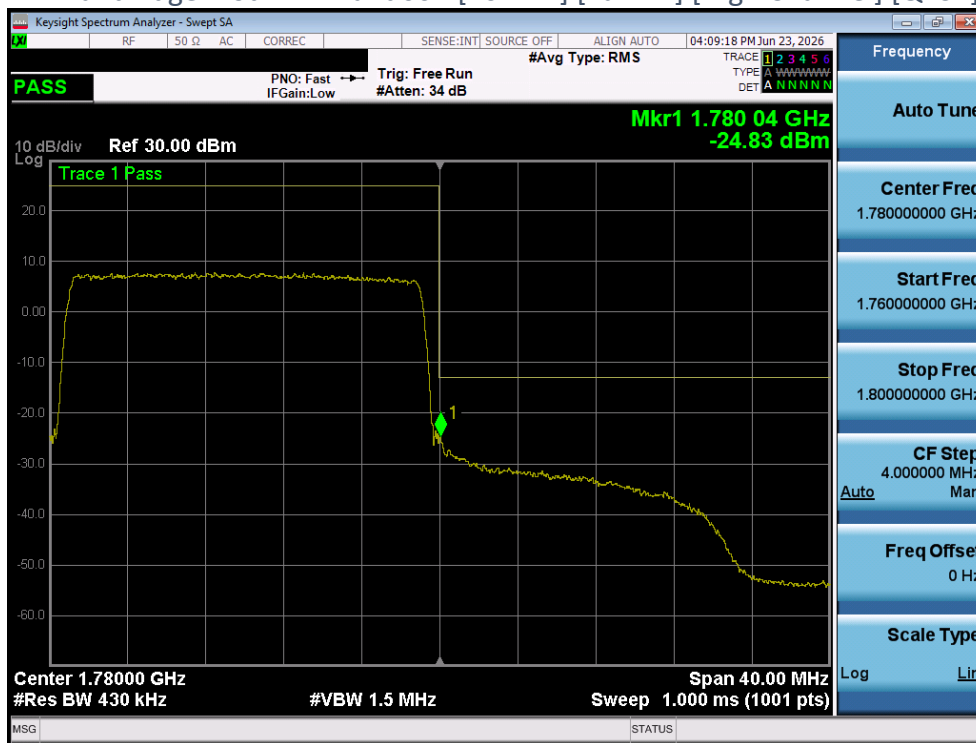
Plot 4-144 Band Edge Plot - LTE Band66 - [20MHz] [Full RB] [High Channel] [QPSK] [Ant 2]
