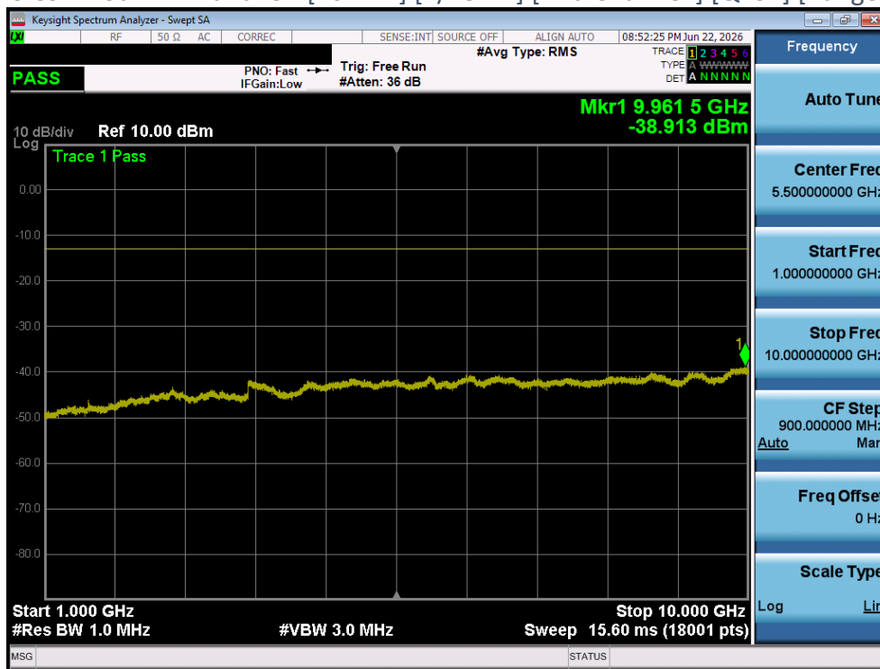
Plot 4-170 CSE Plot - LTE Band13 - [10MHz] [1/25 RB] [Mid Channel] [QPSK] [Range E] [Ant 2]
