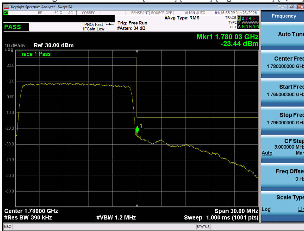
Plot 4-146 Band Edge Plot - LTE Band66 - [15MHz] [Full RB] [High Channel] [QPSK] [Ant 2]
