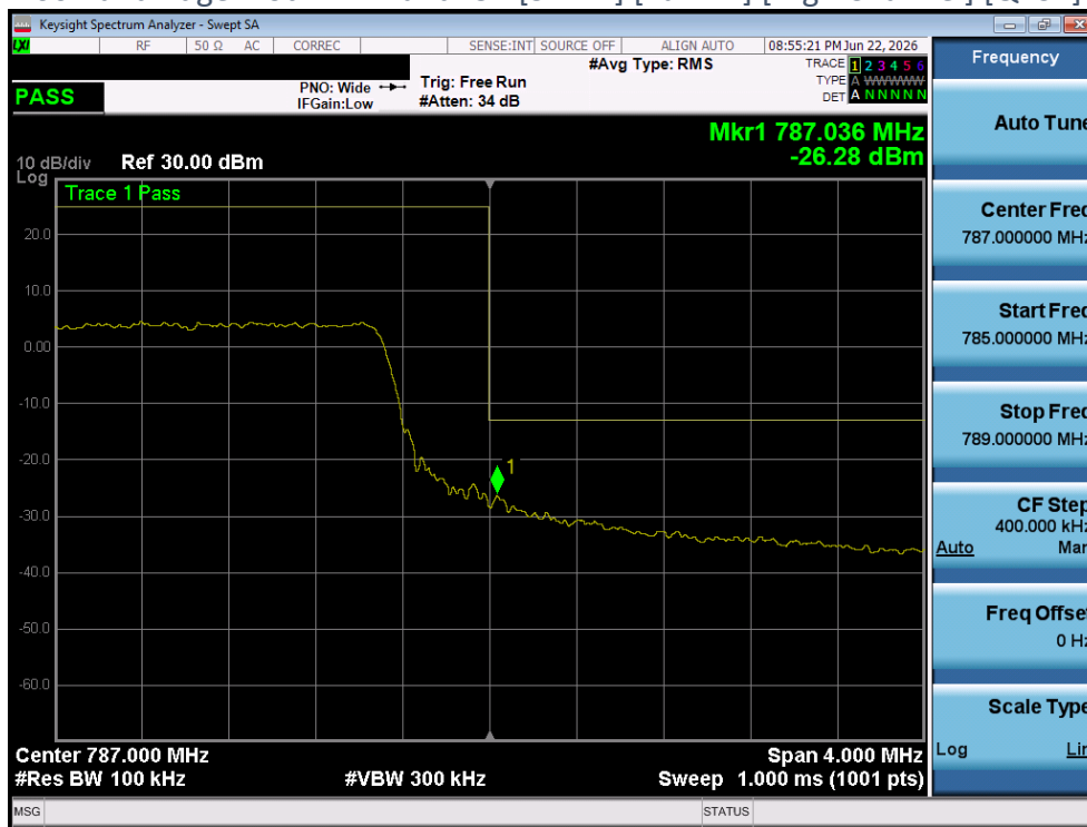
Plot 4-100 Band Edge Plot - LTE Band13 - [5MHz] [Full RB] [High Channel] [QPSK] [Ant 1]
