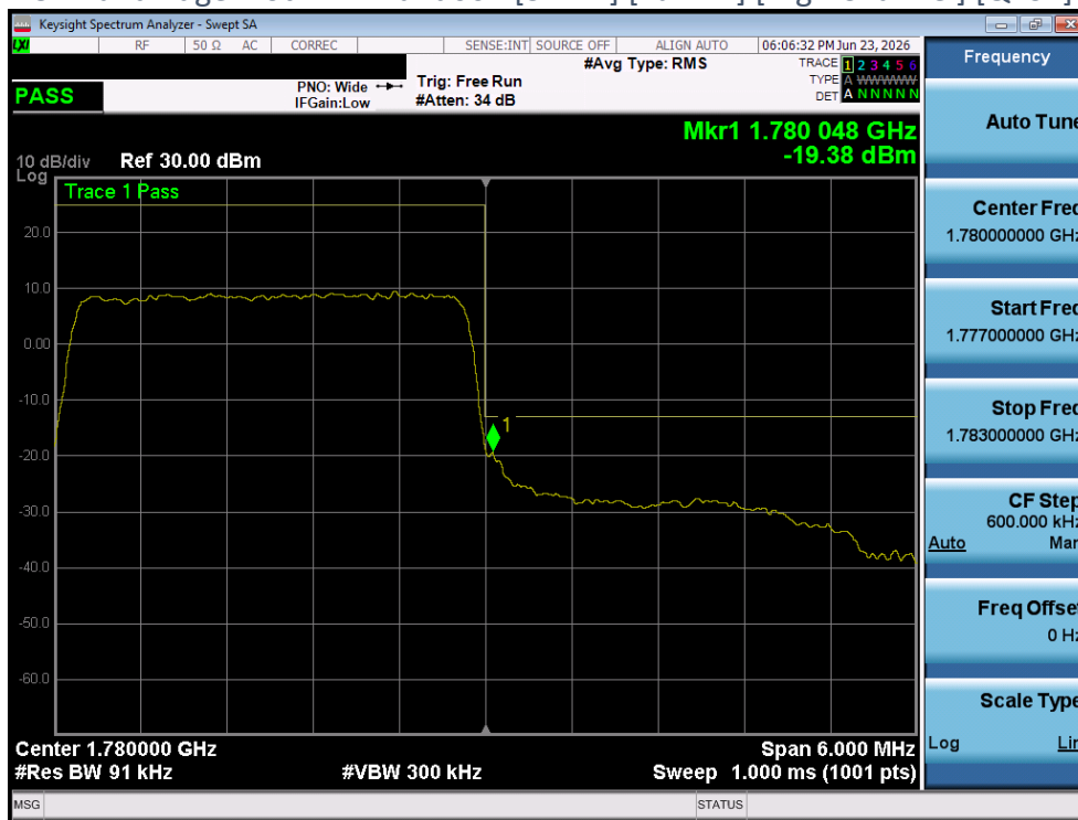
Plot 4-152 Band Edge Plot - LTE Band66 - [3MHz] [Full RB] [High Channel] [QPSK] [Ant 2]
