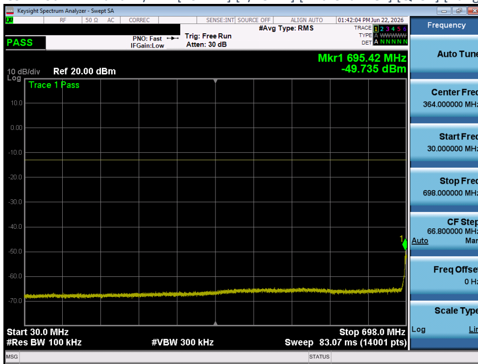
Plot 4-184 CSE Plot - LTE Band12/17 - [10MHz] [1/25 RB] [Mid Channel] [QPSK] [Range B] [Ant 2]
