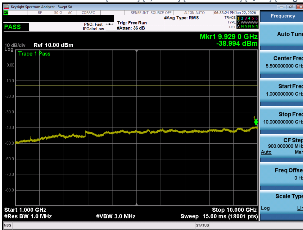
Plot 4-166 CSE Plot - LTE Band13 - [10MHz] [1/25 RB] [Mid Channel] [QPSK] [Range A] [Ant 2]
