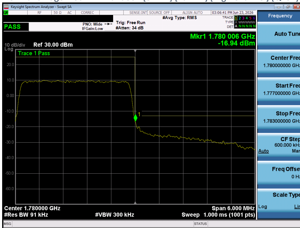
Plot 4-134 Band Edge Plot - LTE Band66 - [3MHz] [Full RB] [High Channel] [QPSK] [Ant 1]
