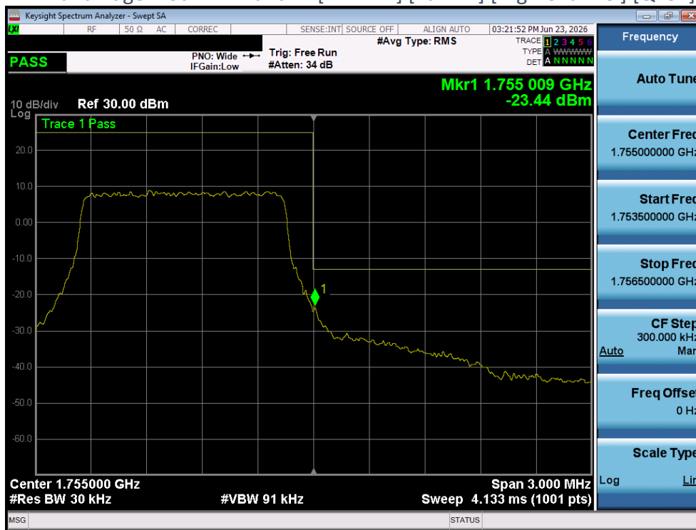
Plot 4-142 Band Edge Plot - LTE Band4 - [1.4MHz] [Full RB] [High Channel] [QPSK] [Ant 1]
