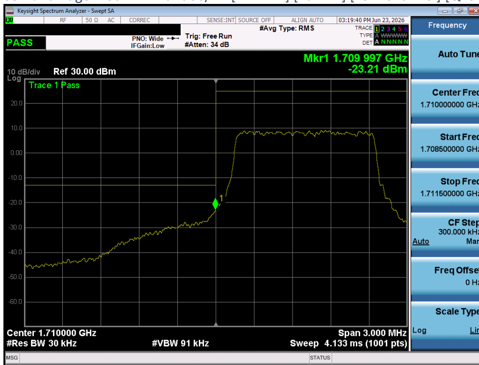
Plot 4-136 Band Edge Plot - LTE Band66 - [1.4MHz] [Full RB] [High Channel] [QPSK] [Ant 1]
