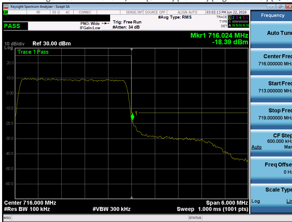
Plot 4-120 Band Edge Plot - LTE Band12/17 - [3MHz] [Full RB] [High Channel] [QPSK] [Ant 2]
