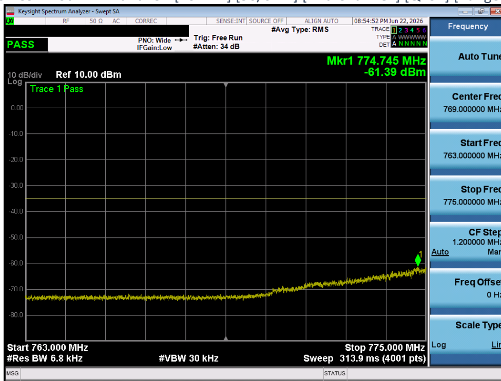
Plot 4-168 CSE Plot - LTE Band13 - [10MHz] [50/0 RB] [Mid Channel] [QPSK] [Range C] [Ant 2]
