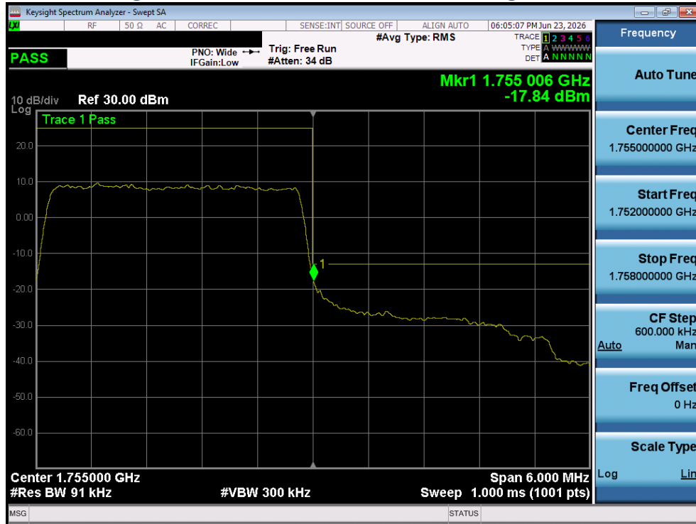
Plot 4-159 Band Edge Plot - LTE Band4 - [3MHz] [Full RB] [High Channel] [QPSK] [Ant 2]
