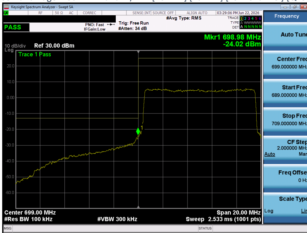
Plot 4-106 Band Edge Plot - LTE Band12/17 - [10MHz] [Full RB] [High Channel] [QPSK] [Ant 1]
