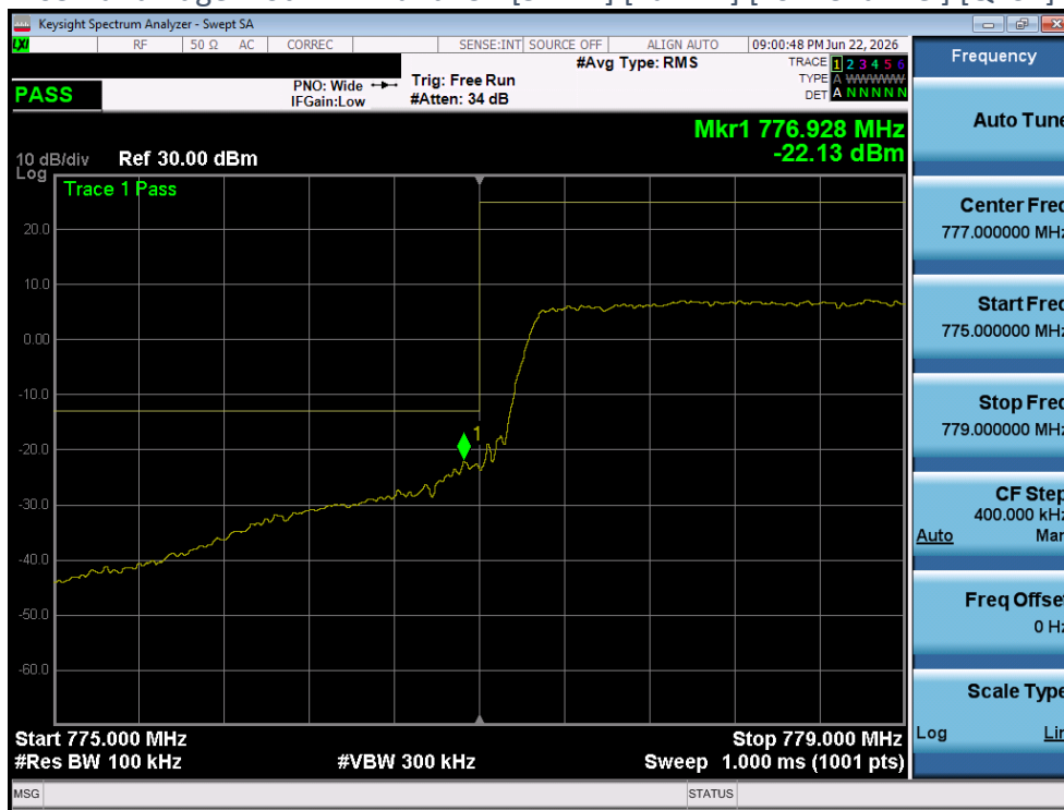
Plot 4-104 Band Edge Plot - LTE Band13 - [5MHz] [Full RB] [High Channel] [QPSK] [Ant 2]
