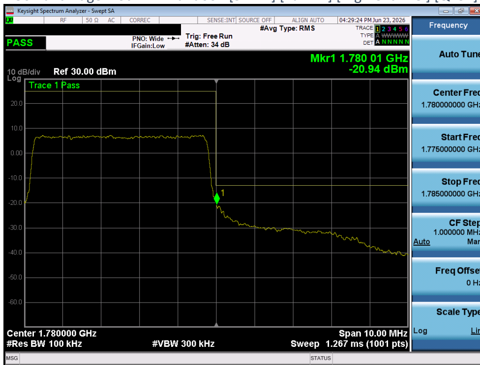
Plot 4-150 Band Edge Plot - LTE Band66 - [5MHz] [Full RB] [High Channel] [QPSK] [Ant 2]
