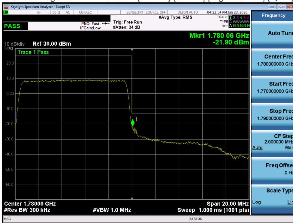
Plot 4-148 Band Edge Plot - LTE Band66 - [10MHz] [Full RB] [High Channel] [QPSK] [Ant 2]
