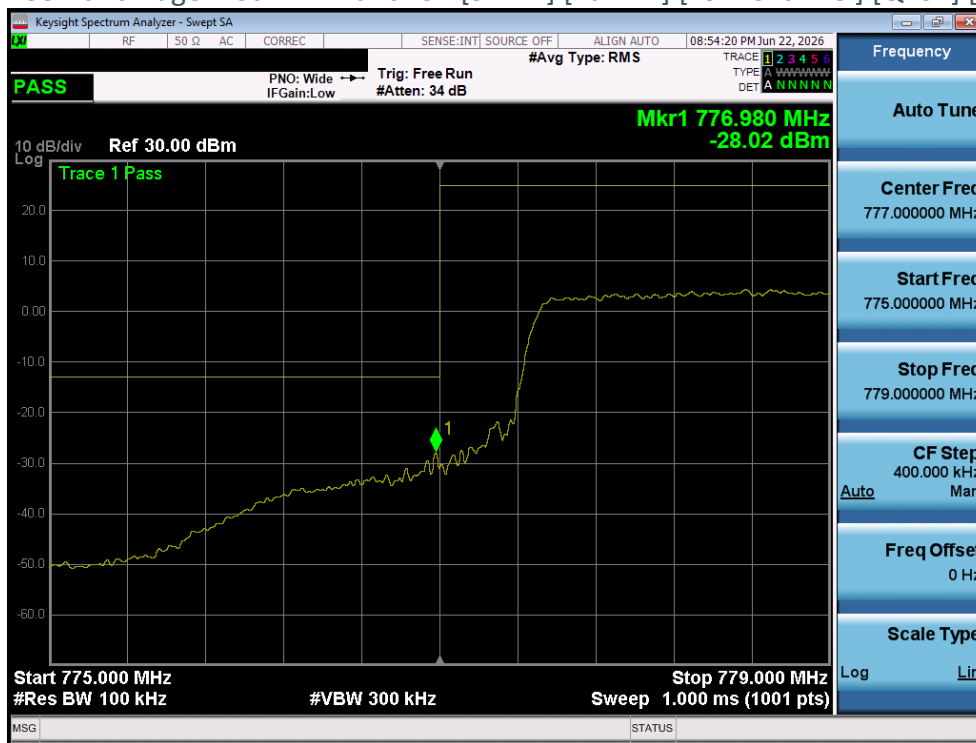
Plot 4-100 Band Edge Plot - LTE Band13 - [5MHz] [Full RB] [High Channel] [QPSK] [Ant 1]
