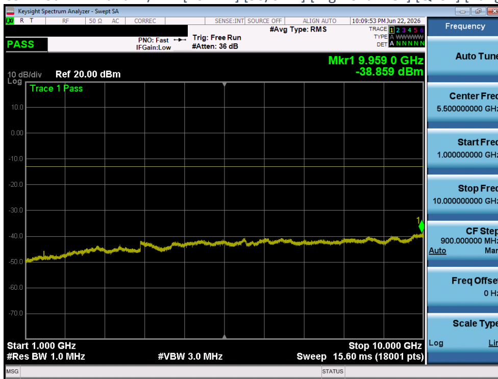
Plot 4-180 CSE Plot - LTE Band12/17 - [10MHz] [50/0 RB] [Low Channel] [QPSK] [Range A] [Ant 2]
