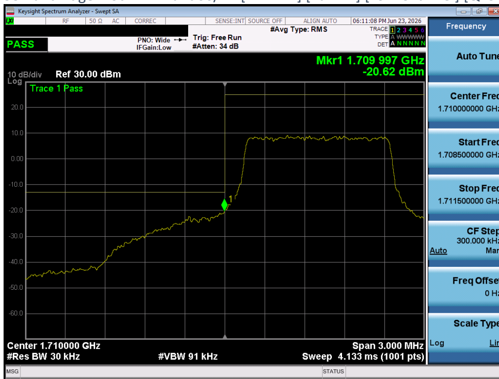
Plot 4-154 Band Edge Plot - LTE Band66 - [1.4MHz] [Full RB] [High Channel] [QPSK] [Ant 2]
