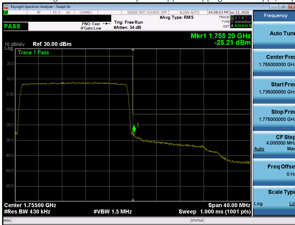
Plot 4-156 Band Edge Plot - LTE Band4 - [15MHz] [Full RB] [High Channel] [QPSK] [Ant 2]
