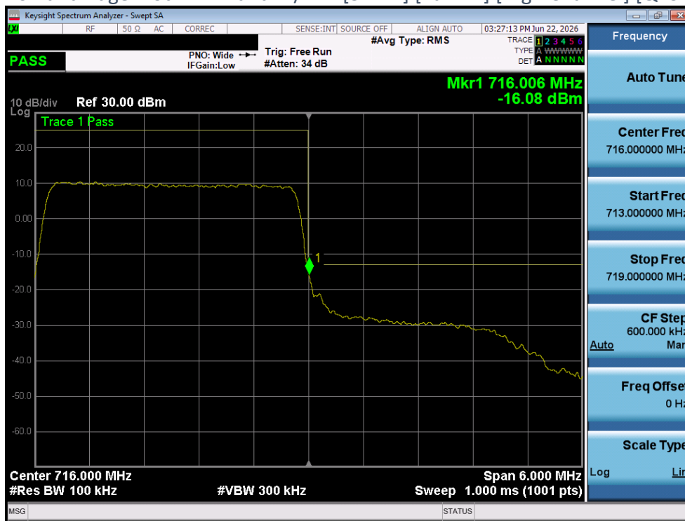
Plot 4-110 Band Edge Plot - LTE Band12/17 - [3MHz] [Full RB] [High Channel] [QPSK] [Ant 1]
