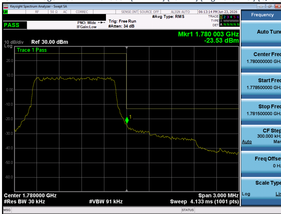
Plot 4-154 Band Edge Plot - LTE Band66 - [1.4MHz] [Full RB] [High Channel] [QPSK] [Ant 2]
