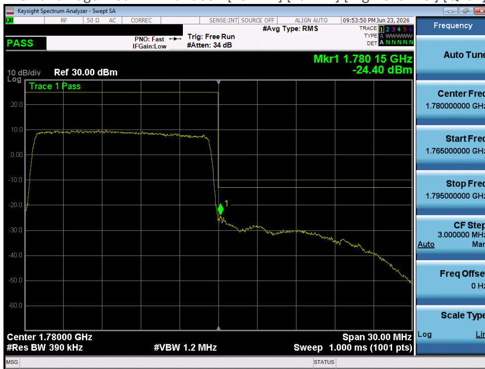
Plot 4-128 Band Edge Plot - LTE Band66 - [15MHz] [Full RB] [High Channel] [QPSK] [Ant 1]
