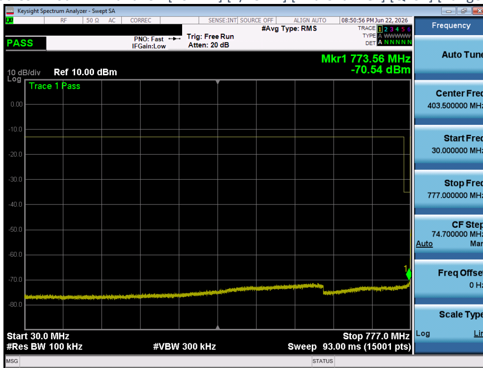
Plot 4-166 CSE Plot - LTE Band13 - [10MHz] [1/25 RB] [Mid Channel] [QPSK] [Range A] [Ant 2]
