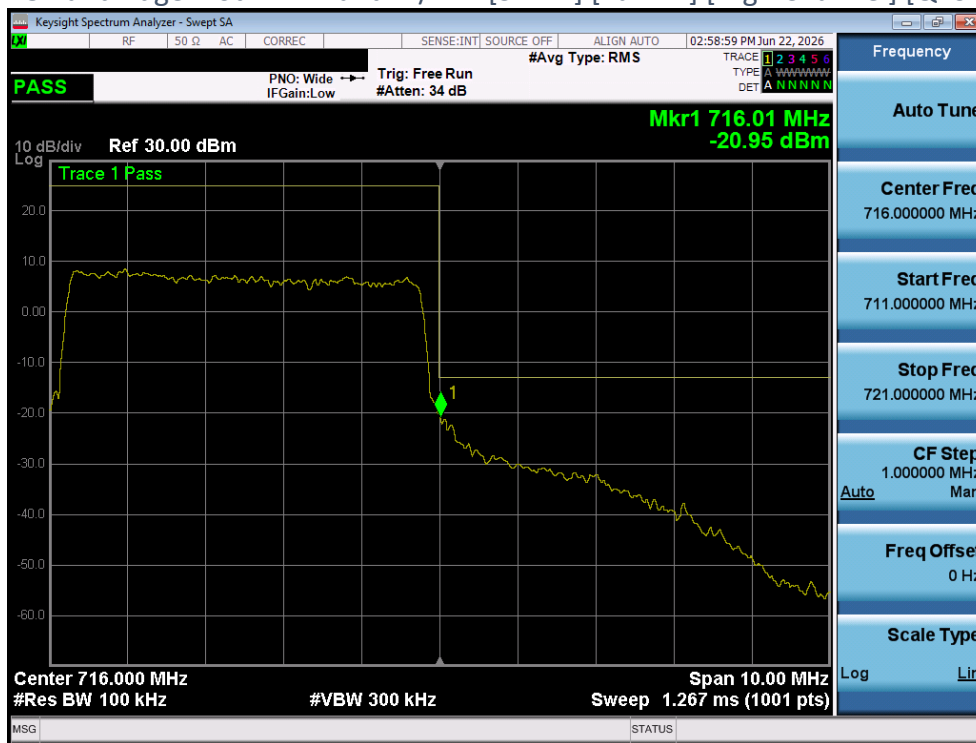
Plot 4-118 Band Edge Plot - LTE Band12/17 - [5MHz] [Full RB] [High Channel] [QPSK] [Ant 2]
