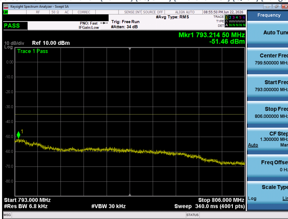
Plot 4-168 CSE Plot - LTE Band13 - [10MHz] [50/0 RB] [Mid Channel] [QPSK] [Range C] [Ant 2]
