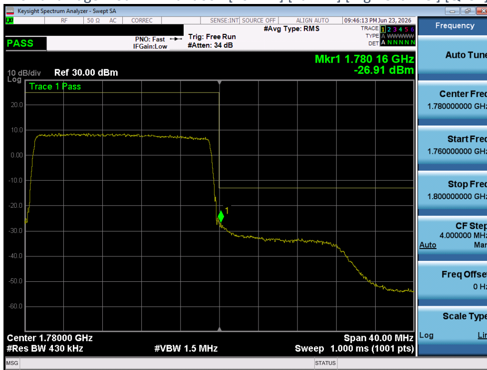
Plot 4-126 Band Edge Plot - LTE Band66 - [20MHz] [Full RB] [High Channel] [QPSK] [Ant 1]
