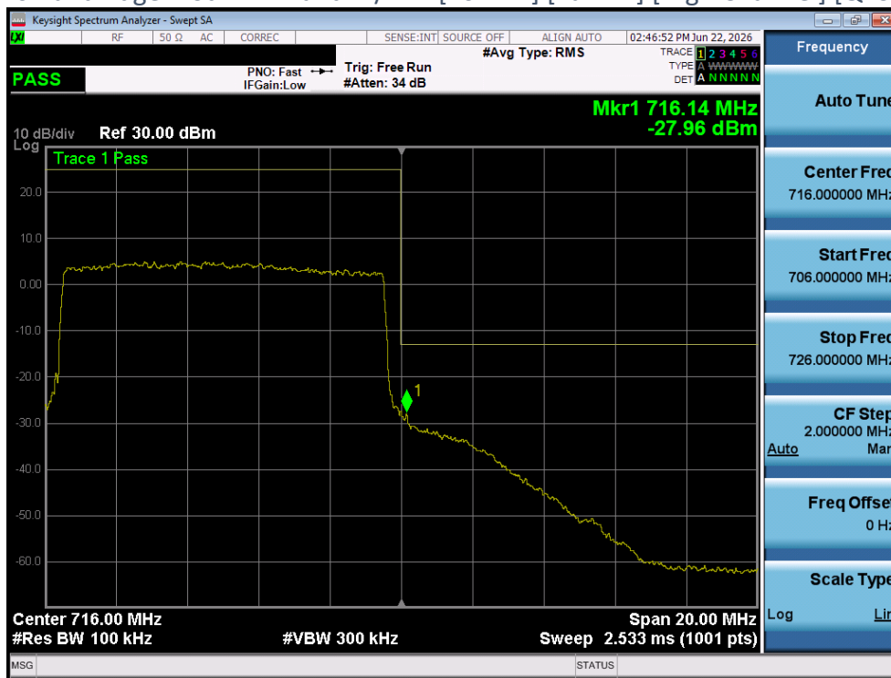
Plot 4-116 Band Edge Plot - LTE Band12/17 - [10MHz] [Full RB] [High Channel] [QPSK] [Ant 2]
