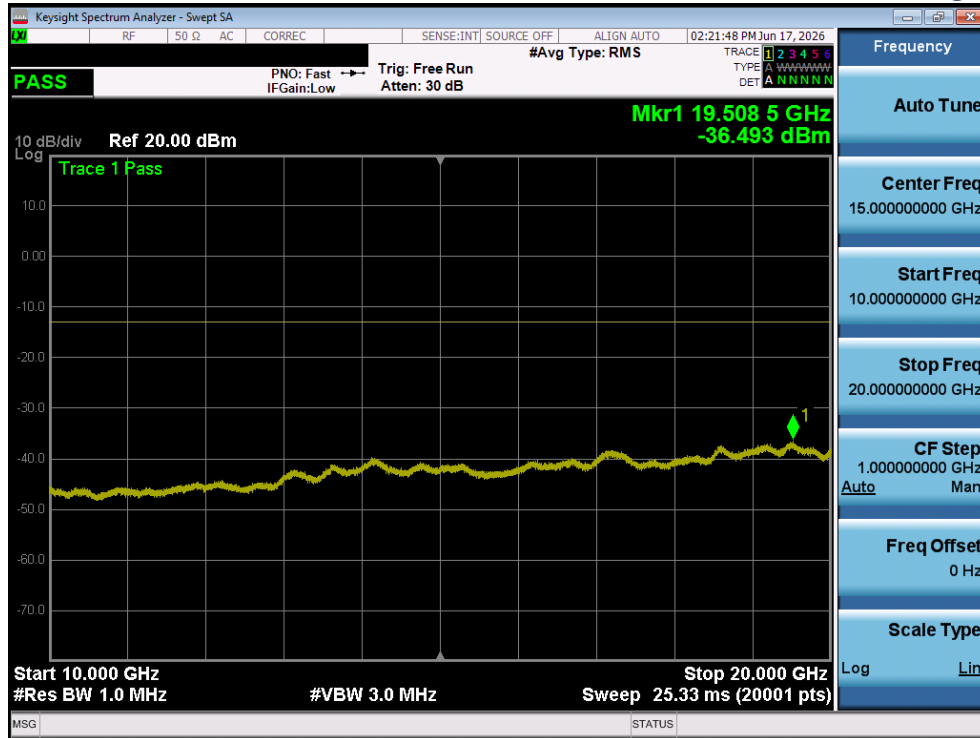
Plot 4-99 CSE Plot - LTE Band25/2 - [20MHz] [1/50 RB] [Mid Channel] [QPSK] [Range C] [Ant 2]
