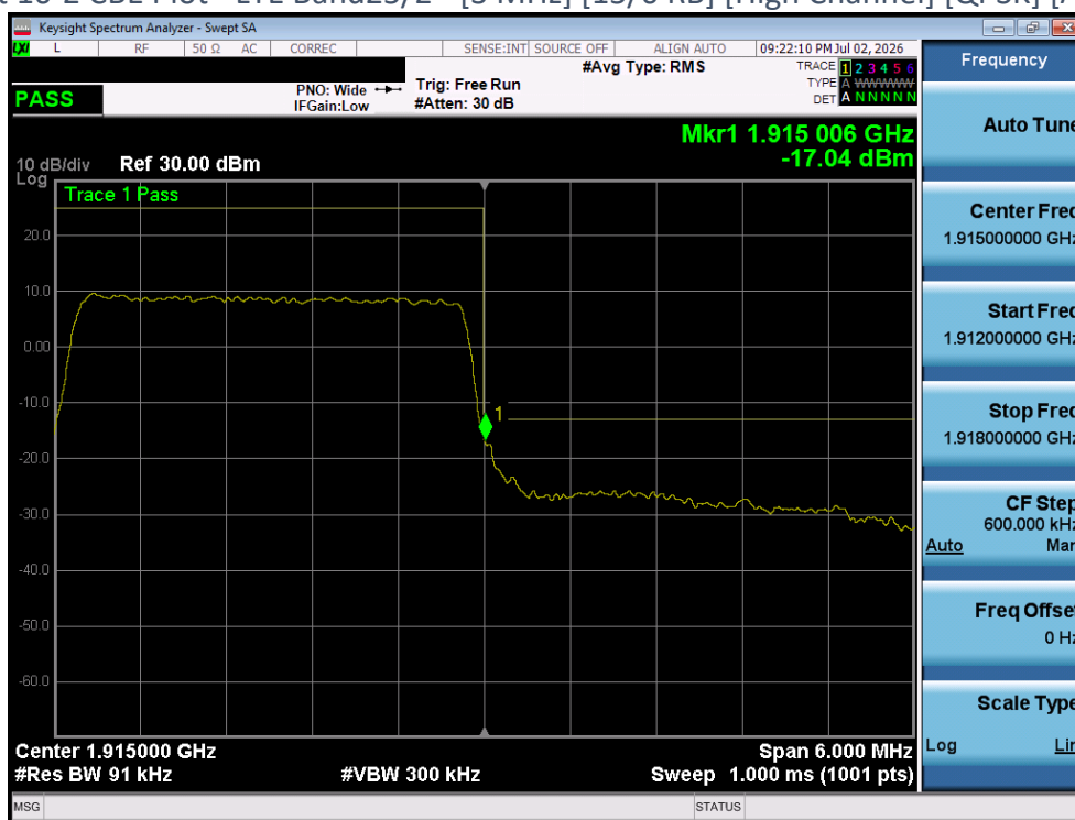
Plot 10-2 CBE Plot - LTE Band25/2 - [3 MHz] [15/0 RB] [High Channel] [QPSK] [Ant 1]
