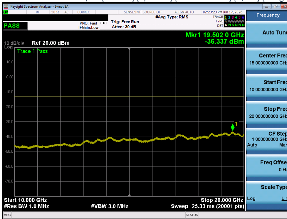
Plot 4-96 CSE Plot - LTE Band25/2 - [20MHz] [1/50 RB] [Low Channel] [QPSK] [Range C] [Ant 2]
