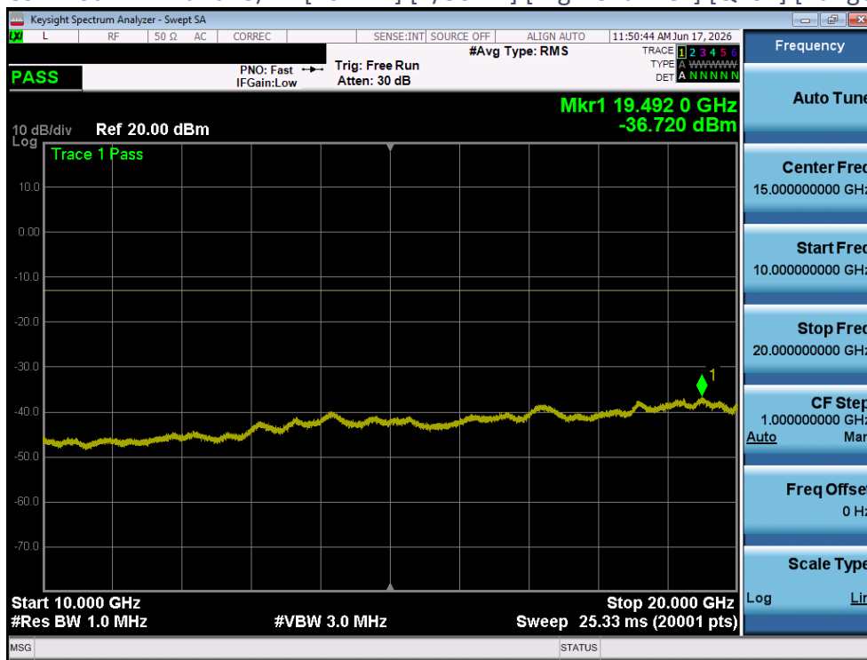
Plot 4-94 CSE Plot - LTE Band25/2 - [20MHz] [1/50 RB] [Low Channel] [QPSK] [Range A] [Ant 2]
