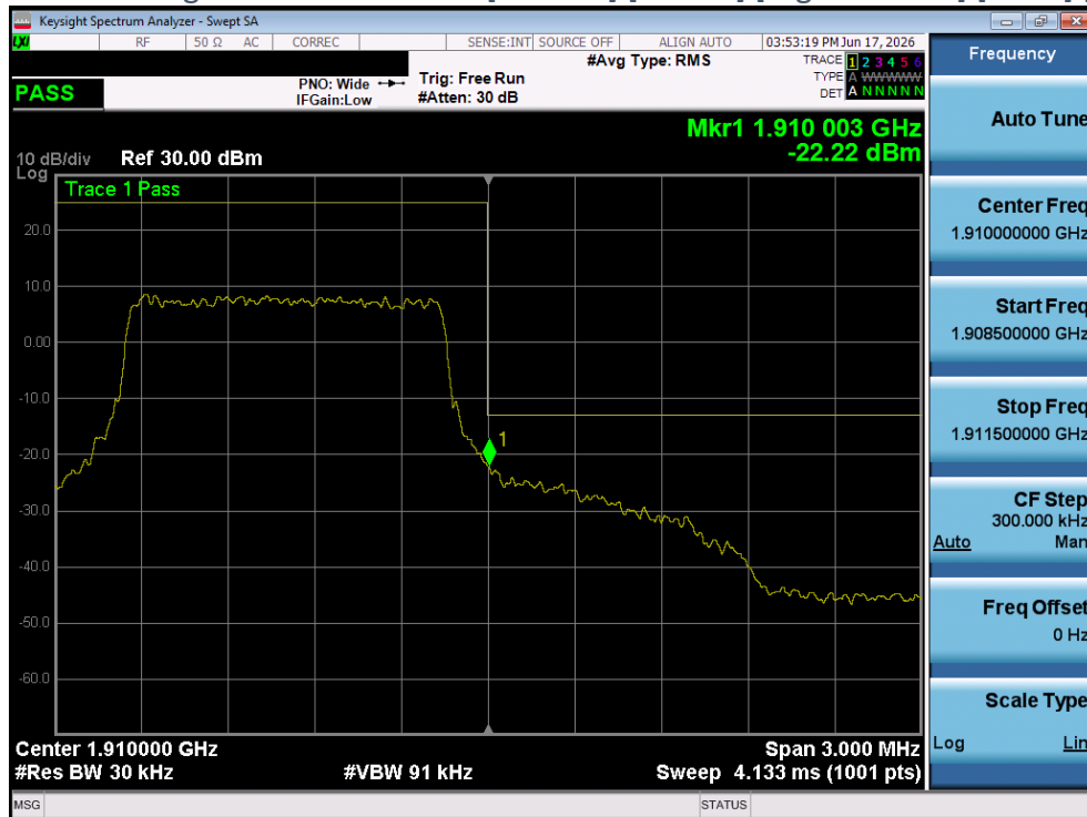
Plot 4-84 Band Edge Plot - LTE Band2 - [1.4MHz] [Full RB] [High Channel] [QPSK] [Ant 2]
