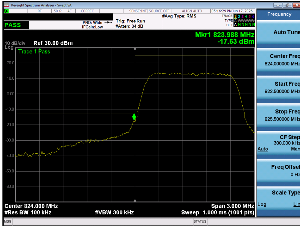
Plot 4-59 Band Edge Plot - LTE Band26/5 - [1.4MHz] [Full RB] [Low Channel] [QPSK] [Ant 2]
