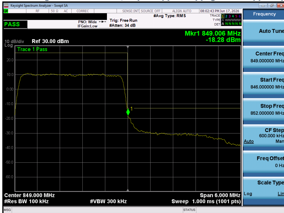
Plot 4-48 Band Edge Plot - LTE Band26/5 - [3MHz] [Full RB] [High Channel] [QPSK] [Ant 1]
