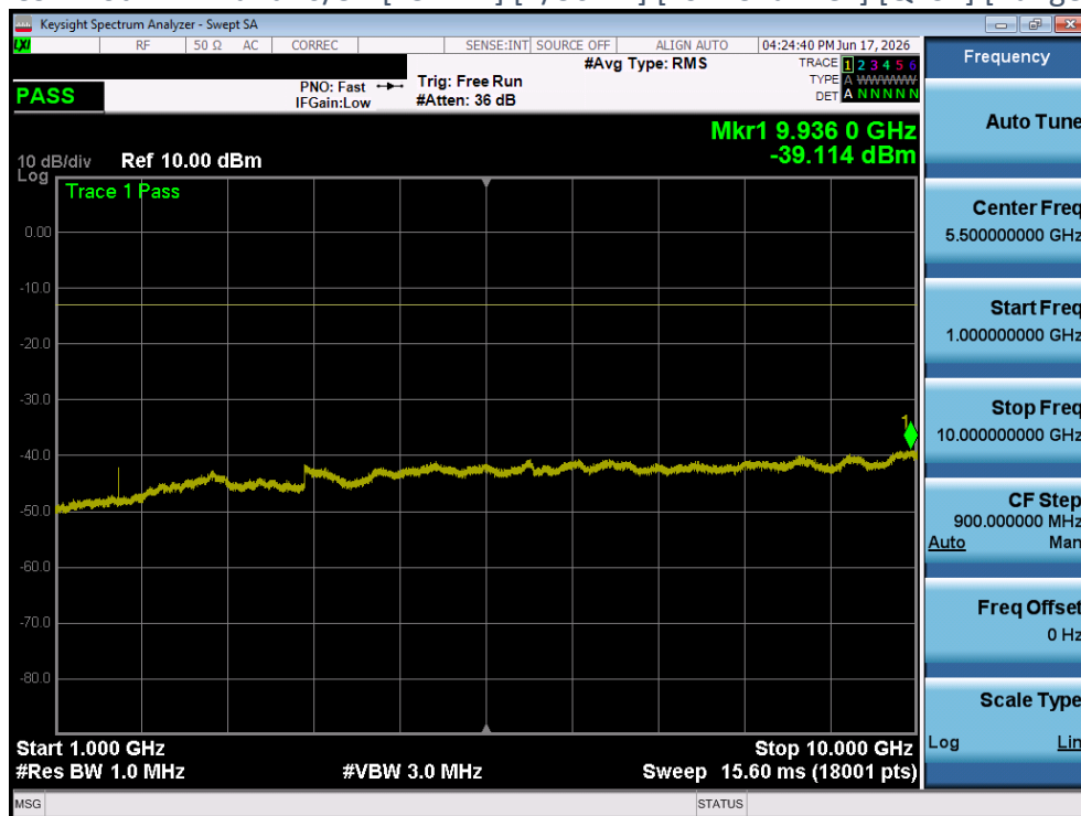
Plot 4-72 CSE Plot - LTE Band26/5 - [15MHz] [1/36 RB] [Low Channel] [QPSK] [Range C] [Ant 2]
