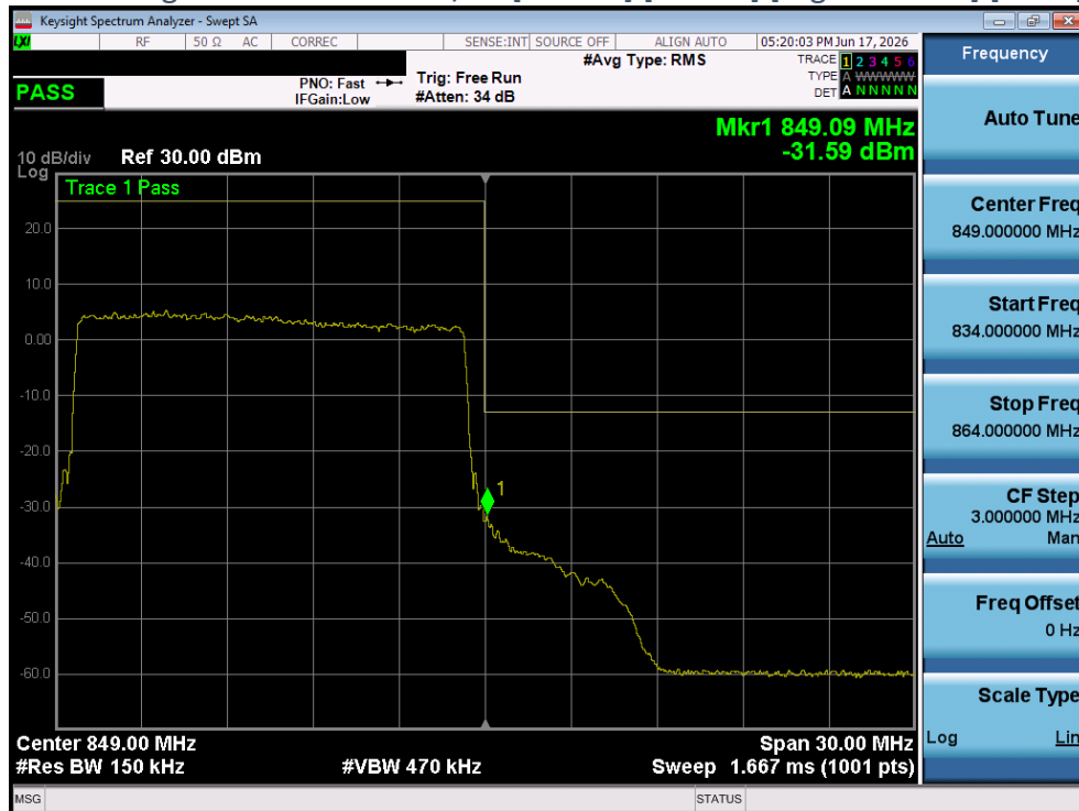
Plot 4-52 Band Edge Plot - LTE Band26/5 - [15MHz] [Full RB] [High Channel] [QPSK] [Ant 2]
