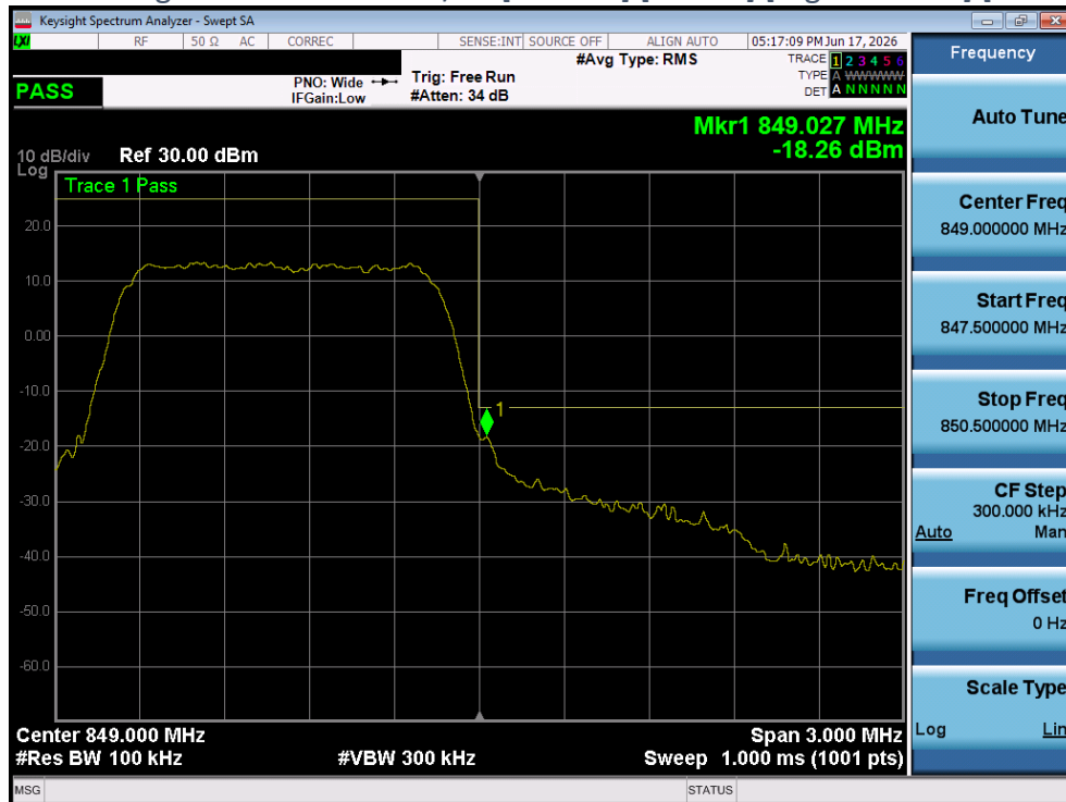
Plot 4-60 Band Edge Plot - LTE Band26/5 - [1.4MHz] [Full RB] [High Channel] [QPSK] [Ant 2]
