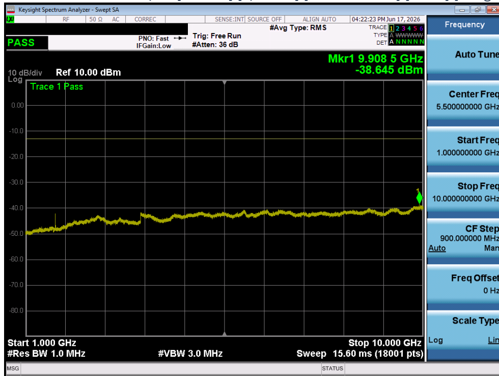
Plot 4-76 CSE Plot - LTE Band26/5 - [15MHz] [1/36 RB] [High Channel] [QPSK] [Range A] [Ant 2]
