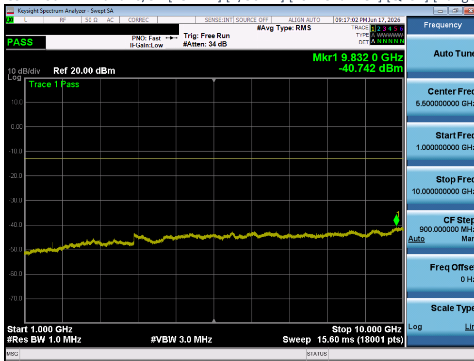
Plot 4-64 CSE Plot - LTE Band26/5 - [15MHz] [1/36 RB] [Mid Channel] [QPSK] [Range A] [Ant 1]
