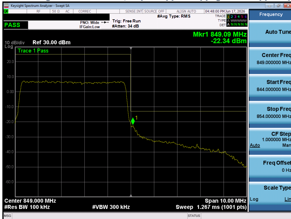
Plot 4-56 Band Edge Plot - LTE Band26/5 - [5MHz] [Full RB] [High Channel] [QPSK] [Ant 2]
