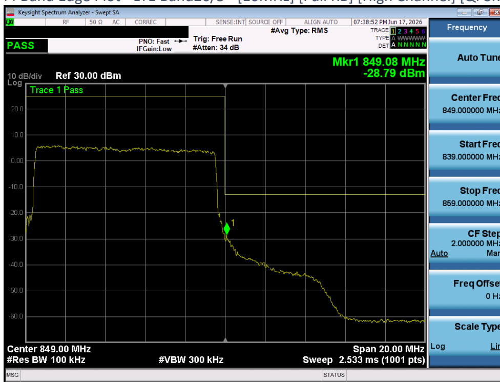
Plot 4-44 Band Edge Plot - LTE Band26/5 - [10MHz] [Full RB] [High Channel] [QPSK] [Ant 1]
