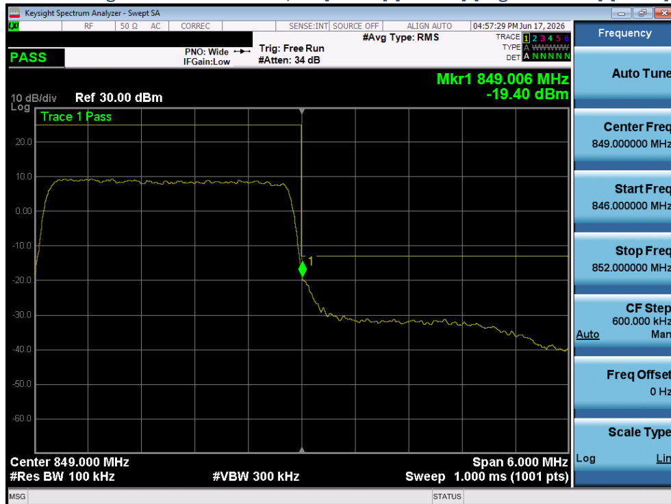
Plot 4-58 Band Edge Plot - LTE Band26/5 - [3MHz] [Full RB] [High Channel] [QPSK] [Ant 2]
