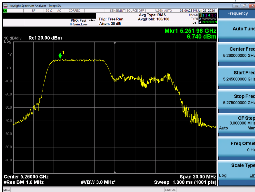
Plot 5-38 802.11ax20 CH.52 OFDMA MIMO 106Tone Maximum PSD - (Ant 2)
