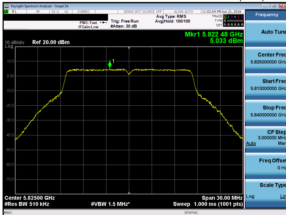
Plot 5-24 802.11a CH.165 OFDM MIMO Maximum PSD – (ANT2)
