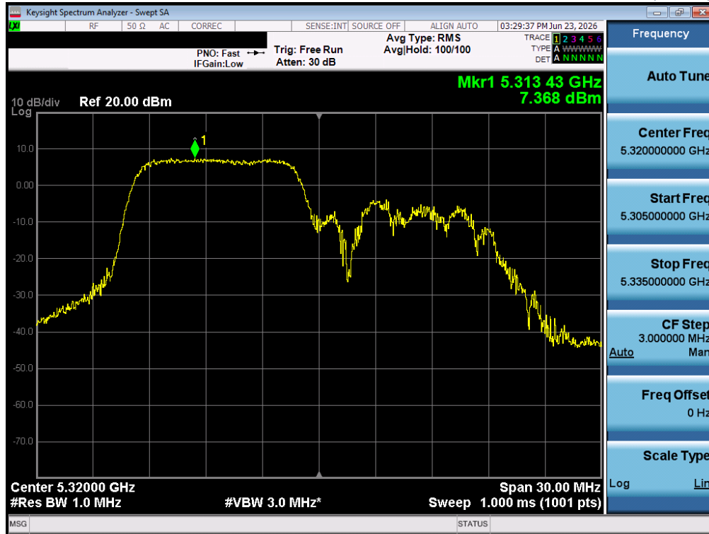
Plot 5-42 802.11ax20 CH.64 OFDMA MIMO 106Tone Maximum PSD - (Ant 2)
