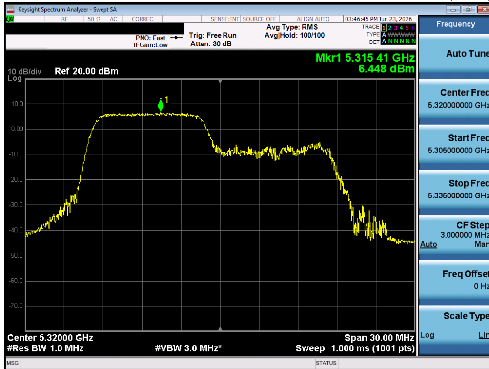
Plot 5-42 802.11ax20 CH.64 OFDMA MIMO 106Tone Maximum PSD - (Ant 2)
