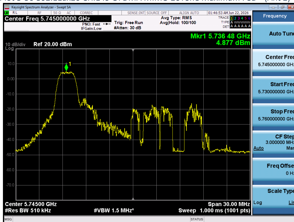
Plot 5-50 802.11ax20 CH.149 OFDMA MIMO 26Tone Maximum PSD - (Ant 2)
