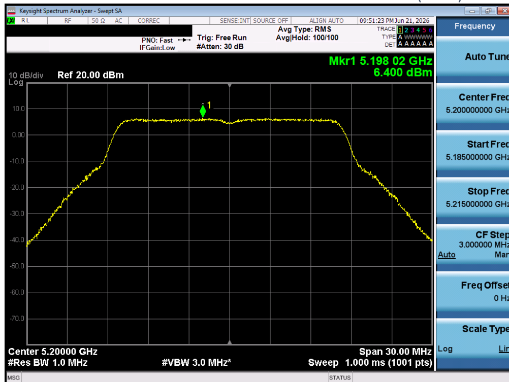
Plot 5-4 802.11a CH.40 OFDM MIMO Maximum PSD – (ANT2)
