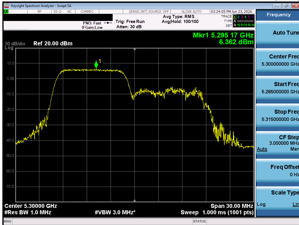
Plot 5-40 802.11ax20 CH.60 OFDMA MIMO 106Tone Maximum PSD - (Ant 2)
