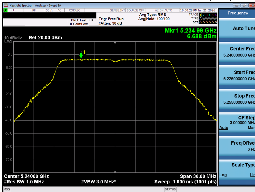
Plot 5-6 802.11a CH.48 OFDM MIMO Maximum PSD – (ANT2)
