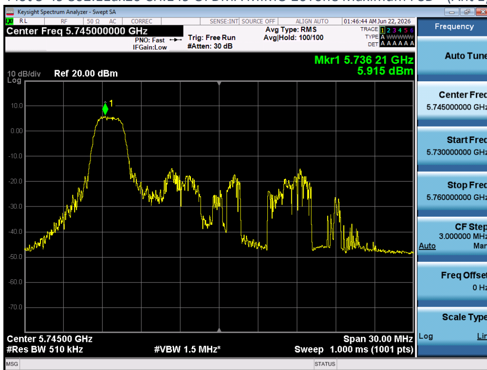
Plot 5-49 802.11ax20 CH.149 OFDMA MIMO 26Tone Maximum PSD - (Ant 1)
