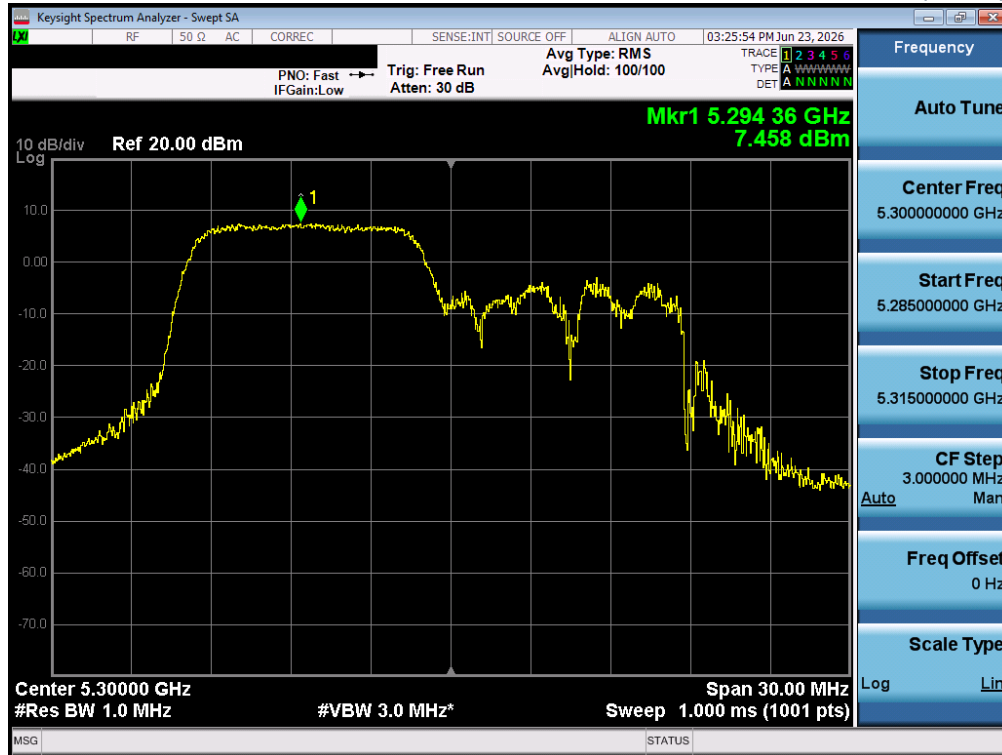
Plot 5-40 802.11ax20 CH.60 OFDMA MIMO 106Tone Maximum PSD - (Ant 2)
