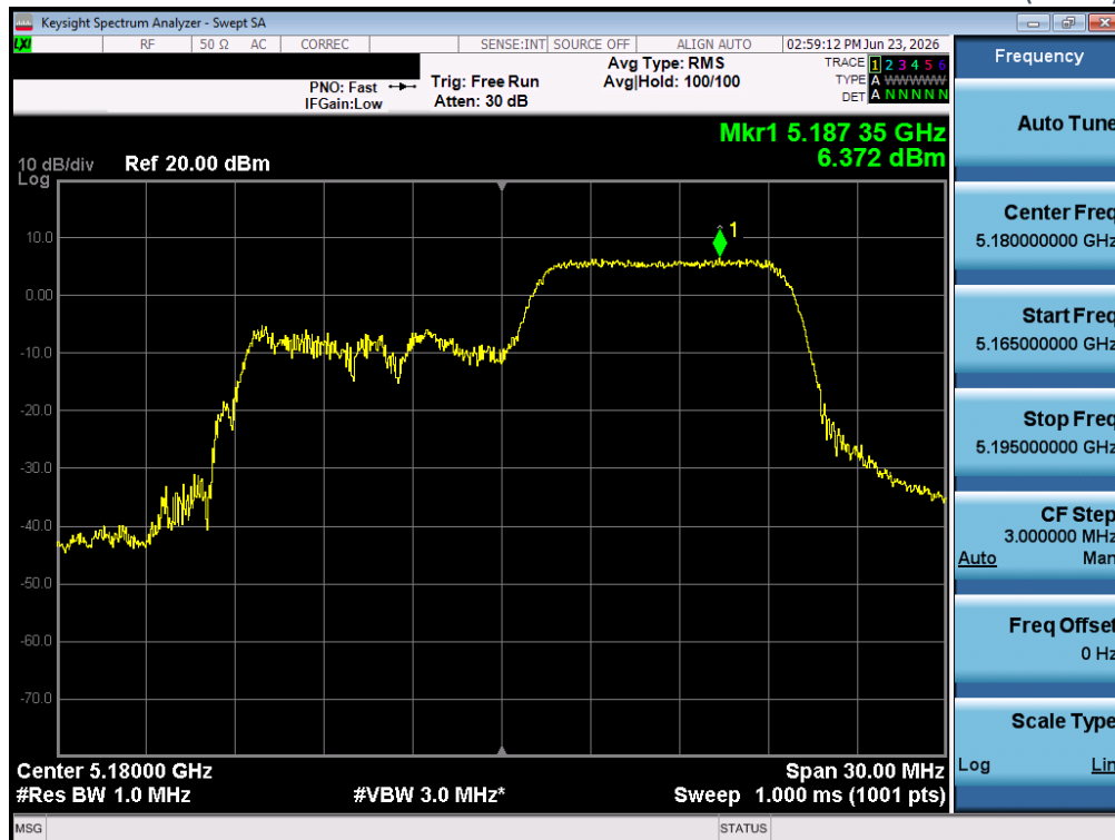
Plot 5-32 802.11ax20 CH.36 OFDMA MIMO 106Tone Maximum PSD - (Ant 2)
