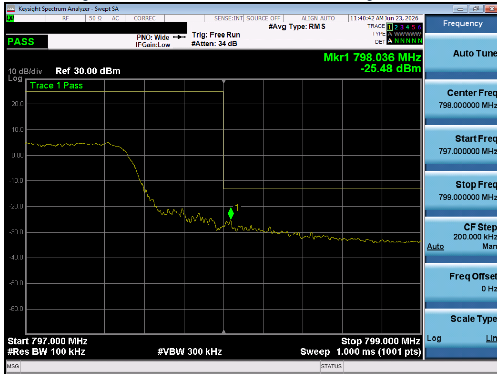
Plot 4-52 Band Edge Plot - LTE Band14 - [10MHz] [Full RB] [High Channel] [QPSK] [Ant 1]
