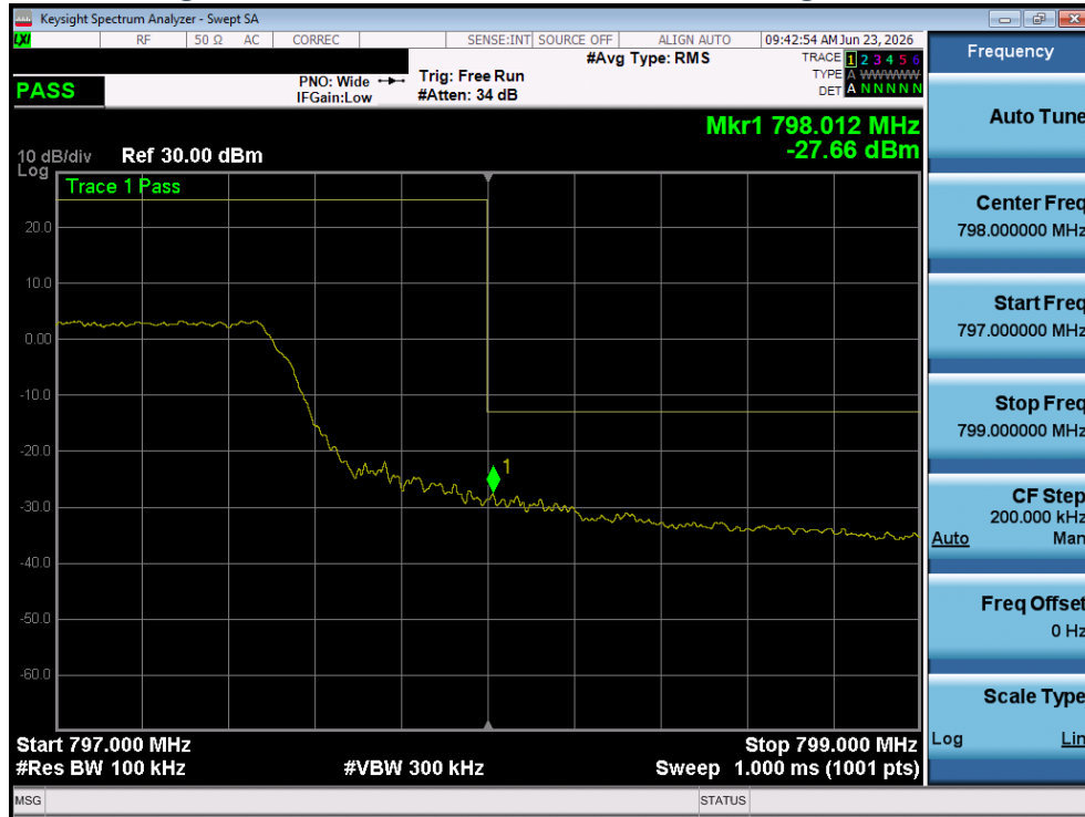
Plot 4-56 Band Edge Plot - LTE Band14 - [10MHz] [Full RB] [High Channel] [QPSK] [Ant 2]
