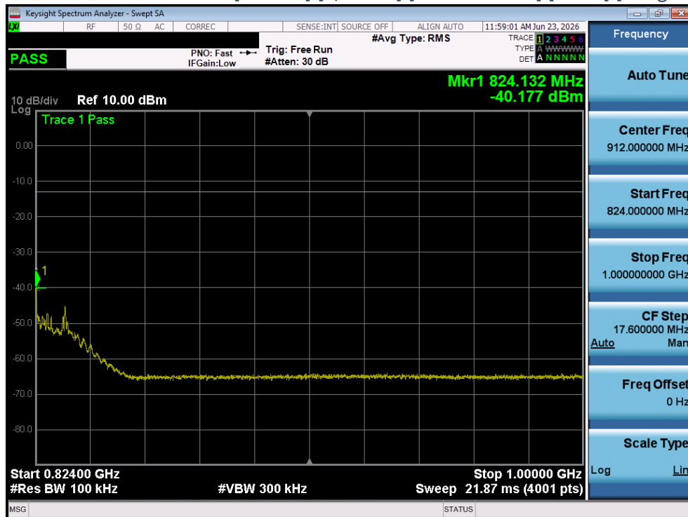
Plot 4-60 CSE Plot - LTE Band26 - [15MHz] [1/36 RB] [Mid Channel] [QPSK] [Range B] [Ant 1]
