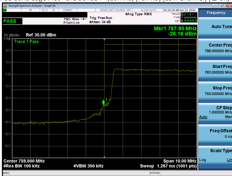
Plot 4-55 Band Edge Plot - LTE Band14 - [10MHz] [Full RB] [Low Channel] [QPSK] [Ant 2]
