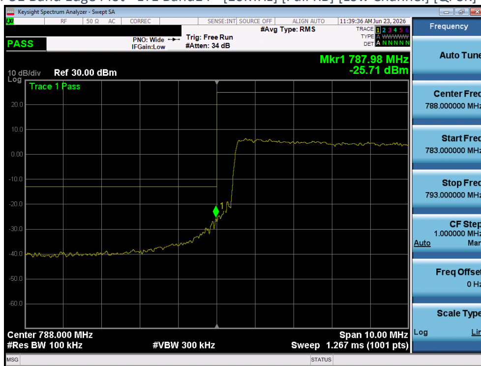
Plot 4-51 Band Edge Plot - LTE Band14 - [10MHz] [Full RB] [Low Channel] [QPSK] [Ant 1]
