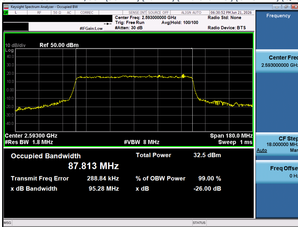
Plot 4-110 OBW Plot - NR n41/38 - [90MHz] [Full RB] [Mid Channel] [CP OFDM] [QPSK] [Ant 2]
