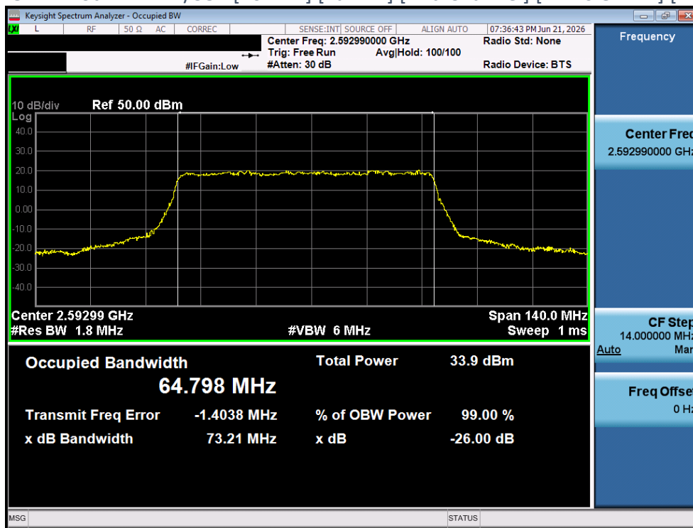
Plot 4-120 OBW Plot - NR n41/38 - [70MHz] [Full RB] [Mid Channel] [DFT-s OFDM] [BPSK] [Ant 2]
