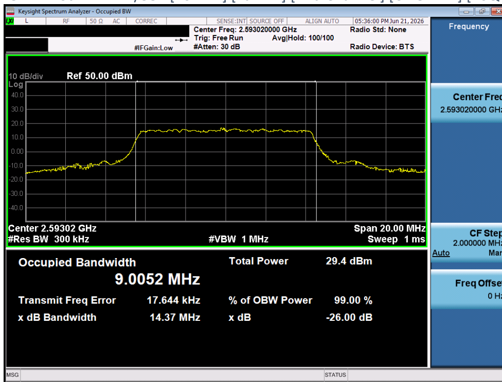
Plot 4-172 OBW Plot - NR n41/38 - [10MHz] [Full RB] [Mid Channel] [CP OFDM] [16QAM] [Ant 2]
