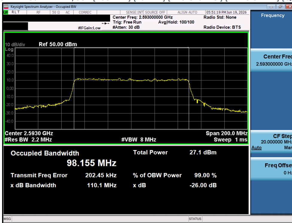
Plot 4-188 OBW Plot - NR n41/38 - [100MHz] [Full RB] [Mid Channel] [DFT-s OFDM] [QPSK] [SRS S3]
