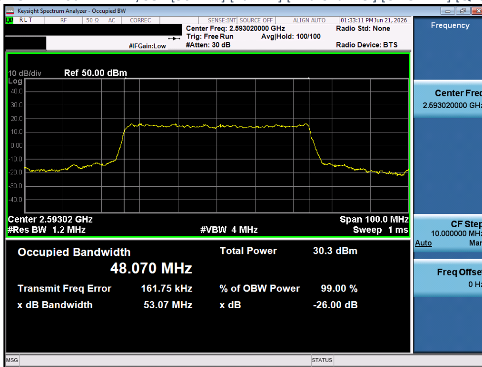
Plot 4-134 OBW Plot - NR n41/38 - [50MHz] [Full RB] [Mid Channel] [CP OFDM] [QPSK] [Ant 2]
