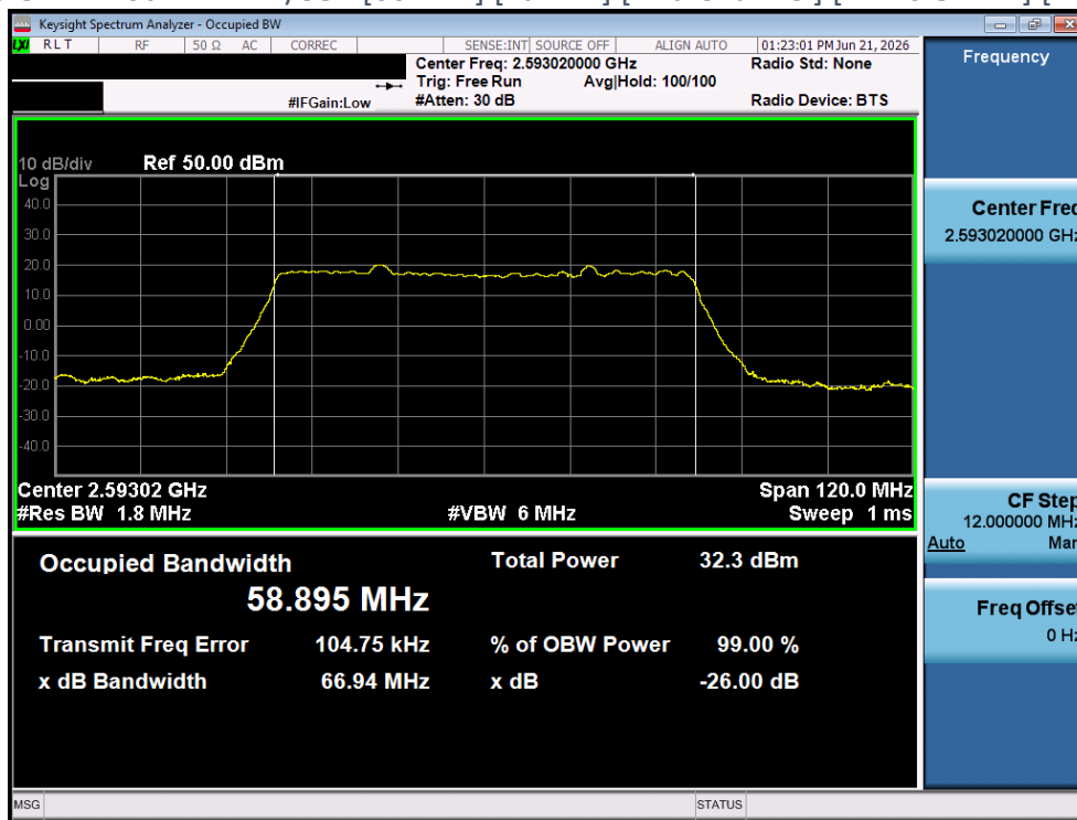
Plot 4-126 OBW Plot - NR n41/38 - [60MHz] [Full RB] [Mid Channel] [DFT-s OFDM] [BPSK] [Ant 2]
