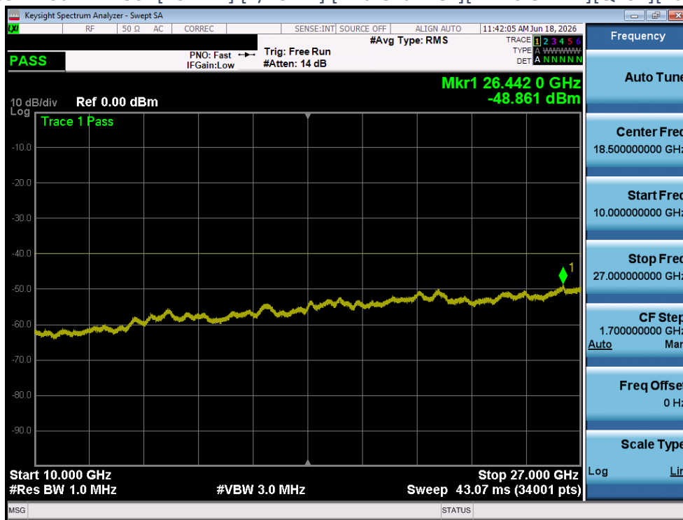
Plot 4-350 CSE Plot -NR n30- [10MHz] [1/25 RB] [Mid Channel ][DFT-s OFDM][QPSK][Range C][Ant 2]
