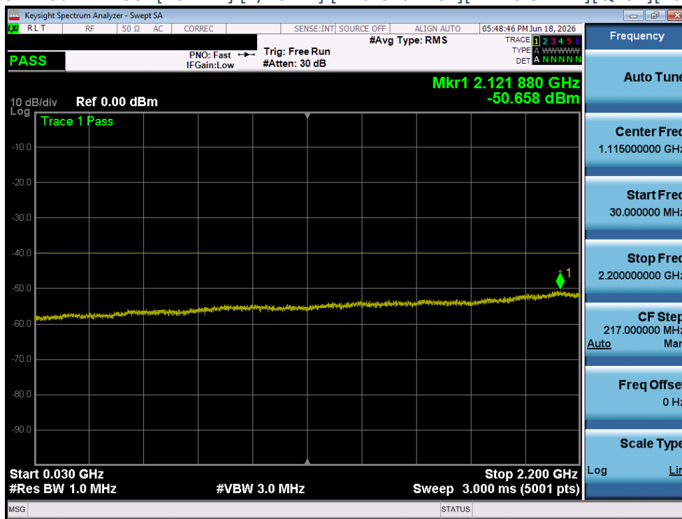
Plot 4-348 CSE Plot -NR n30- [10MHz] [1/25 RB] [Mid Channel ][DFT-s OFDM][QPSK][Range A][Ant 2]
