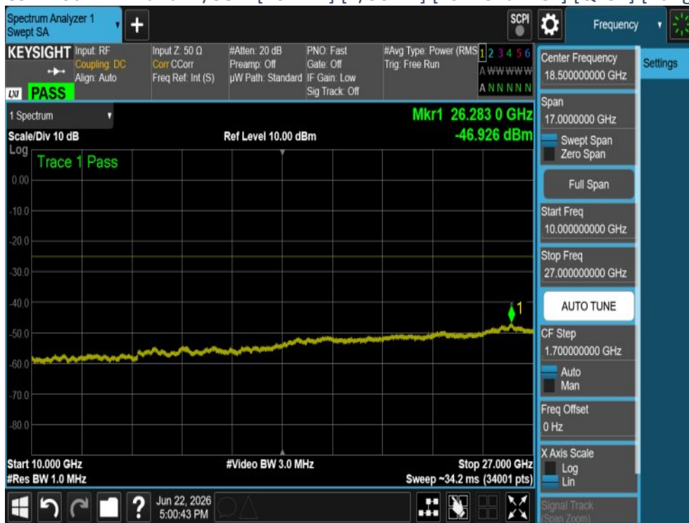
Plot 4-340 CSE Plot - LTE Band41/38[ISED] - [20MHz] [1/50 RB] [Low Channel] [QPSK] [Range A] [Ant 2]
