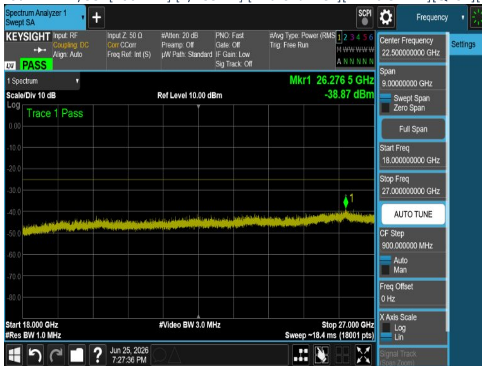
Plot 4-380 CSE Plot -NR n41/38- [100MHz] [1/135 RB] [Mid Channel ][DFT-s OFDM][QPSK][Range A][ SRS S3]
