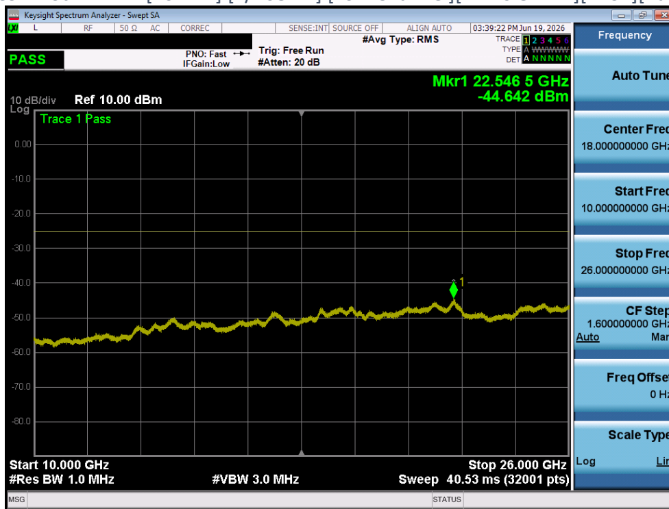
Plot 4-356 CSE Plot -NR n7- [40MHz] [1/108 RB] [Low Channel][DFT-s OFDM][BPSK][Range A][Ant 2]
