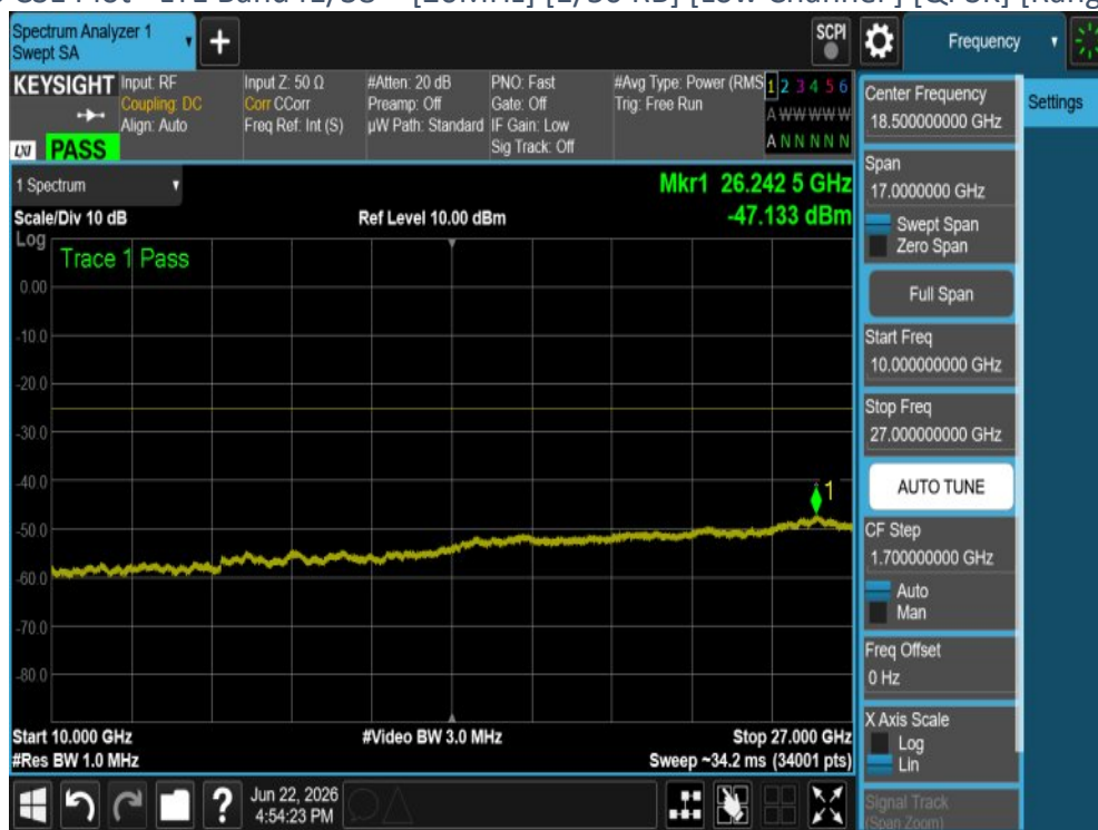
Plot 4-334 CSE Plot - LTE Band41/38[ISED] - [20MHz] [1/50 RB] [Low Channel] [QPSK] [Range A] [Ant 1]
