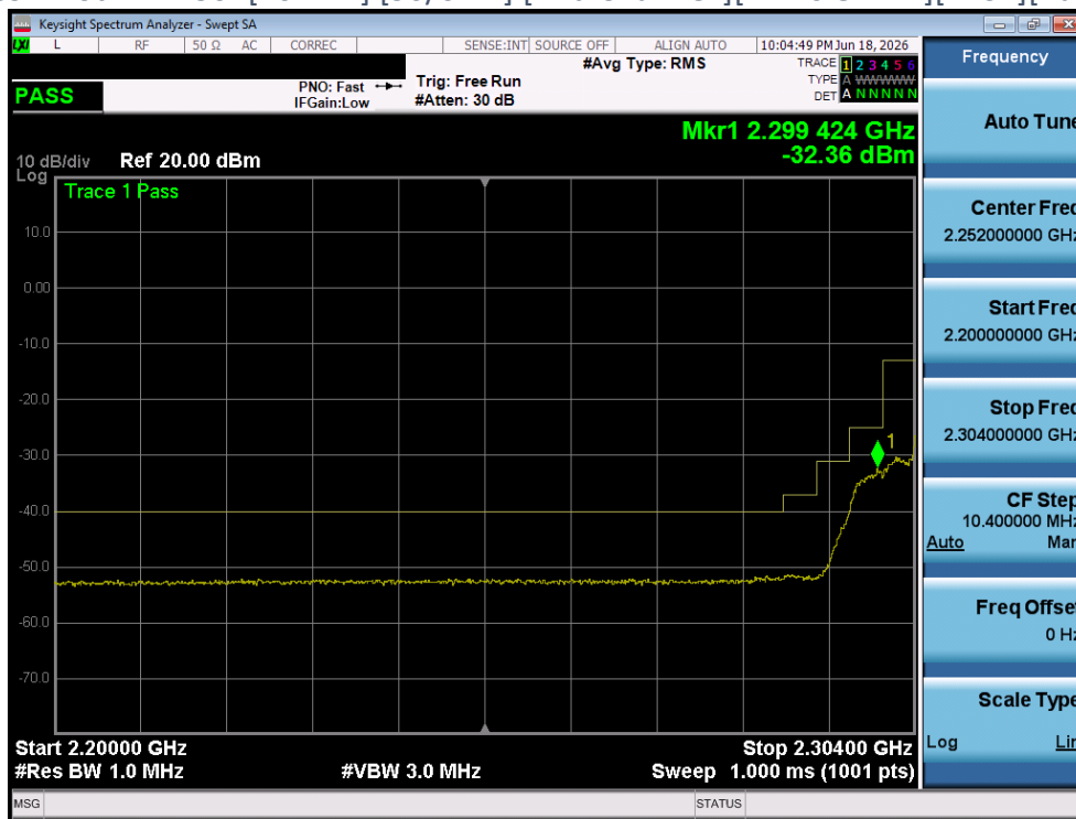
Plot 4-352 CSE Plot -NR n30- [10MHz] [50/0 RB] [Mid Channel ][DFT-s OFDM][ BPSK][Range E][Ant 2]
