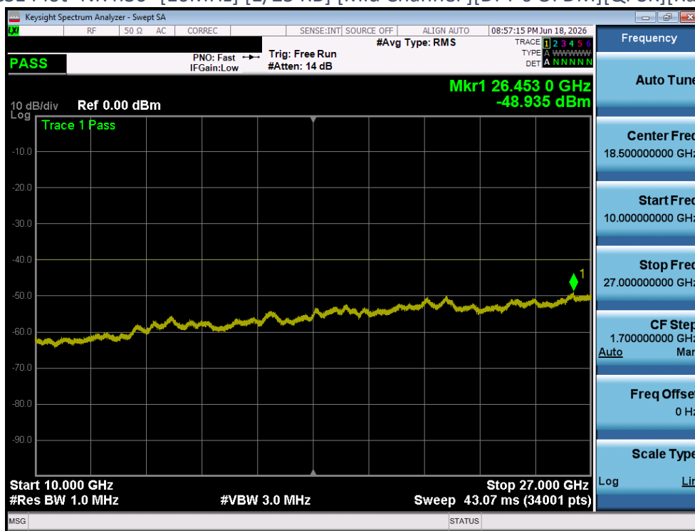
Plot 4-346 CSE Plot -NR n30- [10MHz] [50/0 RB] [Mid Channel ][DFT-s OFDM][BPSK][Range D][Ant 1]
