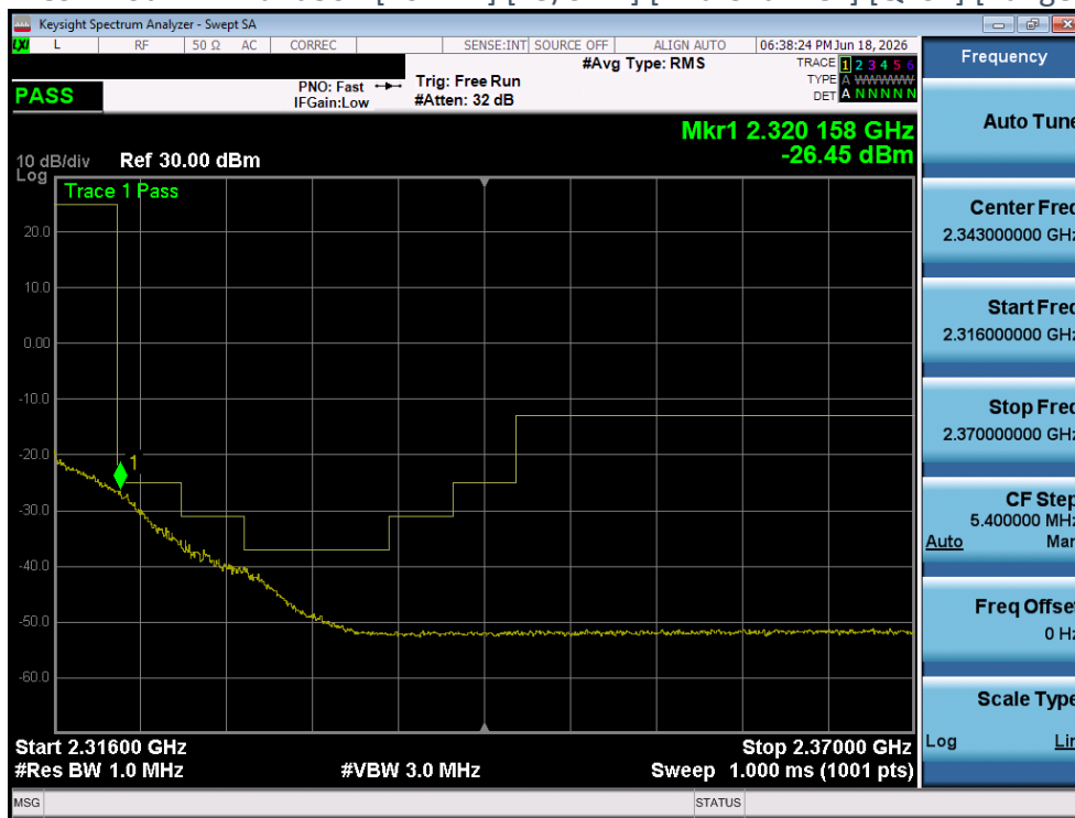
Plot 4-324 CSE Plot - LTE Band30 - [10MHz] [25/0 RB] [Mid Channel] [QPSK] [Range E] [Ant 2]
