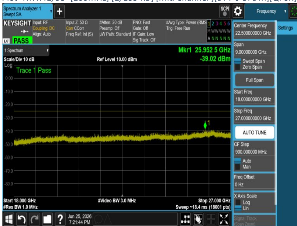
Plot 4-374 CSE Plot -NR n41/38- [100MHz] [1/135 RB] [Mid Channel ][DFT-s OFDM][QPSK][Range A][SRS S1]
