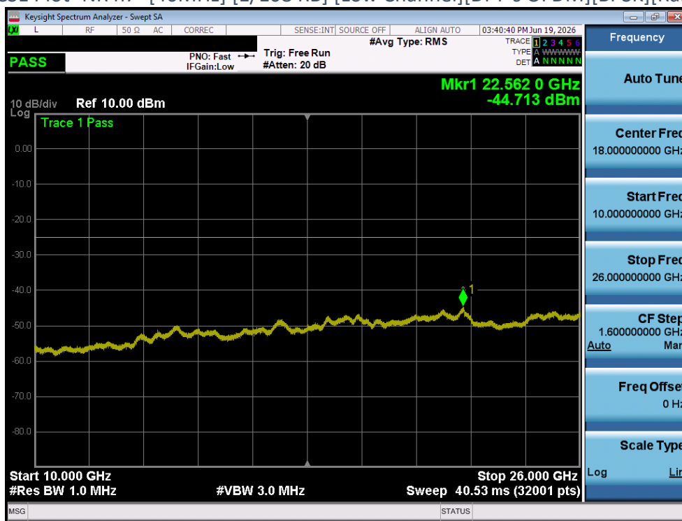
Plot 4-358 CSE Plot -NR n7- [40MHz] [1/108 RB] [Low Channel][DFT-s OFDM][BPSK][Range C][Ant 2]
