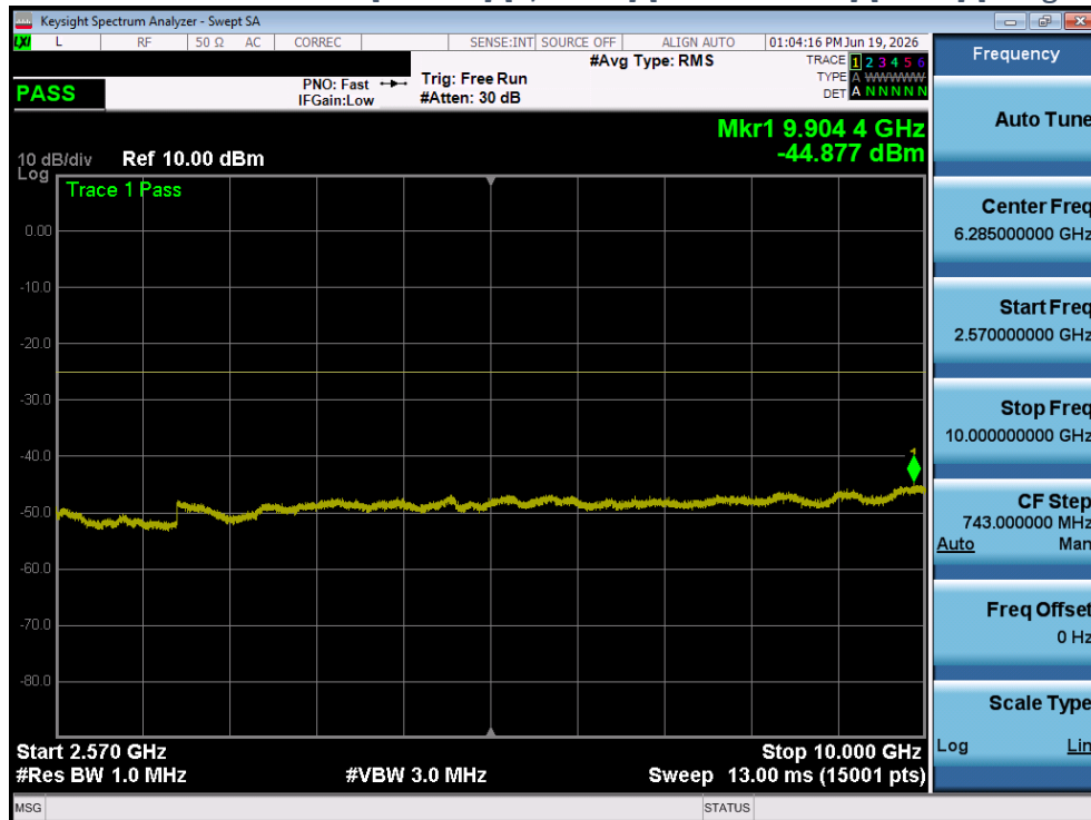
Plot 4-326 CSE Plot - LTE Band7 - [20MHz] [1/50 RB] [Mid Channel] [QPSK] [Range B] [Ant 1]
