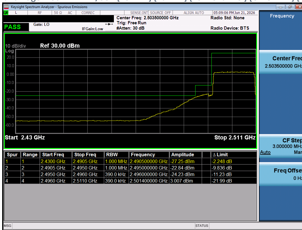
Plot 4-312 Band Edge Plot - NR n41/38 - [15MHz] [Full RB] [Low Channel] [CP-OFDM] [QPSK] [Ant 2]
