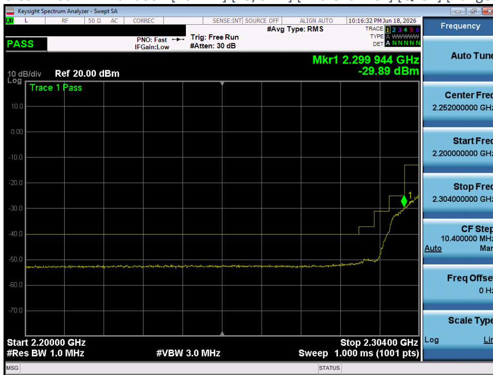
Plot 4-324 CSE Plot - LTE Band30 - [10MHz] [25/0 RB] [Mid Channel] [QPSK] [Range E] [Ant 2]
