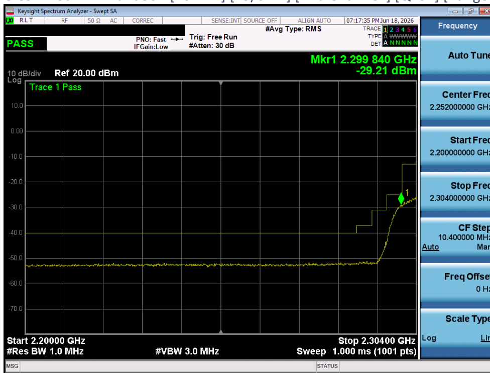
Plot 4-318 CSE Plot - LTE Band30 - [10MHz] [25/0 RB] [Mid Channel] [QPSK] [Range D] [Ant 1]
