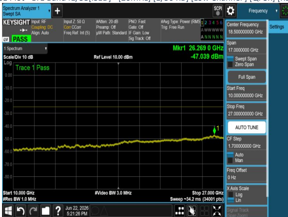
Plot 4-336 CSE Plot - LTE Band41/38[ISED] - [20MHz] [1/50 RB] [Low Channel] [QPSK] [Range C] [Ant 1]
