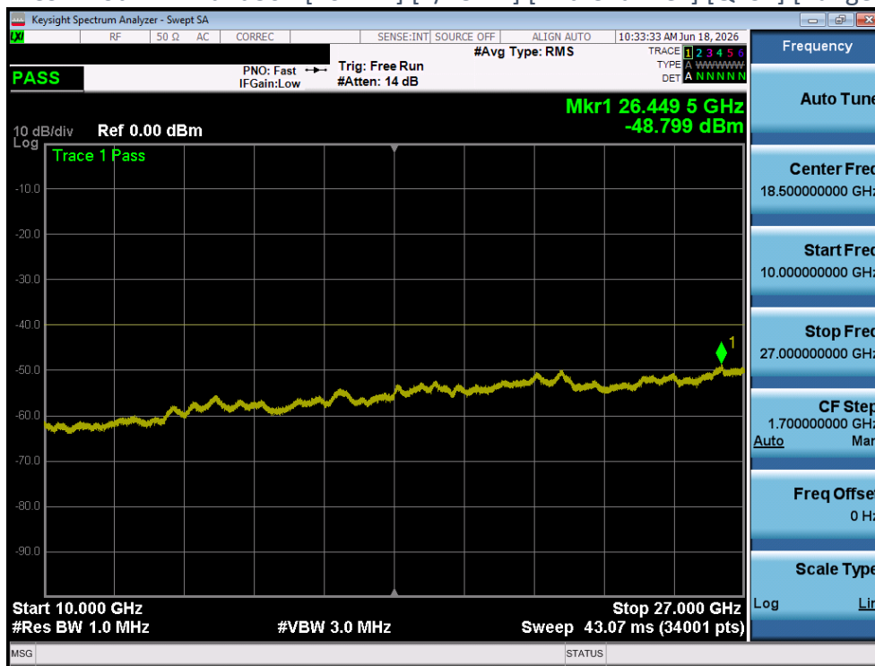
Plot 4-318 CSE Plot - LTE Band30 - [10MHz] [25/0 RB] [Mid Channel] [QPSK] [Range D] [Ant 1]
