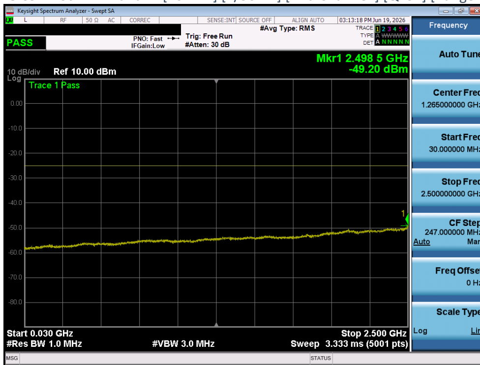
Plot 4-328 CSE Plot - LTE Band7 - [20MHz] [1/50 RB] [Mid Channel] [QPSK] [Range A] [Ant 2]
