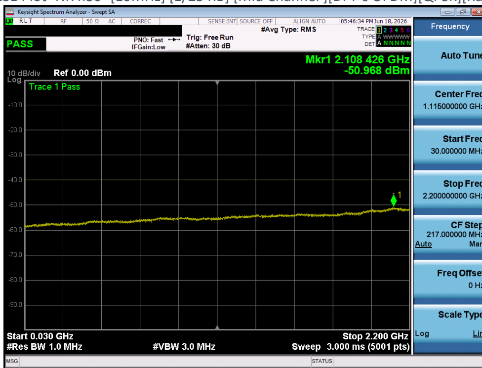
Plot 4-344 CSE Plot -NR n30- [10MHz] [1/25 RB] [Mid Channel ] [DFT-s OFDM] [QPSK] [Range B] [Ant 1]
