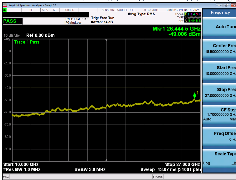
Plot 4-322 CSE Plot - LTE Band30 - [10MHz] [1/25 RB] [Mid Channel] [QPSK] [Range C] [Ant 2]
