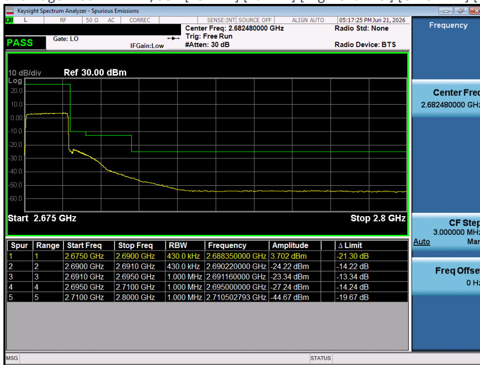
Plot 4-314 Band Edge Plot - NR n41/38 - [15MHz] [Full RB] [High Channel] [CP-OFDM] [QPSK] [Ant 2]
