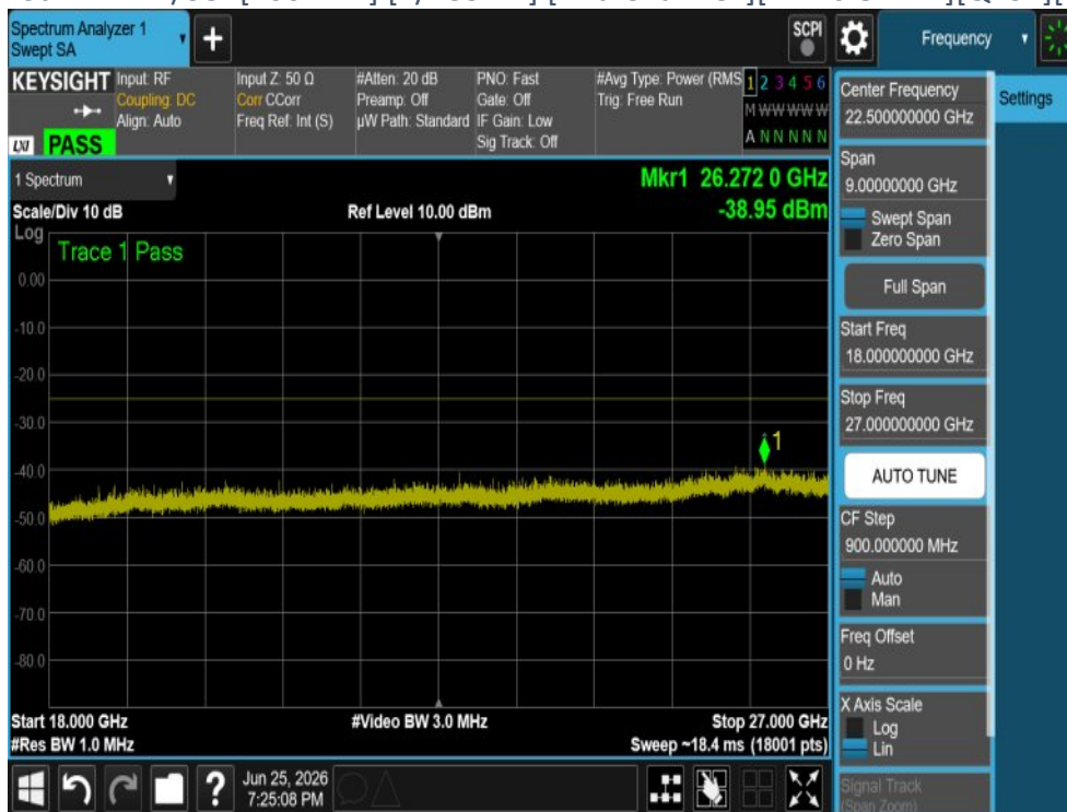
Plot 4-376 CSE Plot -NR n41/38- [100MHz] [1/135 RB] [Mid Channel ][DFT-s OFDM][QPSK][Range C][ SRS S1]
