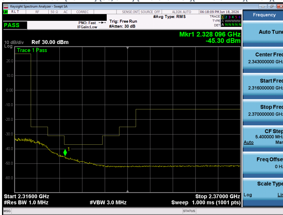
Plot 4-348 CSE Plot -NR n30- [10MHz] [1/25 RB] [Mid Channel ][DFT-s OFDM][QPSK][Range A][Ant 2]
