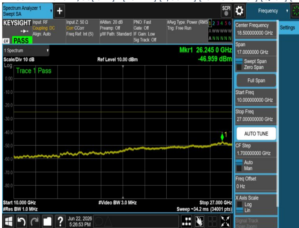
Plot 4-342 CSE Plot - LTE Band41/38[ISED] - [20MHz] [1/50 RB] [Low Channel] [QPSK] [Range C] [Ant 2]
