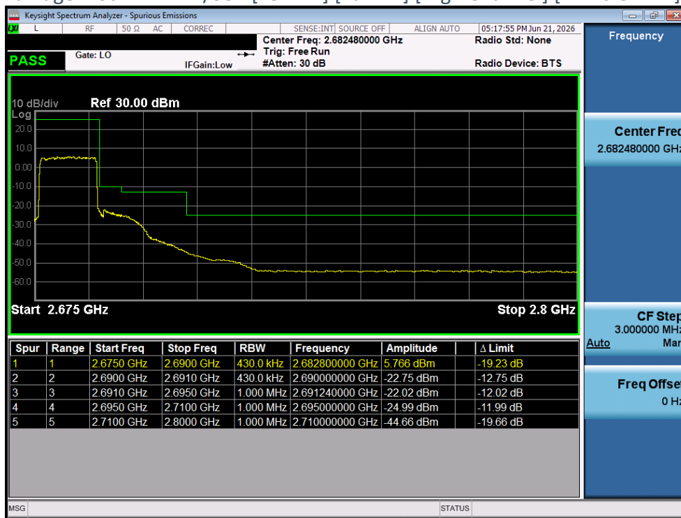
Plot 4-314 Band Edge Plot - NR n41/38 - [15MHz] [Full RB] [High Channel] [CP-OFDM] [QPSK] [Ant 2]
