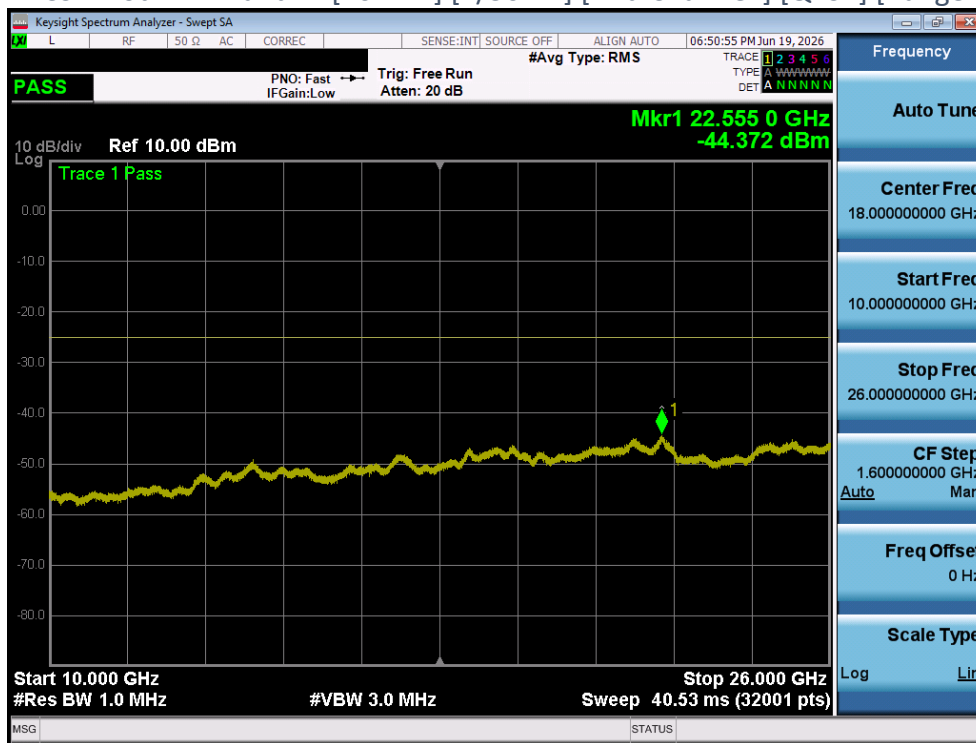
Plot 4-328 CSE Plot - LTE Band7 - [20MHz] [1/50 RB] [Mid Channel] [QPSK] [Range A] [Ant 2]
