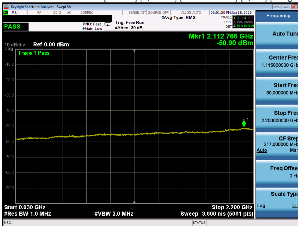
Plot 4-320 CSE Plot - LTE Band30 - [10MHz] [1/25 RB] [Mid Channel] [QPSK] [Range A] [Ant 2]
