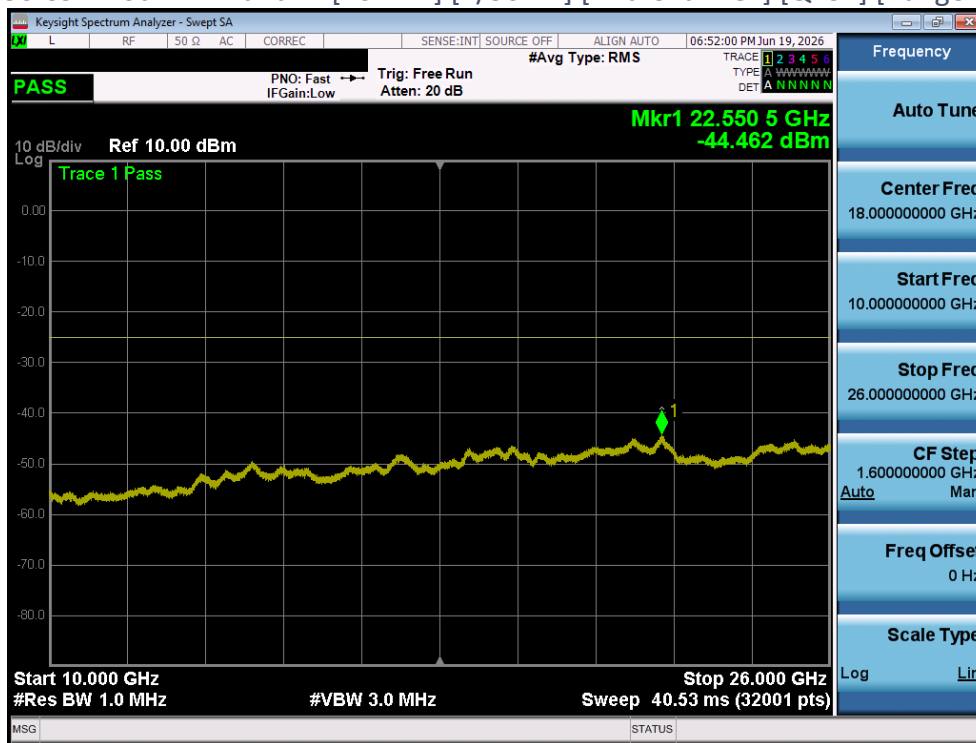
Plot 4-330 CSE Plot - LTE Band7 - [20MHz] [1/50 RB] [Mid Channel] [QPSK] [Range C] [Ant 2]
