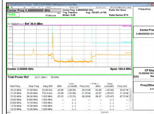
5G NR n77 60MHz BPSK Low Channel RB1-0
