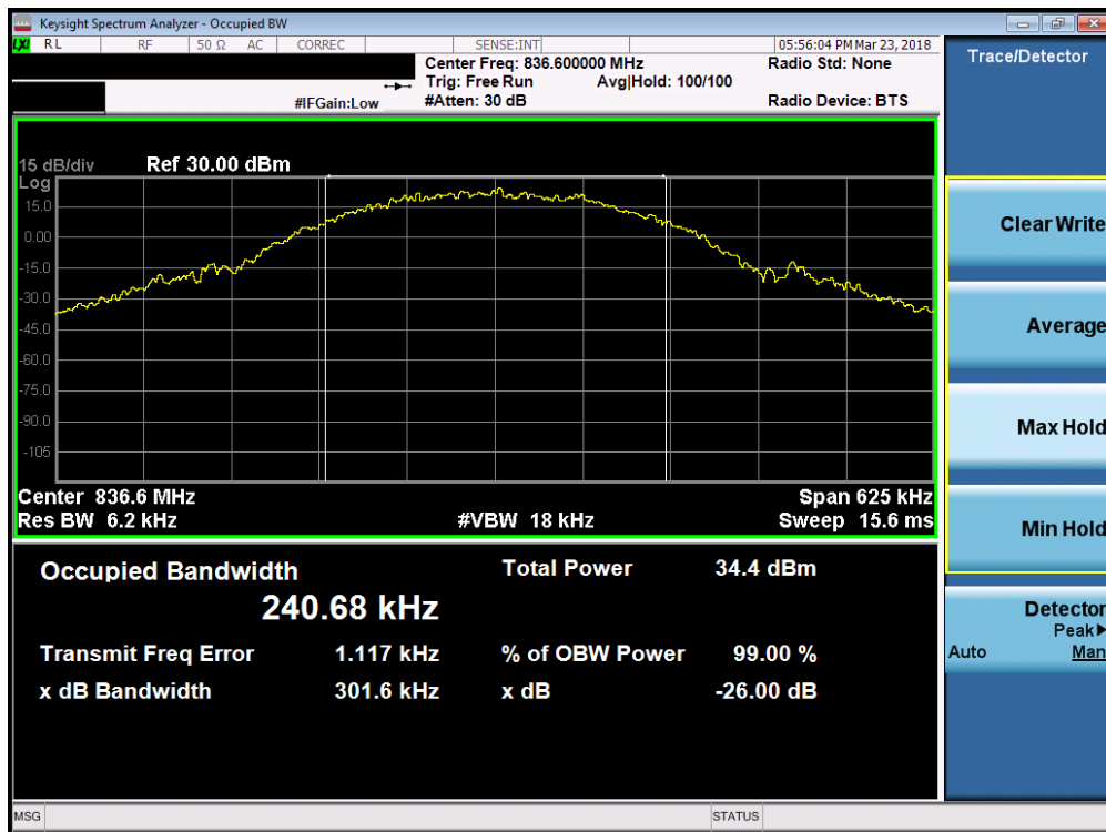
Plot 7-2. Occupied Bandwidth Plot (EDGE850 Mode)
