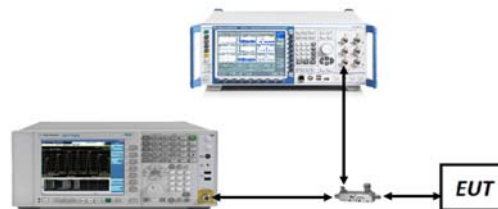
Figure 7-3. Test Instrument & Measurement Setup
