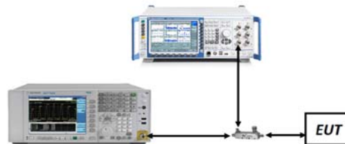
Figure 7-2. Test Instrument & Measurement Setup
