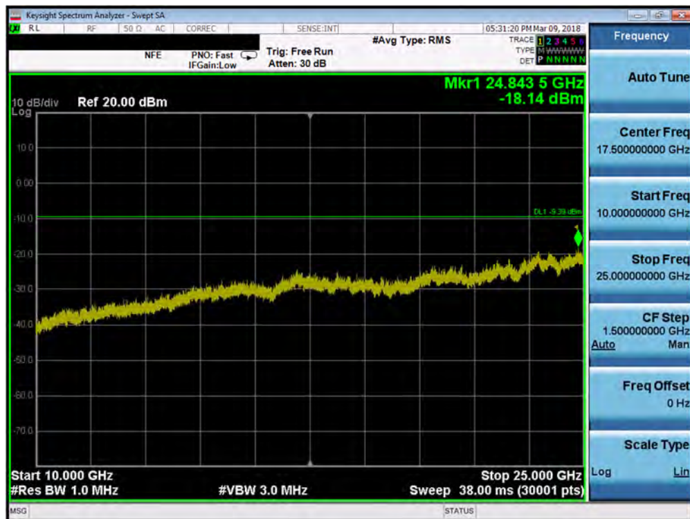
Plot 7-41. Conducted Spurious Plot (Bluetooth, 1Mbps – Ch. 78)
