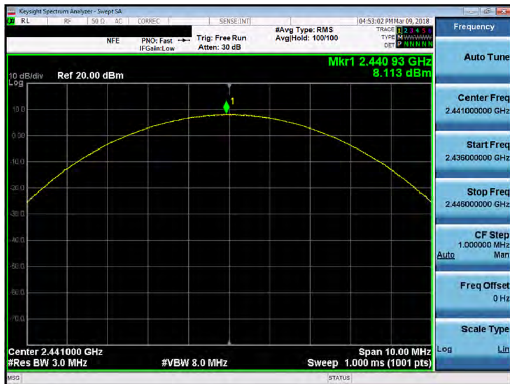
Plot 7-17. Peak Conducted Power (3Mbps – Ch. 39)
