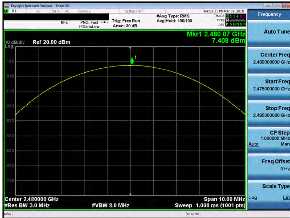
Plot 7-18. Peak Conducted Power (3Mbps – Ch. 78)
