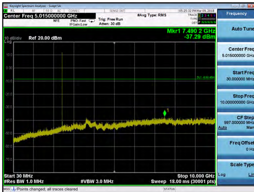
Plot 7-38. Conducted Spurious Plot (Bluetooth, 1Mbps – Ch. 39)
