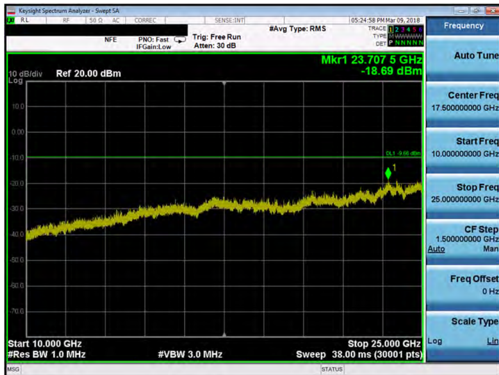
Plot 7-37. Conducted Spurious Plot (Bluetooth, 1Mbps – Ch. 0)
