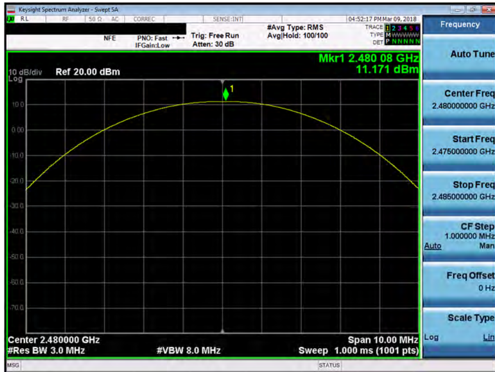
Plot 7-12. Peak Conducted Power (1Mbps – Ch. 78)
