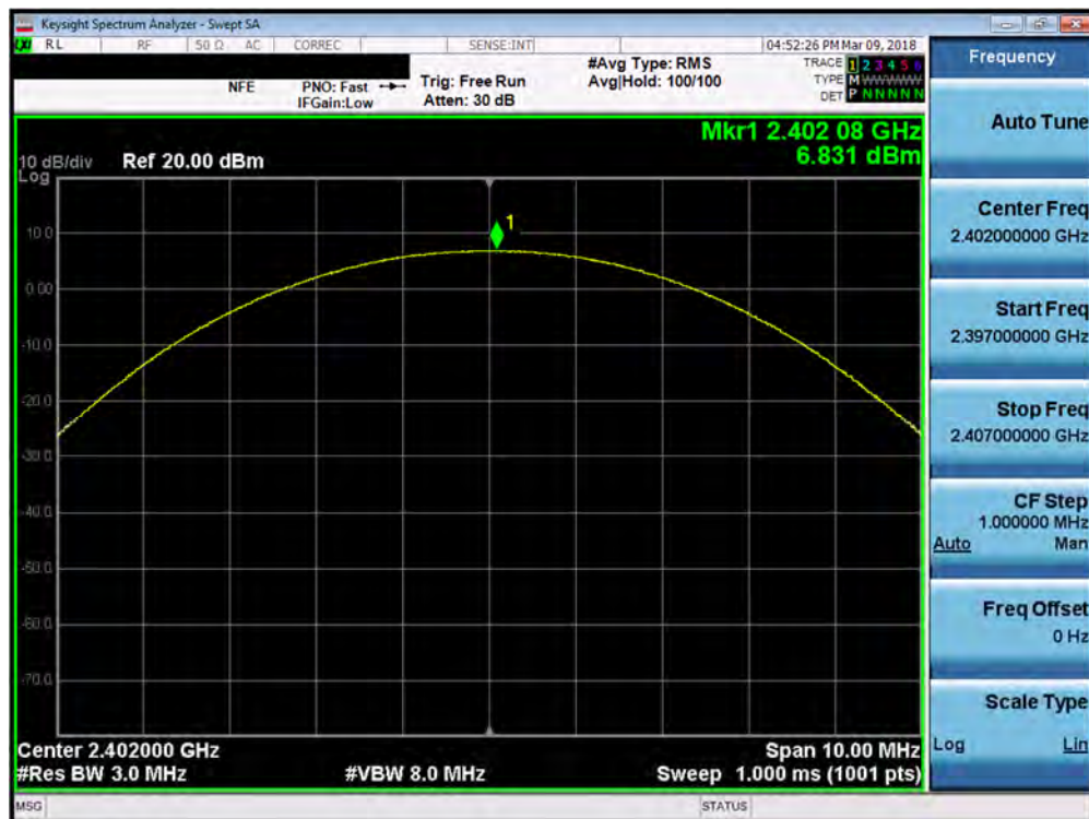
Plot 7-13. Peak Conducted Power (2Mbps – Ch. 0)
