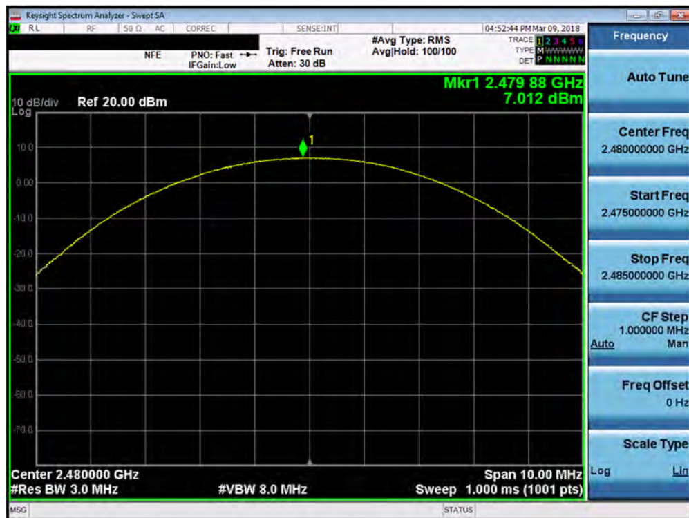
Plot 7-15. Peak Conducted Power (2Mbps – Ch. 78)
