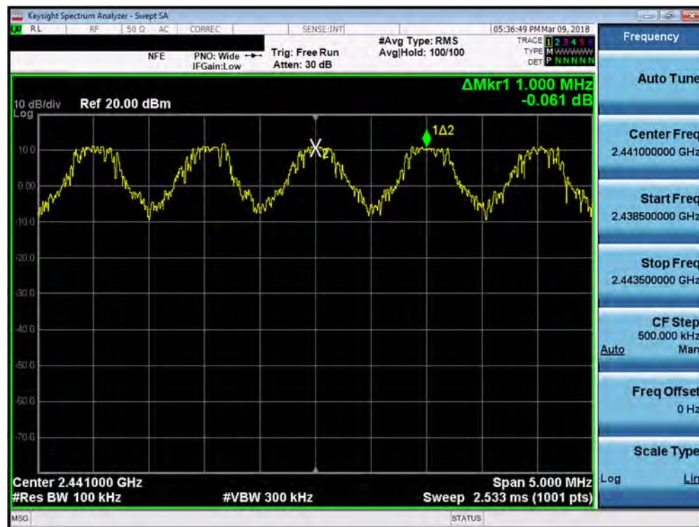
Plot 7-32. Channel Spacing Plot (Bluetooth)
