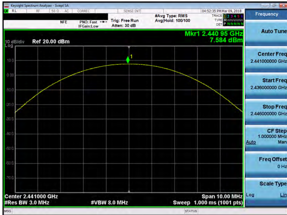
Plot 7-14. Peak Conducted Power (2Mbps – Ch. 39)
