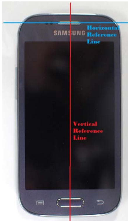
SAR Test Setup Photo 6 – DUT Horizontal and Vertical Reference Lines
