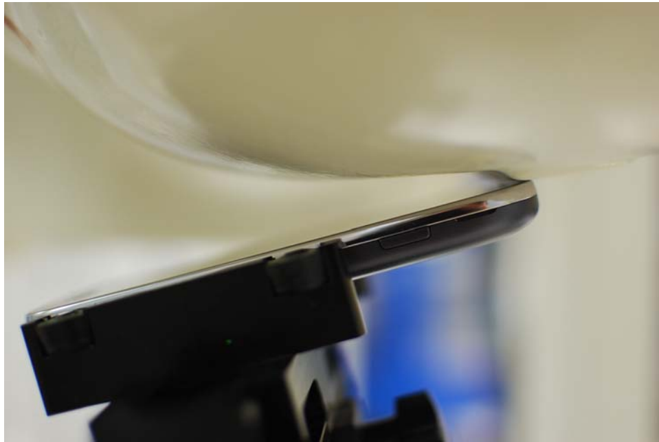
SAR Test Setup Photo 4 – Left Tilt
