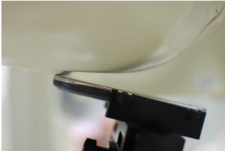
SAR Test Setup Photo 2 – Right Tilt
