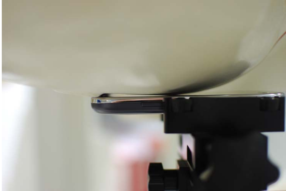
SAR Test Setup Photo 1 – Right Cheek
