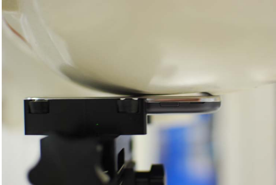
SAR Test Setup Photo 3 – Left Cheek
