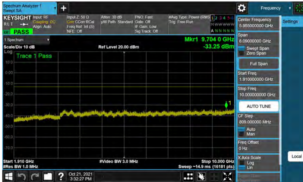
Plot 7-26. Conducted Spurious Plot (GPRS Ch. 512)
