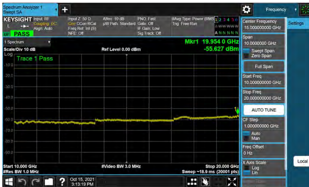
Plot 7-24. Conducted Spurious Plot (LTE Band 25/2 - 20MHz QPSK - 1RB - High Channel)
