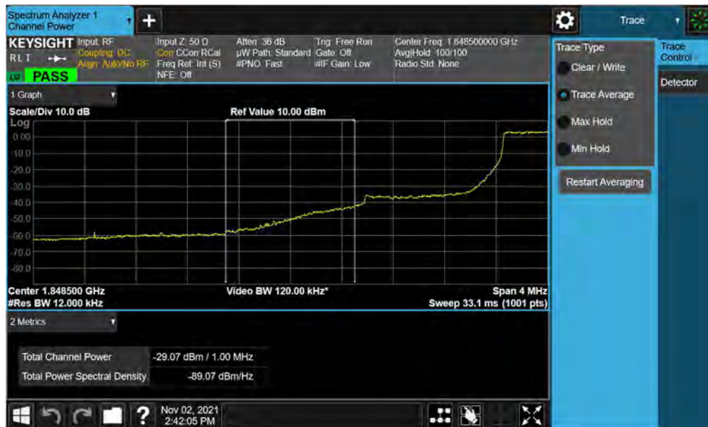
Plot 7-74. Extended Lower Band Edge Plot (LTE Band 25/2 – 1.4MHz QPSK – Full RB)
