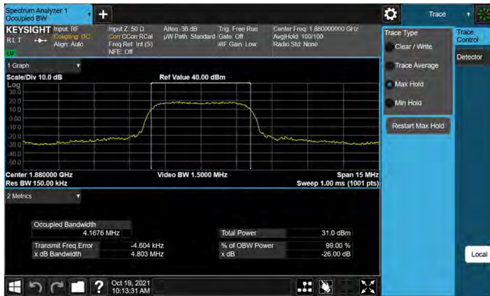
Plot 7-15. Occupied Bandwidth Plot (WCDMA, Ch. 9400)
