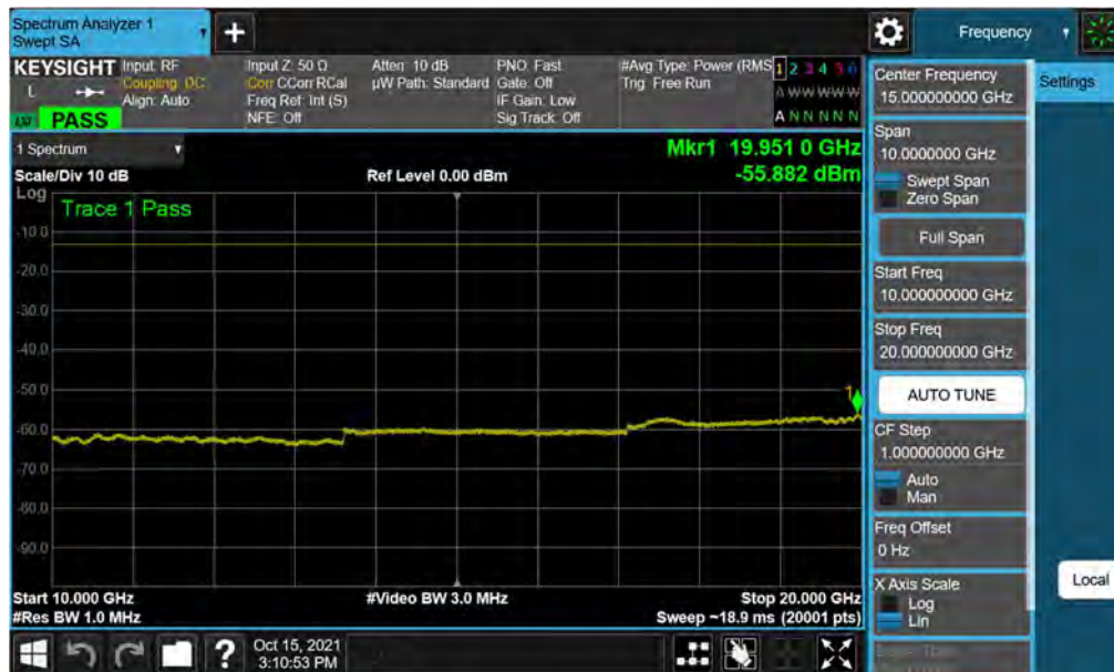
Plot 7-21. Conducted Spurious Plot (LTE Band 25/2 - 20MHz QPSK - 1RB - Mid Channel)
