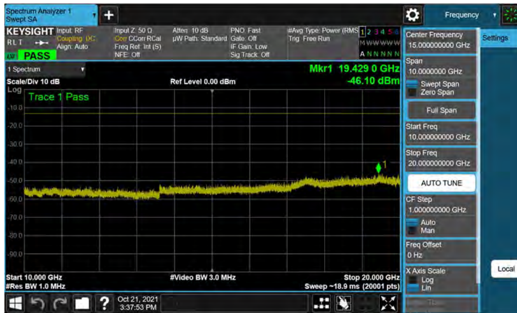
Plot 7-33. Conducted Spurious Plot (GPRS Ch. 810)
