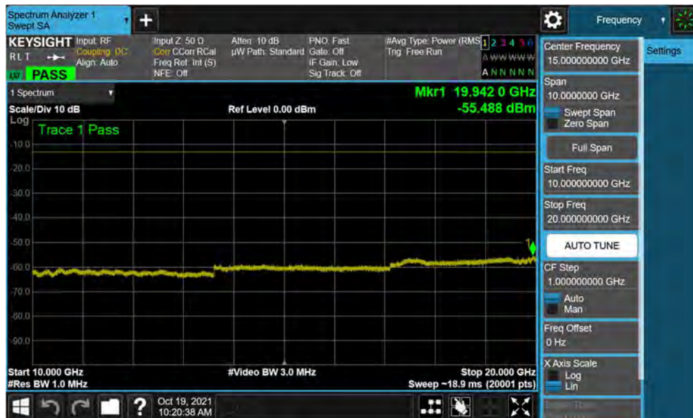
Plot 7-39. Conducted Spurious Plot (WCDMA Ch. 9400)
