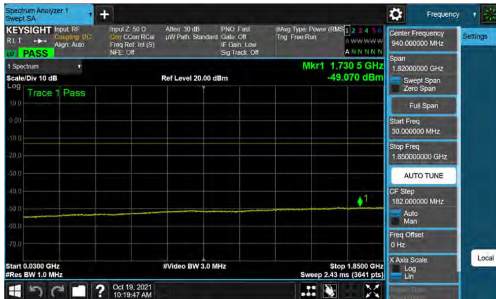
Plot 7-37. Conducted Spurious Plot (WCDMA Ch. 9400)
