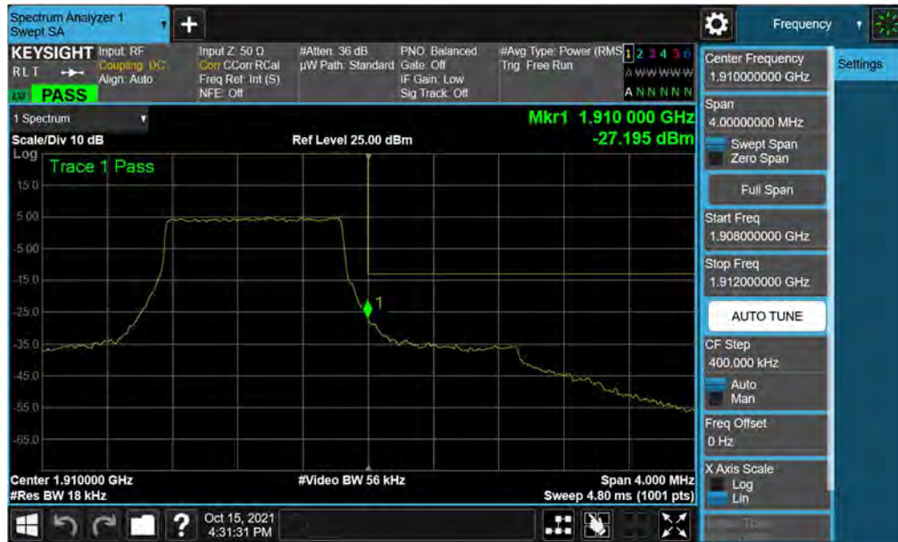
Plot 7-75. Upper Band Edge Plot (LTE Band 2 – 1.4MHz QPSK – Full RB)
