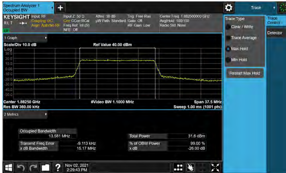
Plot 7-3. Occupied Bandwidth Plot (LTE Band 25/2 - 15MHz QPSK - Full RB)
