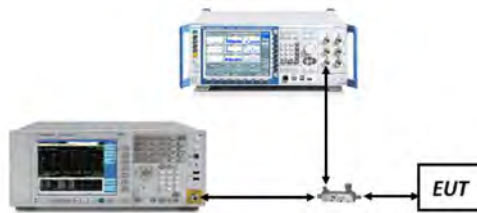
Figure 7-1. Test Instrument & Measurement Setup
