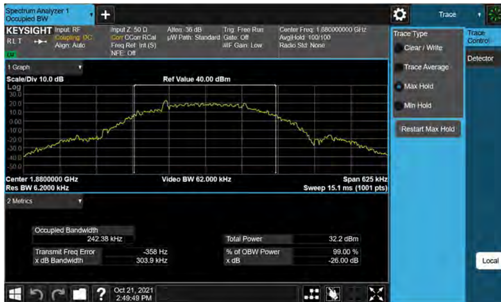
Plot 7-14. Occupied Bandwidth Plot (EDGE, Ch. 661)
