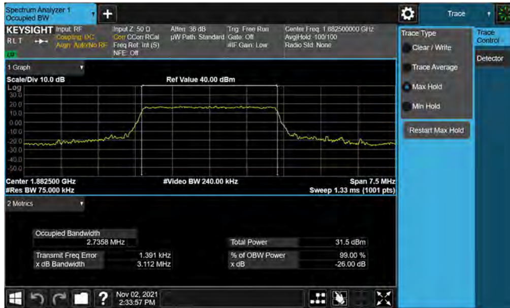
Plot 7-9. Occupied Bandwidth Plot (LTE Band 25/2 - 3MHz QPSK - Full RB)
