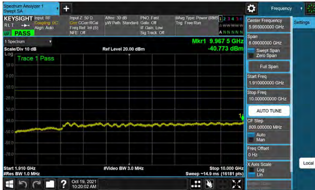
Plot 7-38. Conducted Spurious Plot (WCDMA Ch. 9400)
