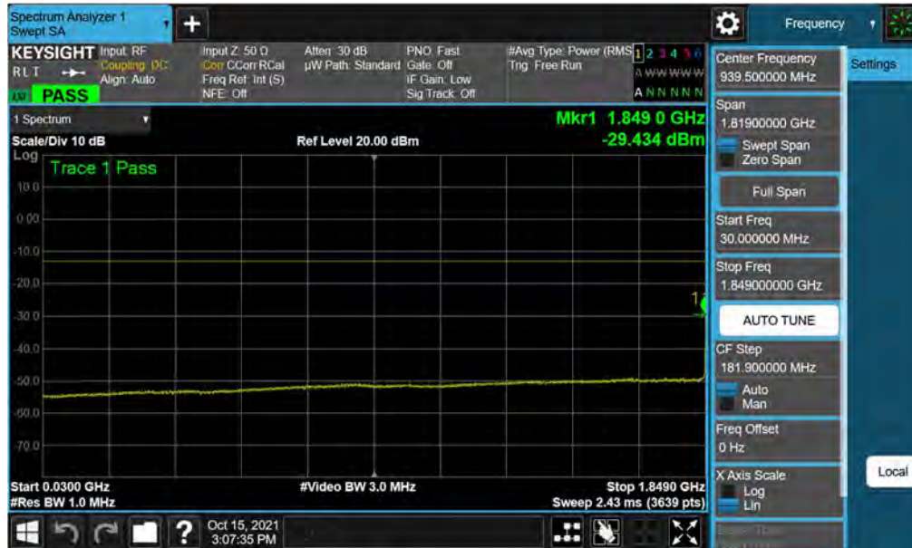
Plot 7-16. Conducted Spurious Plot (LTE Band 25/2 - 20MHz QPSK - 1RB - Low Channel)
