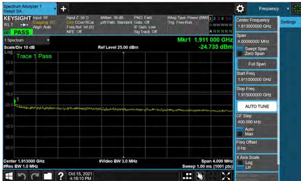
Plot 7-58. Extended Upper Band Edge Plot (LTE Band 2 - 10MHz QPSK – Full RB)
