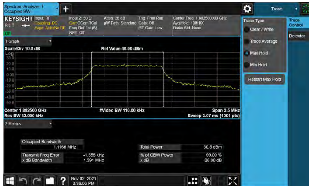
Plot 7-12. Occupied Bandwidth Plot (LTE Band 25/2 - 1.4MHz 16-QAM - Full RB)
