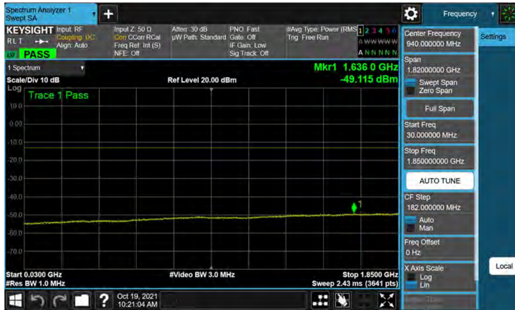
Plot 7-40. Conducted Spurious Plot (WCDMA Ch. 9538)
