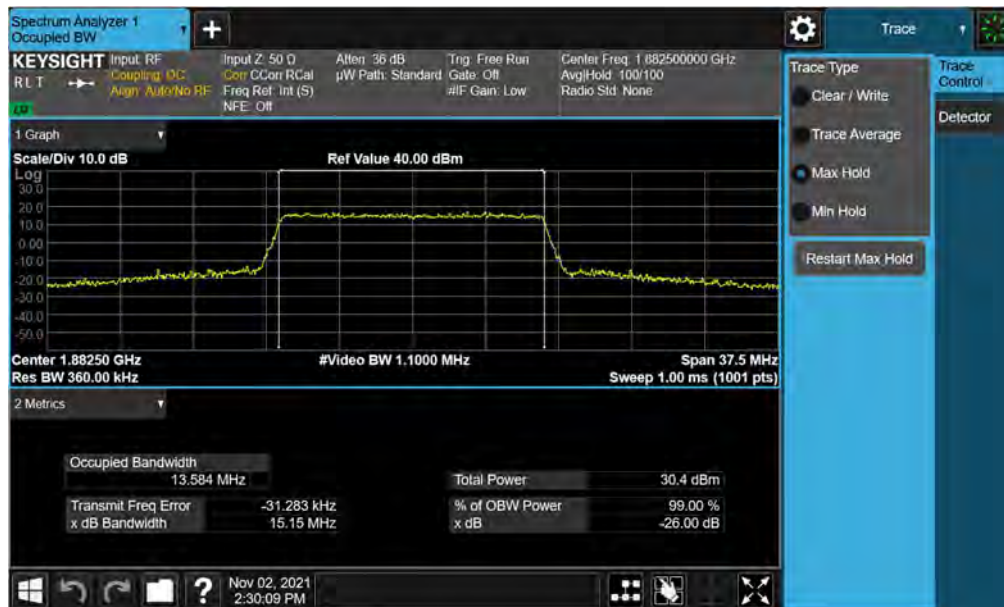
Plot 7-4. Occupied Bandwidth Plot (LTE Band 25/2 - 15MHz 16-QAM - Full RB)
