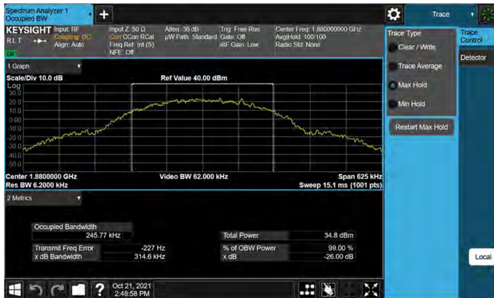
Plot 7-13. Occupied Bandwidth Plot (GPRS, Ch. 661)
