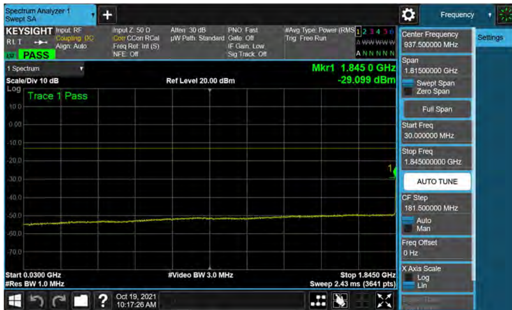
Plot 7-34. Conducted Spurious Plot (WCDMA Ch. 9262)
