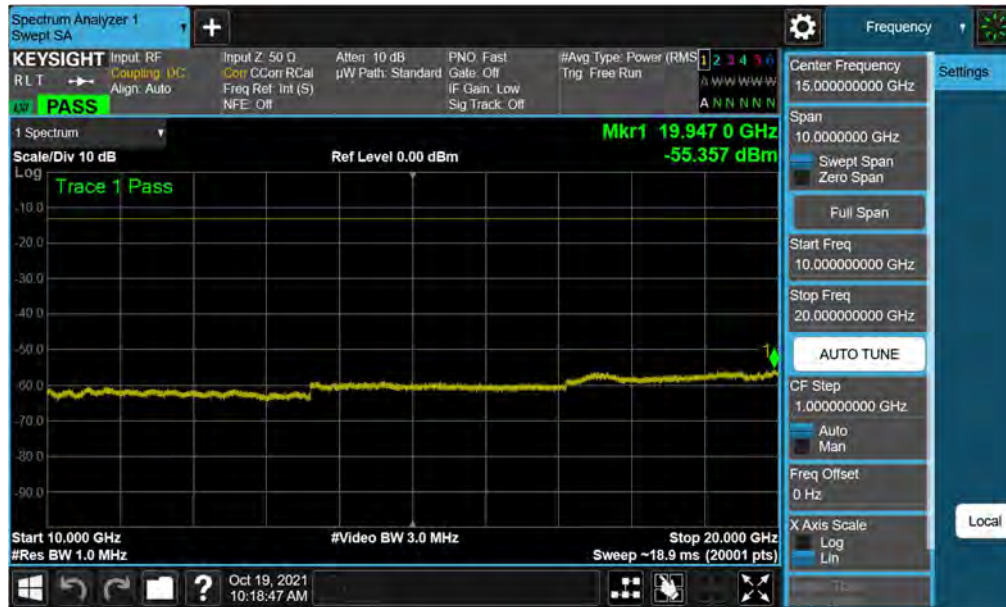
Plot 7-36. Conducted Spurious Plot (WCDMA Ch. 9262)
