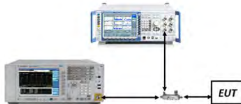
Figure 7-3. Test Instrument & Measurement Setup
